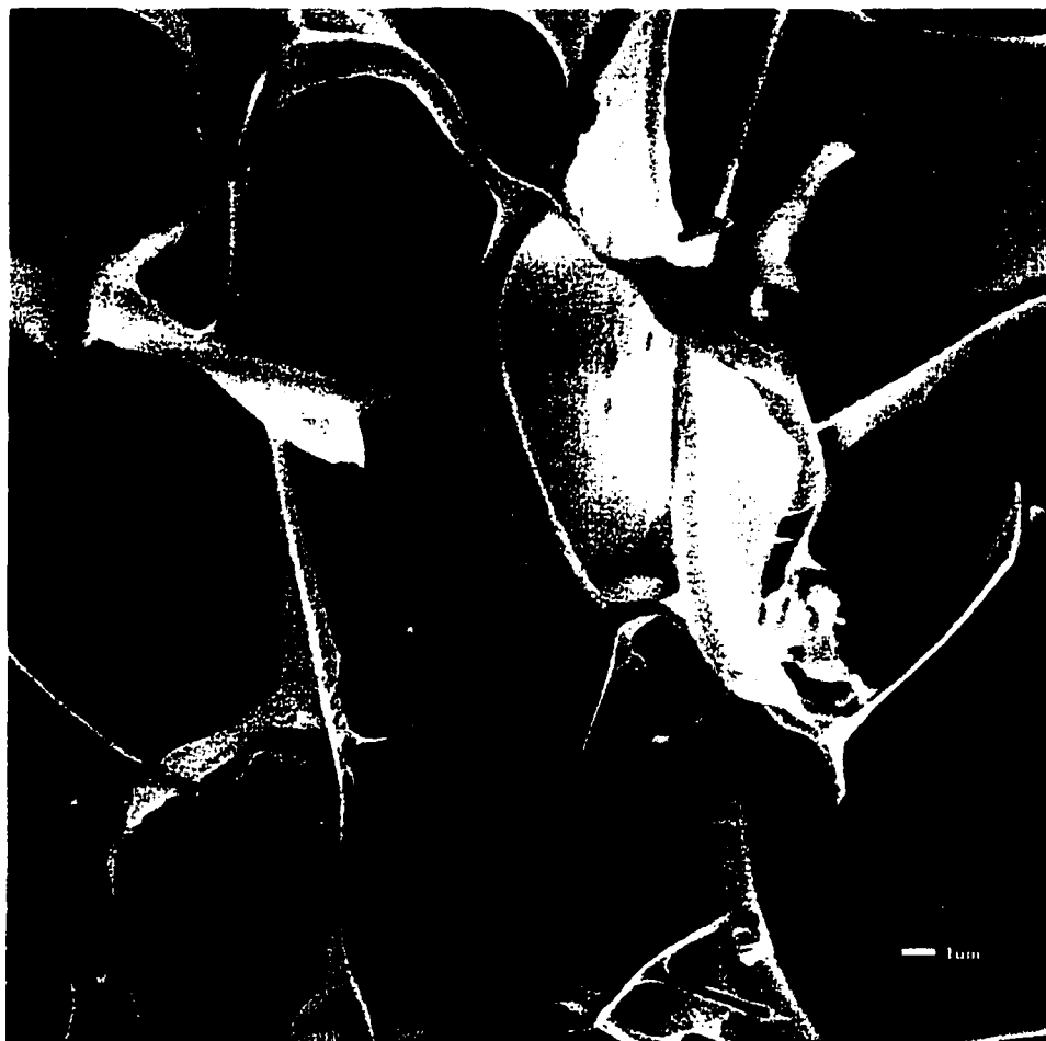
Figure 5.76 High Magnification Electron Microscope Image of the Concentrated Material Representative of the Above 5000 MW Fraction (Top Sample Portion)
