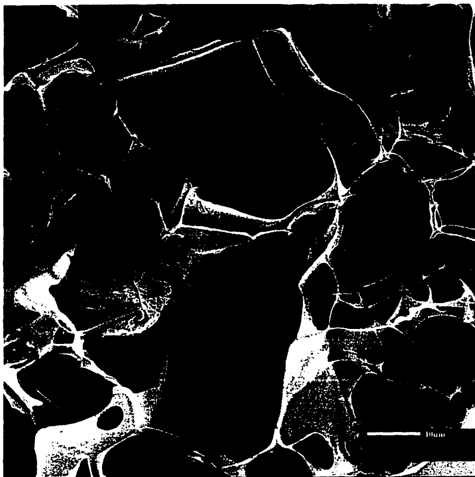
Figure 5.75 Electron Microscope Photograph of the Concentrated Material Structure Observed for the Above 5000 MW Fraction for Membrane Concentrate Frozen at the Initial Freezing Temperature -15 degrees Celsius (Top Sample Portion)
