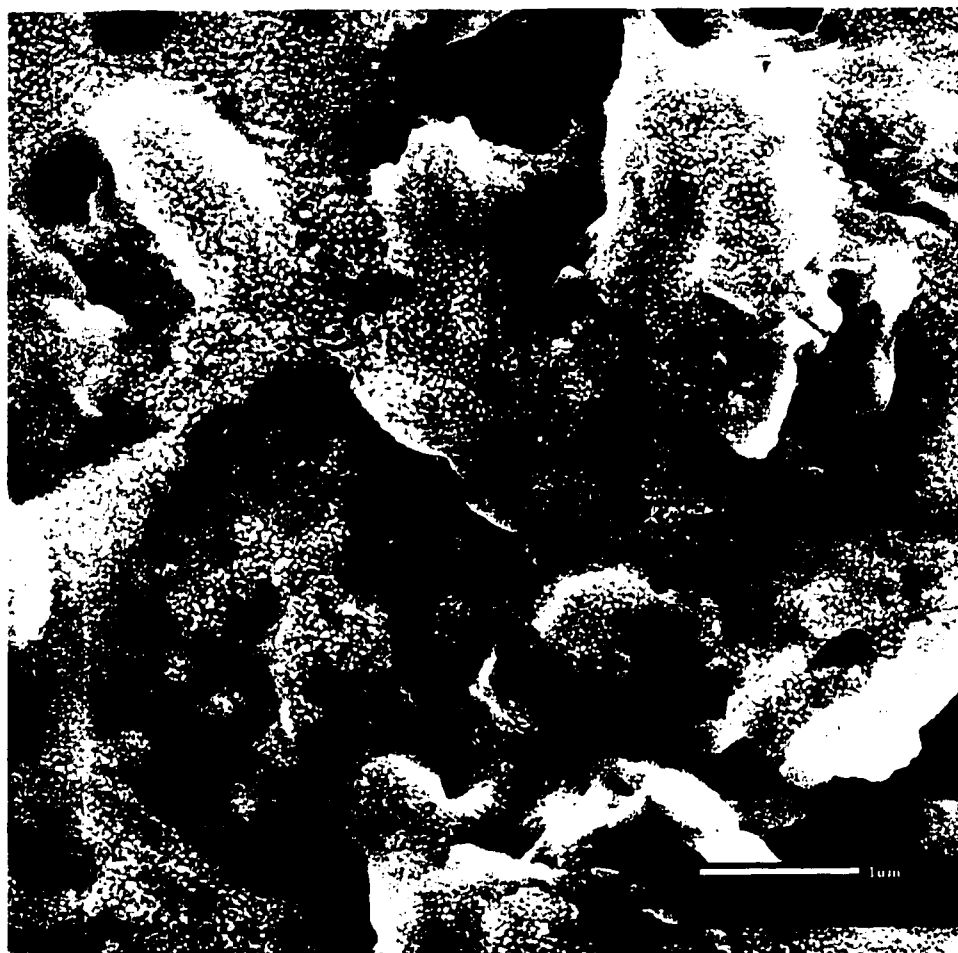
Figure 5.50 High Magnification Electron Microscope Image Showing the Morphology of the Concentrated Material Retained on the Filter Paper After Thawing Membrane Concentrate Frozen at the Initial Freezing Temperature -2 degrees Celsius (Extreme Close-up)
