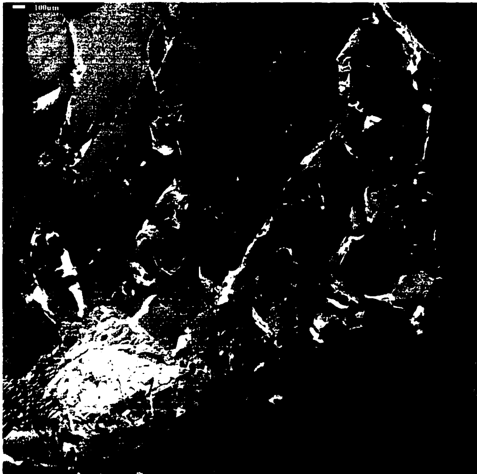
Figure 5.73 Electron Microscope Photograph of a Fractured Ice Specimen Surface Produced by Freezing Membrane Concentrate Diluted to 75 % at the Initial Freezing Temperature -15 degrees Celsius
