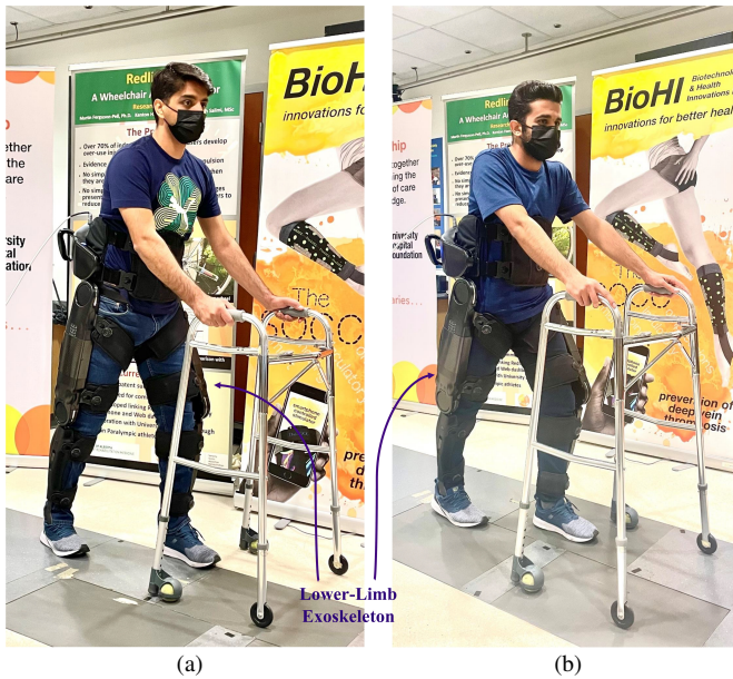
Fig. 3. Indego lower-limb exoskeleton worn by two able-bodied users for overground walking: (a) first participant (33 year-old) and (b) second participant (27 year-old)
