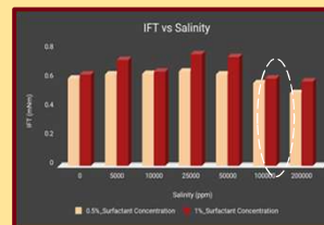
Figure 12: Effect of Surfactant concentration on IFT
