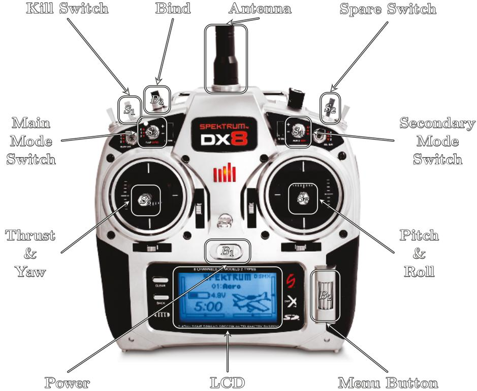
Figure 3.2: The Spektrum DX8 remote transmitter
