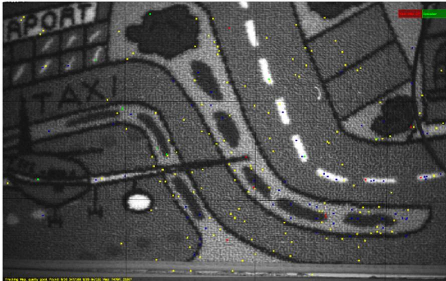
Figure 5.8: A screen shot of the camera view during the experiment. The coloured points are 3 D points from the map that are being tracked in the image.
