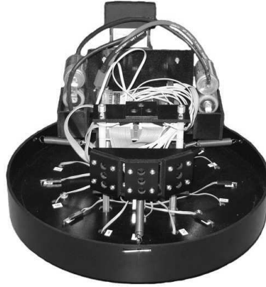
Figure 4.13: This figure shows one of the robots used in the physical experiments. Each robot possessed a circular bump sensor that permitted it to detect obstacles. At the rear and top of the robot is an 802.11B radio, which it used to communicate with its teammates when making a group decision.
