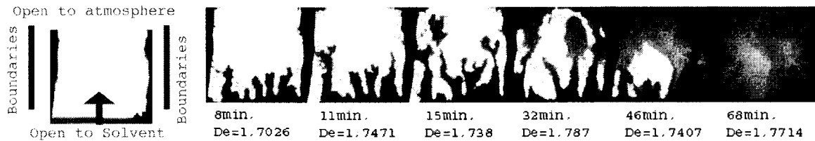
Figure 9.5: Pentane (red) kerosene (white) experiment (co-current, vertical orientation). Thick (blue) lines in the model representation indicate the sides closed to flow.
