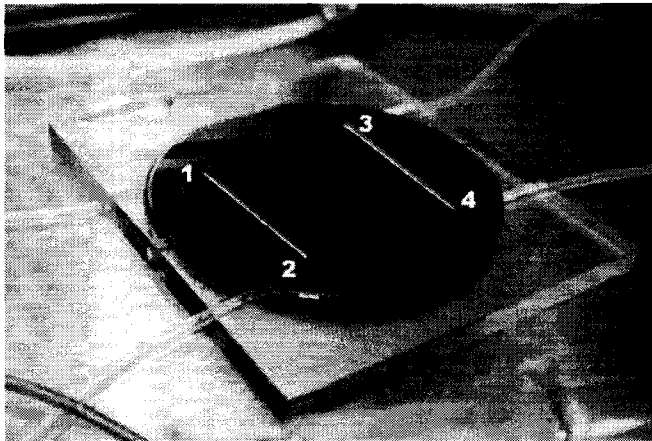
Figure 3.6 a) Glass model on holder, inlet-outlet ports connected, vacuum port disconnected. Ports on the model are marked with numbers. Ports 1&2 and 3&4 are connected with fracture which is highlighted with gray lines, b) model holder with four configurable ports and one vacuum port. Vacuum suction cups are connected to vacuum port internally.
