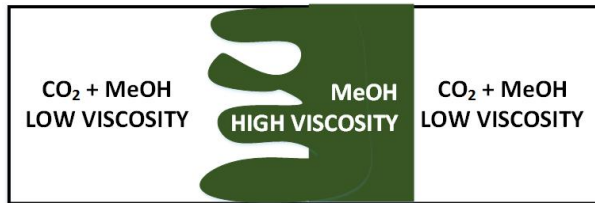
Figure 5.3: Displacement of two miscible fluids with different viscosities in porous media when rear interface is affected by viscous fingering. MeOH (methanol) is the high viscosity plug and \text{CO}_2 + \text{MeOH} represents the low viscosity mobile phase.
