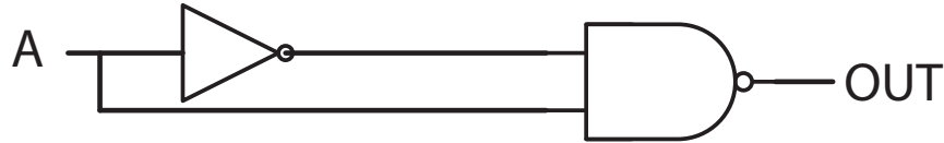
Figure 4.7: NAND gate with statistically dependent input signals.
