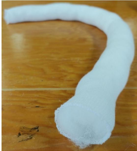
Figure 2.6: Photo of regenerator matrix, made of tubular gauze and polyester fiber material.
