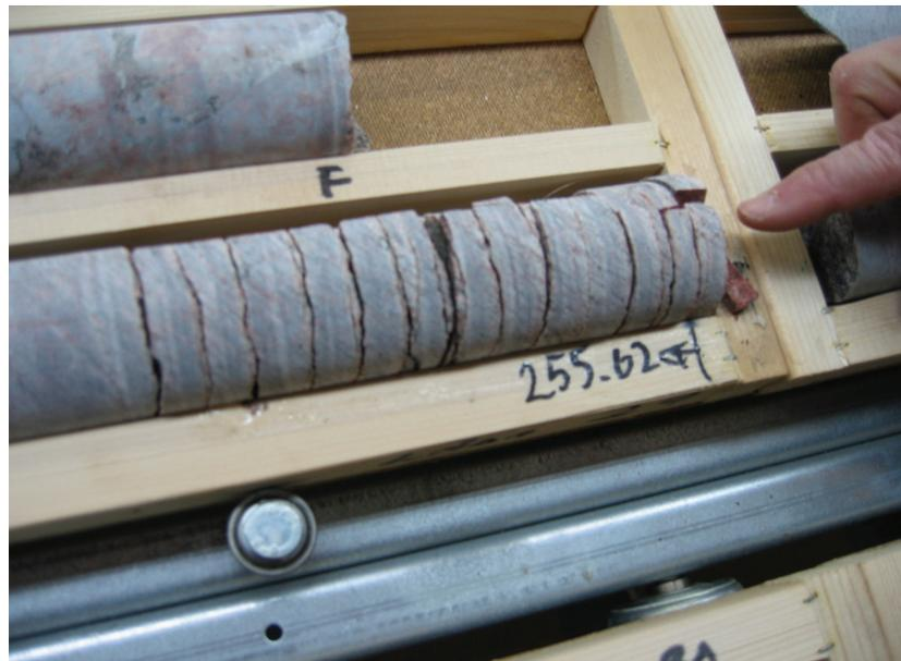
Figure B.2: Core dinking in overcored sample at a depth of 255 m in Forsmark site investigation borehole.
