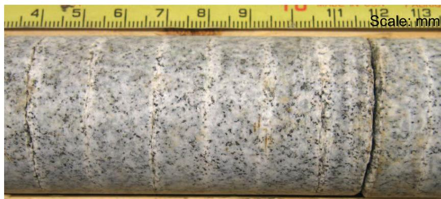
Figure 4.7: The partial core diking fractures.
