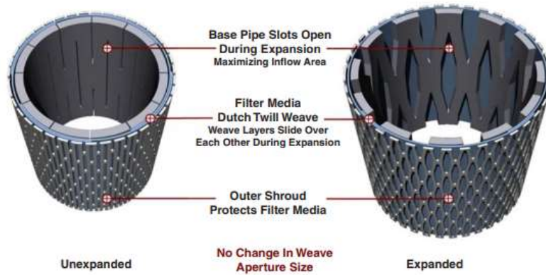
Figure 2-6. Expandable-Sand-Screen (ESS) (Ismail and Geddes, 2014).
