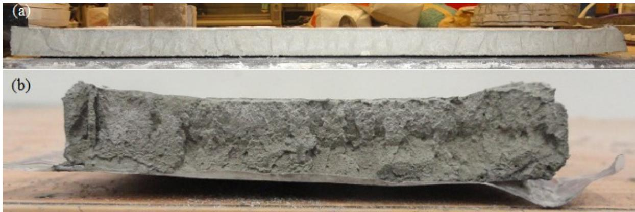
Figure 5.7 Curling observed in the slab-like specimen: (a) side view, and (b) end view.
