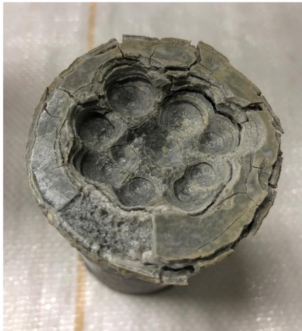
Figure 2.2 Loss of cohesion, delamination and fragmentation observed at the top-end cylinder with the sides coated with epoxy resin after being submitted to  $Na_2SO_4$  solution for one year.
