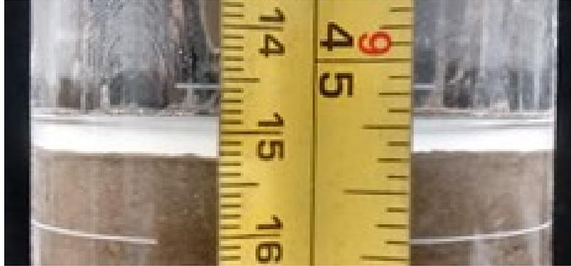
Figure 5.17 View of the clear-light turbid bleed water in the control paste after 4-hour trail.
