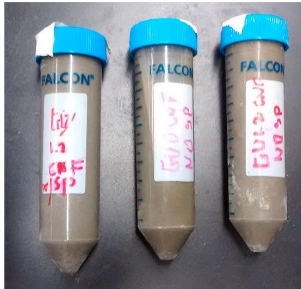
Figure 4.1 View of the sealed vials containing the 1-year paste samples.
