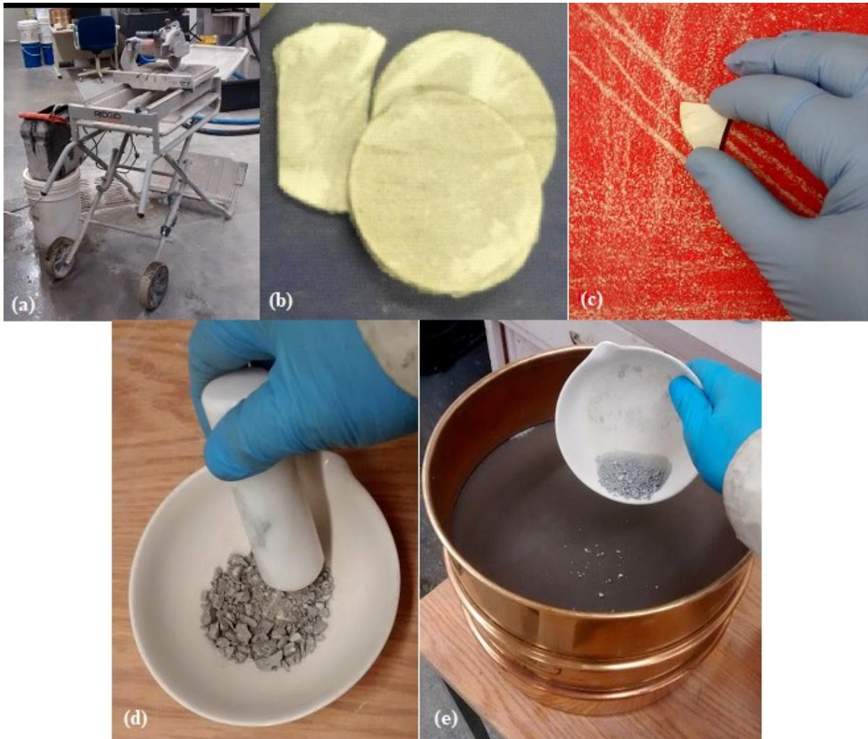
Figure 6.19 Sequence showing the sample preparation: (a) bench saw cutting machine used to slice the cylinder; (b) cut slices; (c) sandpapering; (d) grinding; and (e) sieving the sample.
