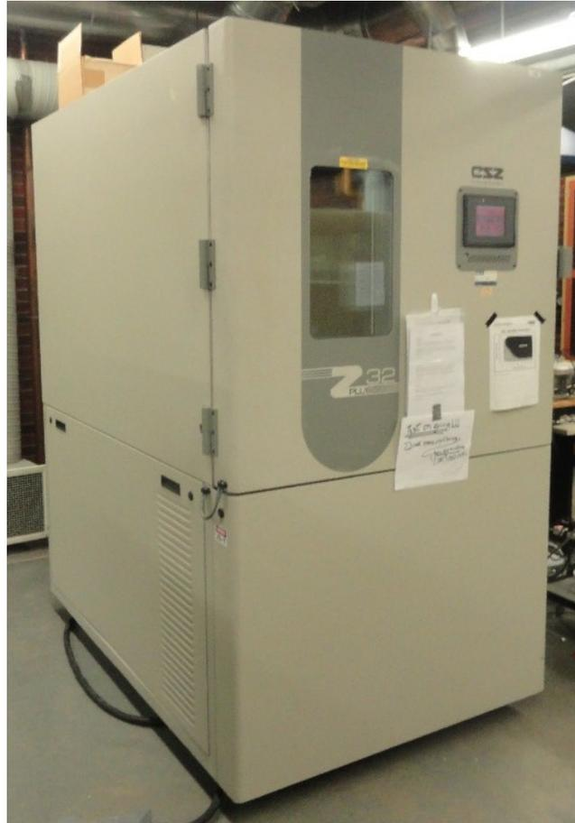
Figure 5.8 Environmental chamber used to expose the specimens to a controlled mild condition.
