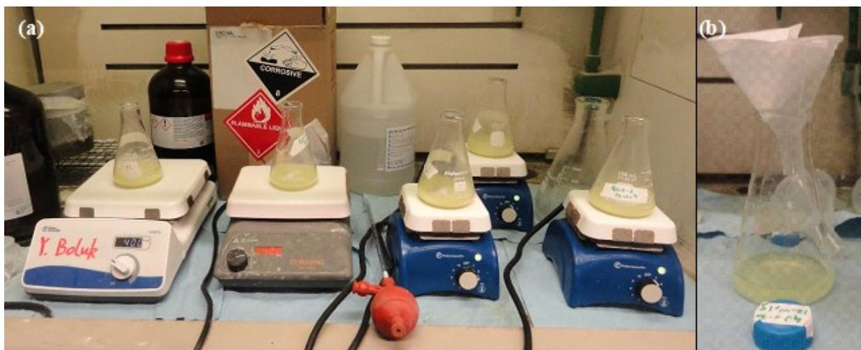
Figure 6.2.(a) Sample digesting in  $HCl$ , and (b) filtrating the  $BaSO_4$  precipitate.
