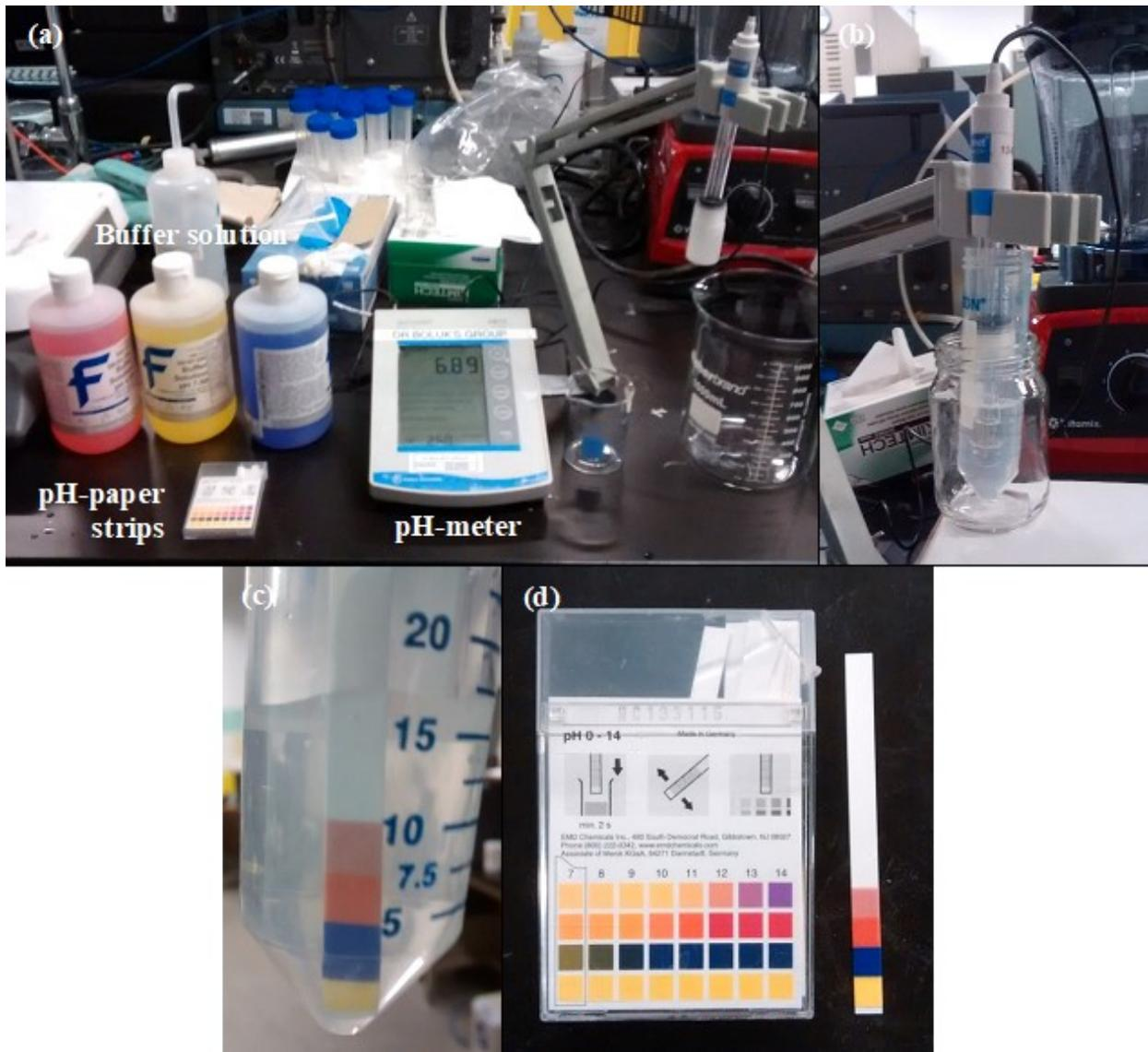
Figure 6.28.(a) pH-meter (and the pH-indicator strips). (b) Probe sensor of pH-meter inserted in the filtrated to measure the pH. (c) pH-indicator strips immersed in the filtered. (d) Measurement of pH by matching the colours of the indicator strip with the shades in the colour chart.
