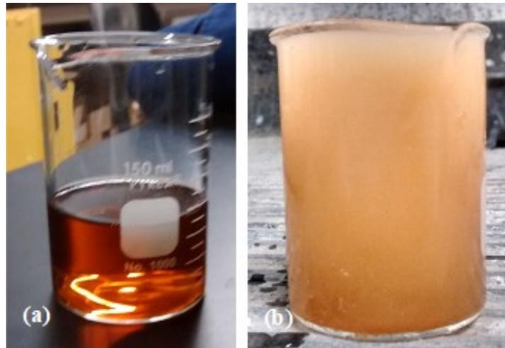
Figure 3.11 View of the superplasticizer (a) before and (b) after the manual mixing with around 1/3 of the CNF-mixing water pre-mixture.
