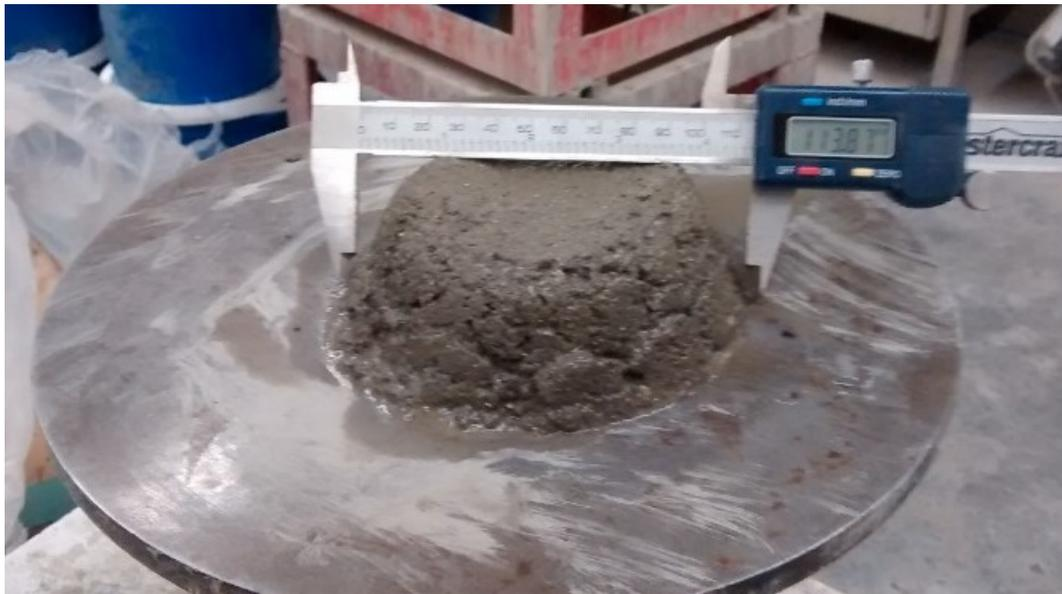
Figure 3.7 View of the flow table test apparatus used to determine the consistency of mortars.
