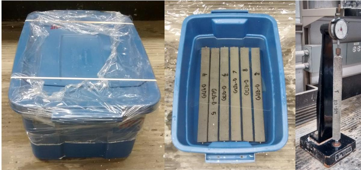
Figure 6.10 View of (a) the sealed container, (b) the prisms immersed in  $Na_2SO_4$  solution, and (c) the length comparator used to measure the length change of prisms.
