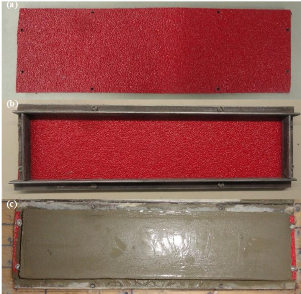
Figure 5.12 View of (a) the sandpaper, (b) the mold ready for casting, and (c) the paste specimen without the mold sides and the sandpaper ends fastened with screws to mold base.
