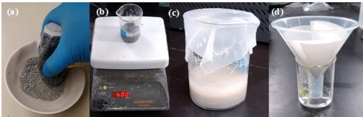
Figure 6.27 Sample preparation for pH analysis: (a) grinding; (b) stirring the powder dispersed in distilled water; (c) soaking period; and (g) filtrating the solid part of the dispersion.
