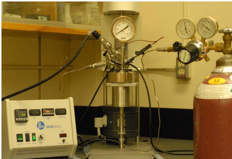
Figure 3-3 Bench-top autoclave used for pressurizing the tailings with CO<sub>2</sub>.
