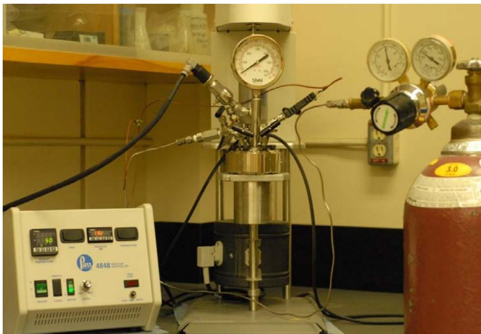
Figure 3-3 Bench-top autoclave used for pressurizing the tailings with CO<sub>2</sub>.
