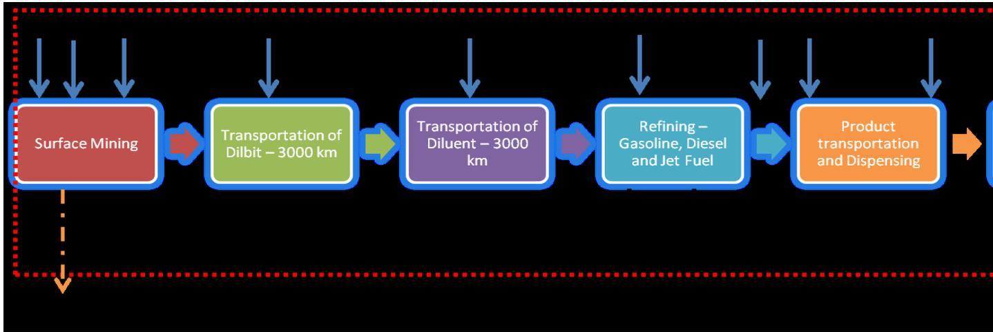
**Figure 2 (F): Pathway 6- Surface-mined bitumen is transported as dilbit to refineries and refined to produce gasoline and diesel.**
