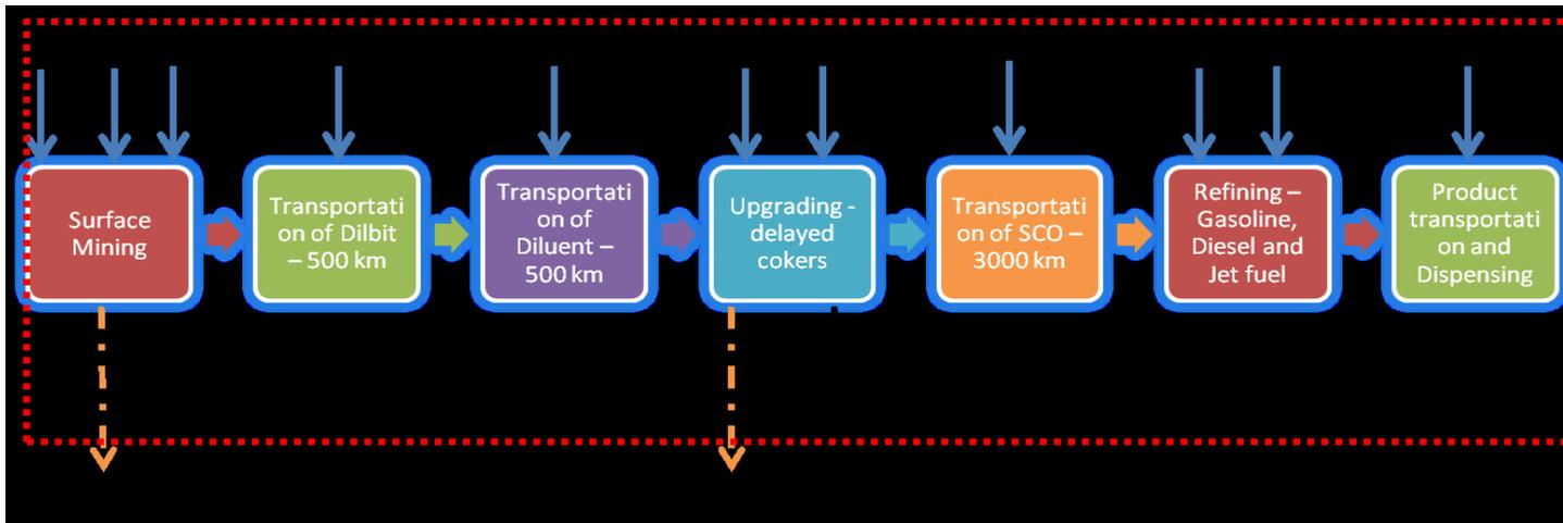
**Figure 2 (A): Pathway 1- Surface-mined bitumen is upgraded in delayed cokers and the produced SCO refined to gasoline and diesel.**
