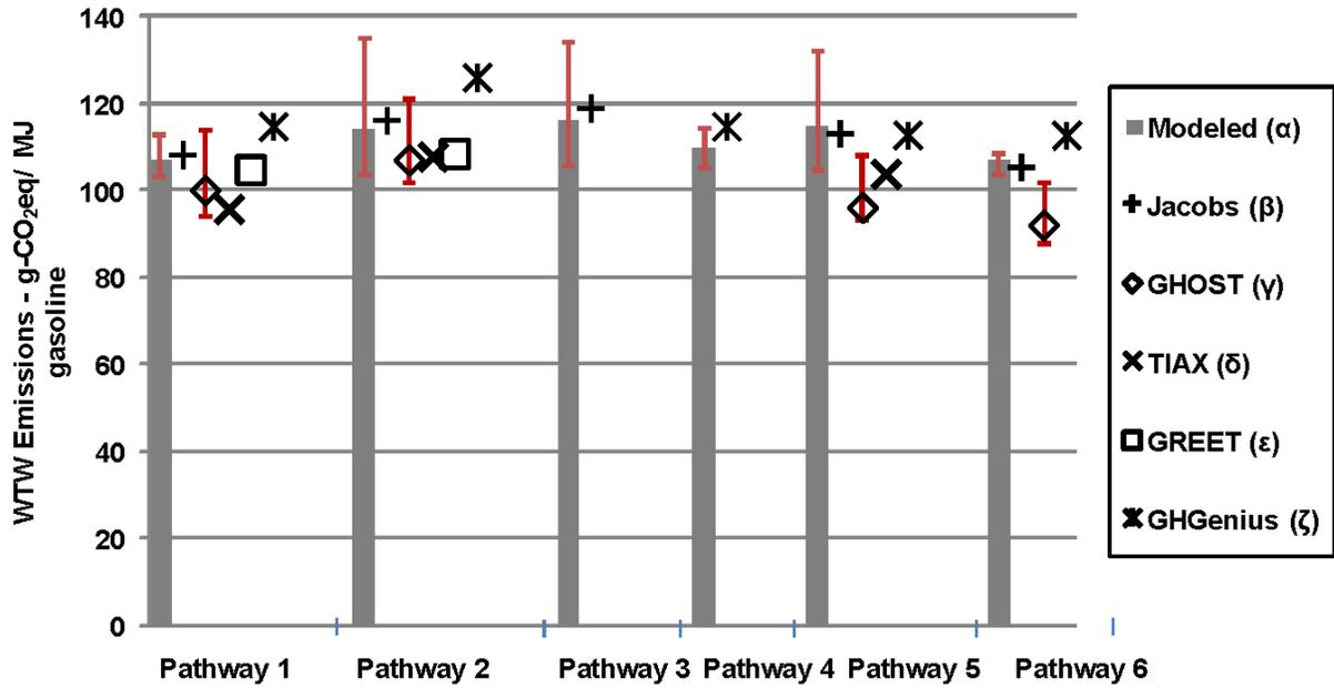
Figure 4: Comparison of modeled WTW GHG emissions for gasoline with literature values
