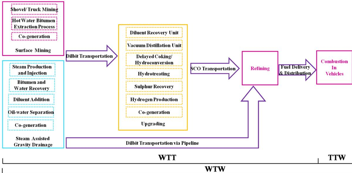
**Figure 1: WTW diagram for the bitumen life cycle showing the different unit operations of recovery, extraction, upgrading, transportation, refining, and combustion along with the involved subunit operation in each unit operation.**
