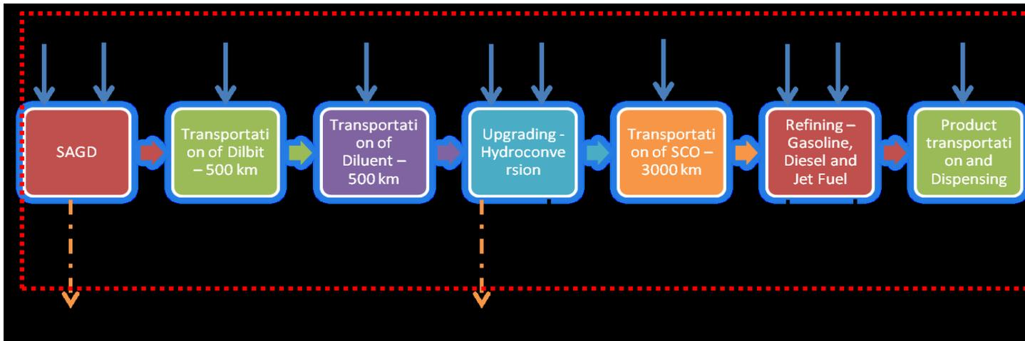
**Figure 2 (C): Pathway 3- Bitumen recovered in SAGD is upgraded through hydroconversion and the produced SCO refined to diesel and gasoline.**
