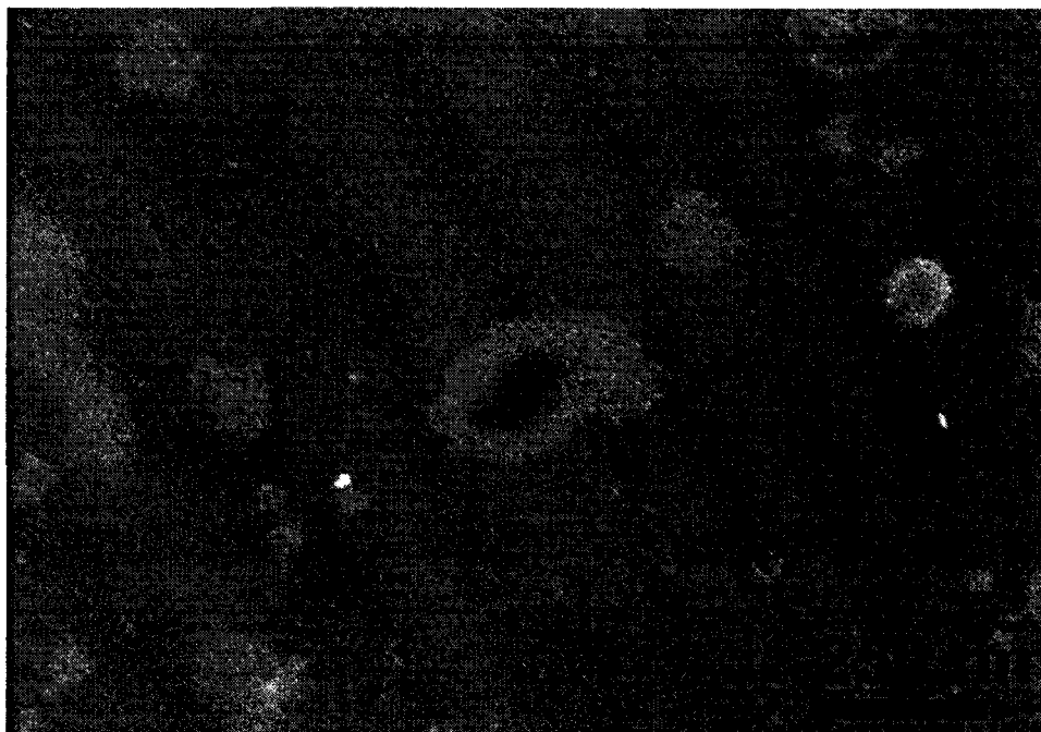
Figure 2.7. SEM image showing no RNTs obtained from G ^ C base 7 (0.25mg/mL, 24 hours) cast from methanol on carbon coated grid.
