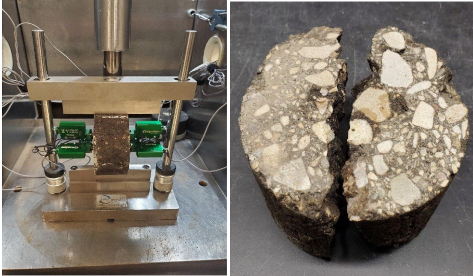
Figure 2-5: ITS test specimen testing and specimen after testing
