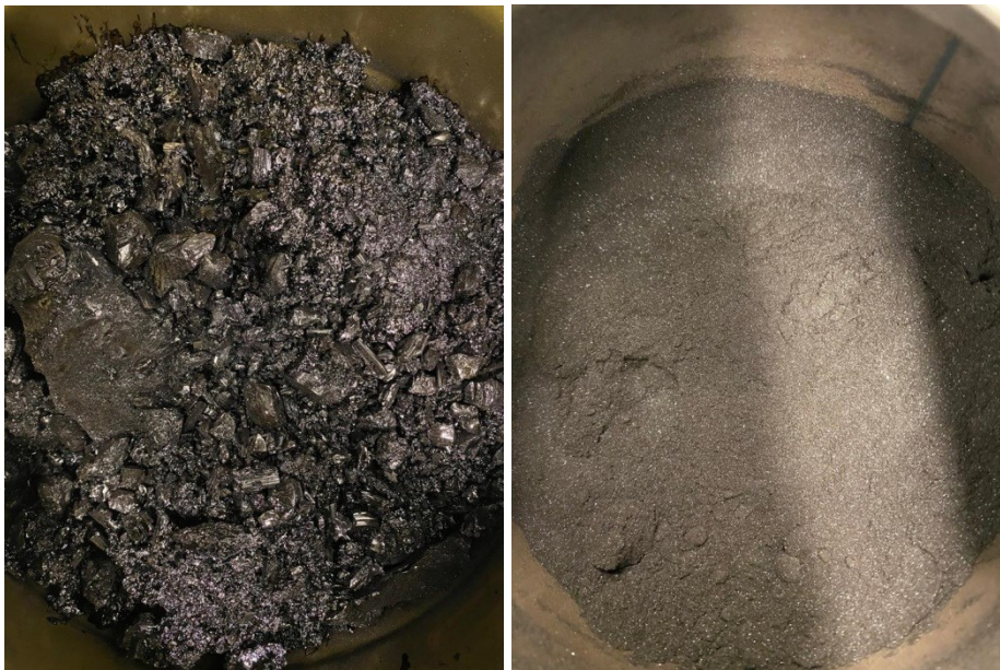
Figure 4-2: Source 1 type of Asphaltenes. ((a) solid & (b) Powdered)
