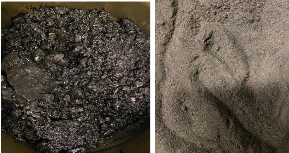
Figure 3-1 Asphaltenes, solid asphaltenes (left), powdered asphaltenes (right)
