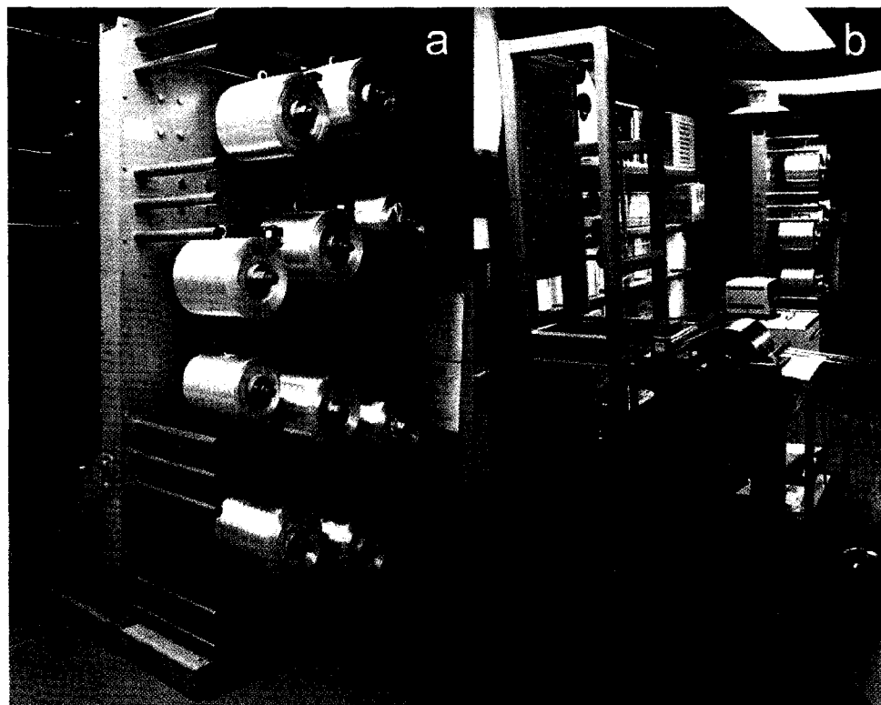
Figure A.2: Tow tensioning equipment; a) creel stand with tensioning motors, b) tow redirection stand, resin bath and resin bath heater.
