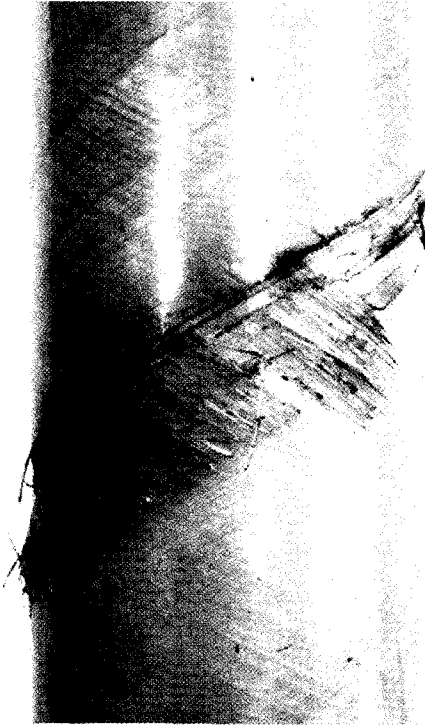
Figure 4.1: Helical crack leading to failure under the 0:1 stress ratio.
