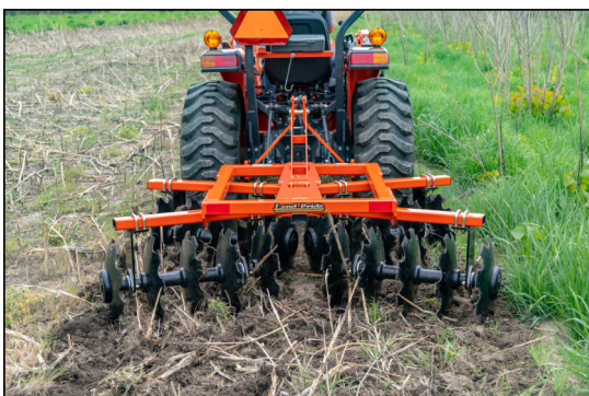
Figure 8. Disk harrow, like one used to prepare the tobacco crops supporting entomological research in North Carolina.
