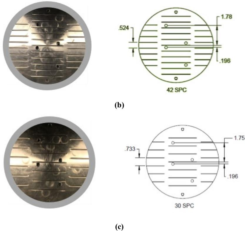
Figure 7: Image and schematics of Seamed Coupons: (a) SPC: 54, (b) SPC: 42, (c) SPC: 30
