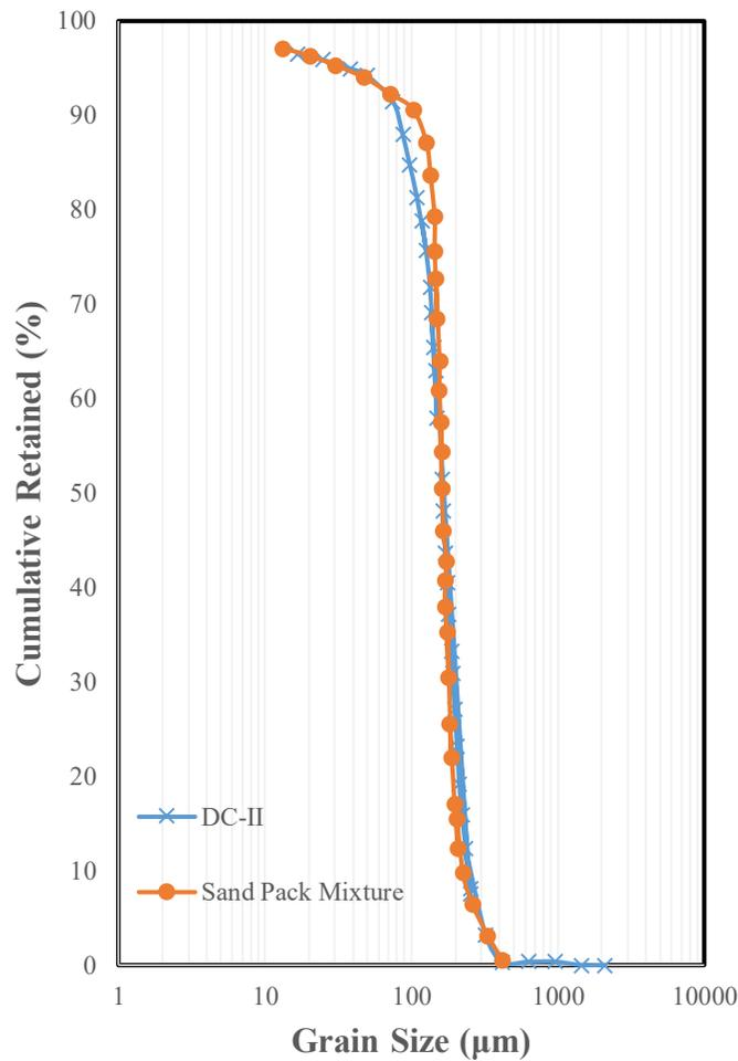
Figure 5: PSD of the Tested Sand-Pack Mixture and Class II Devon Pike 1 Project Categorized by Abram and Cain (2014)
