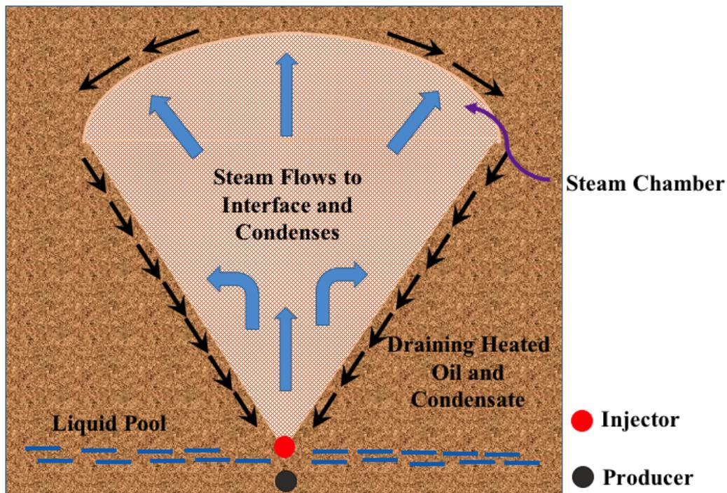
Figure 1: Schematic Concept of Steam Chamber in SAGD Operation
