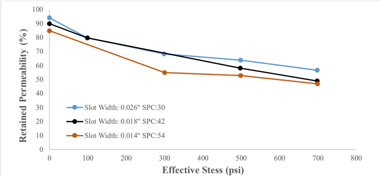
Figure 17: Retained Permeability at the Near-Coupon Zone vs. Effective Stress
