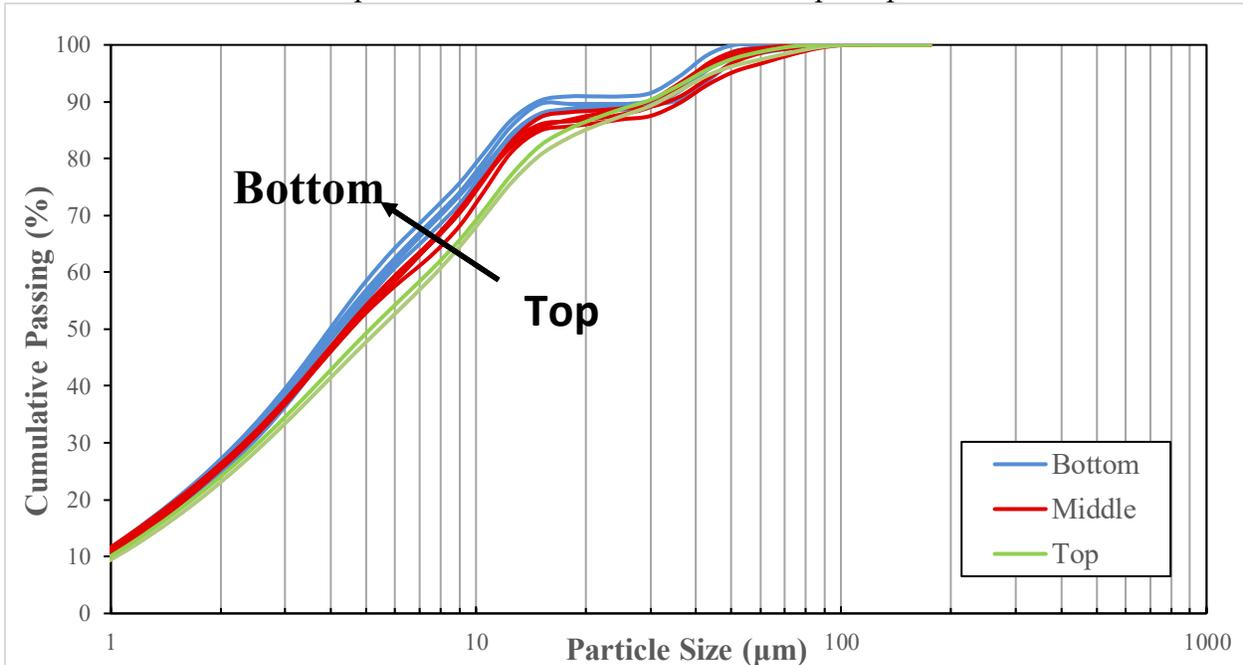
**Figure 13: PSD of Fines across the Sand-Pack for Single Flow Rate Test**
