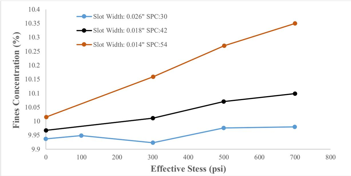
Figure 15: Fines Concentration at the Near-Coupon Zone vs. Effective Stress
