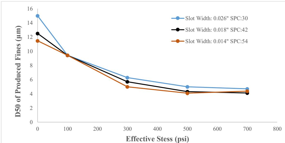
Figure 18:  $D_{50}$  of Produced Fines vs. Effective Stress
