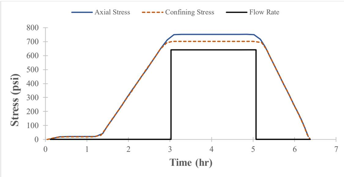
Figure 8: Example of Effective Stress (700 psi) and Flow Rate Application During SCT Test
