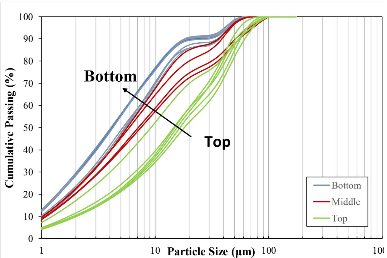
Figure 14: PSD of Fines across the Sand-Pack for Multi-Flowrate Test
