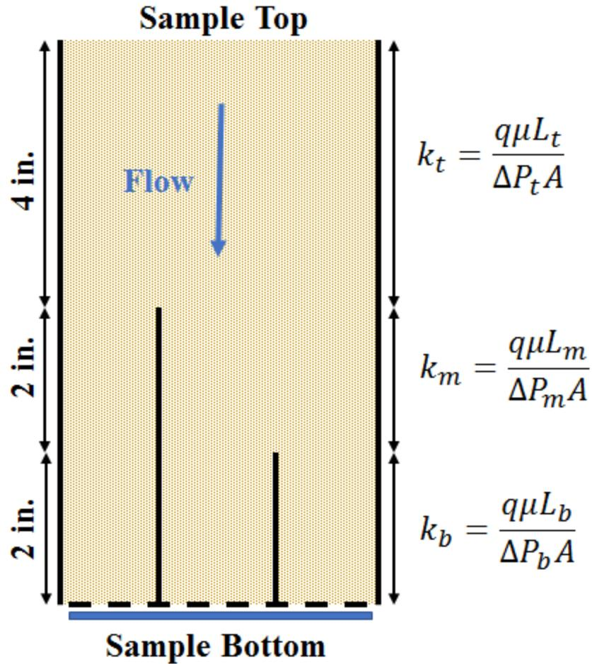
**Figure 16: Retained Permeability Definition**
