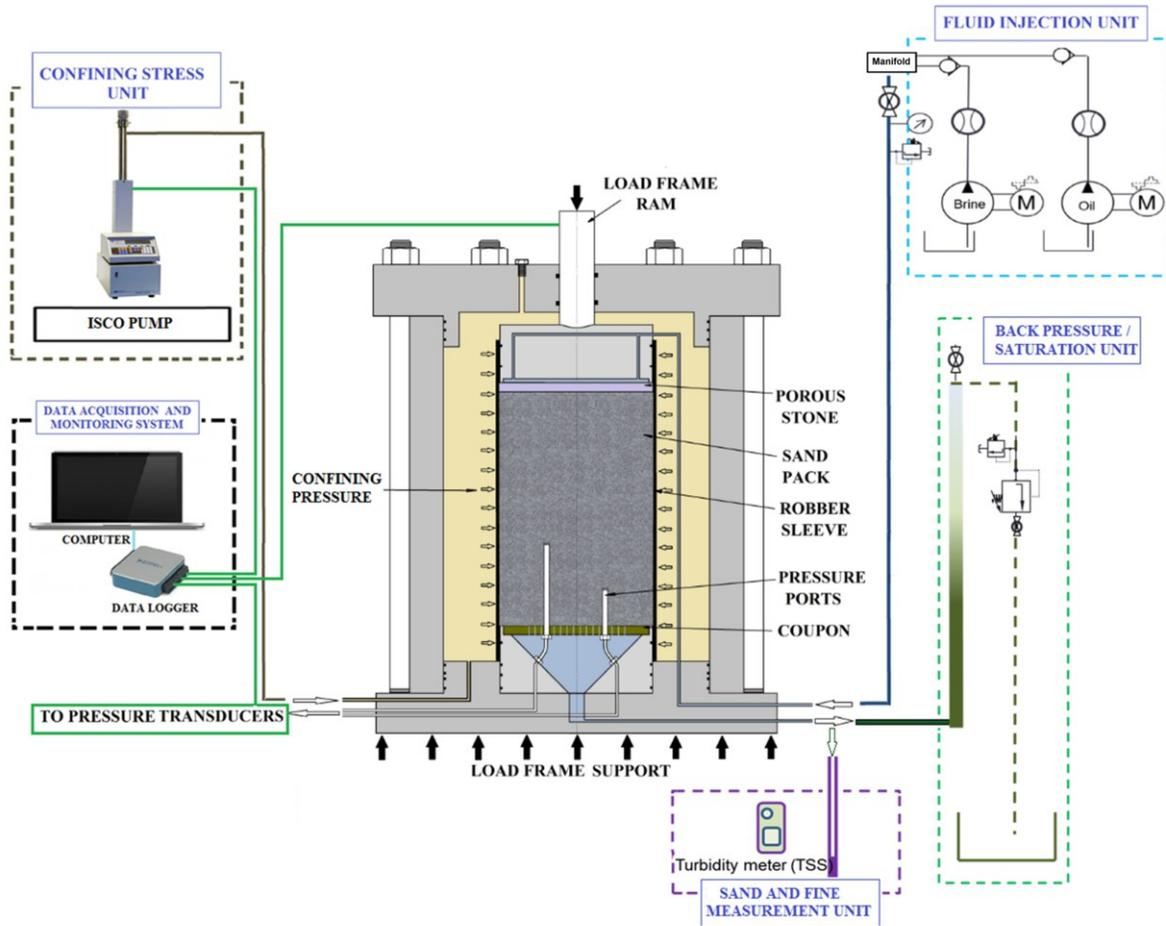
**Figure 3: Schematic View of Different Units of the SCT Facility (after Fattahpour et al., 2016)**
