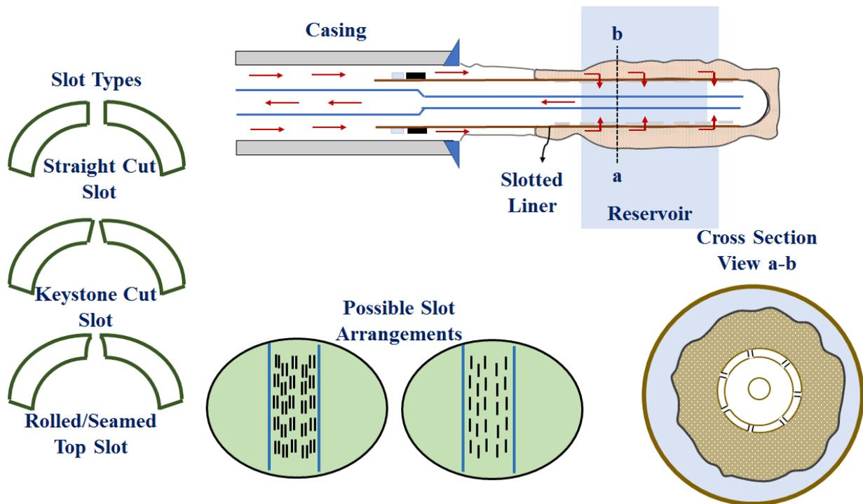
Figure 2: Configurations of Slotted Liners
