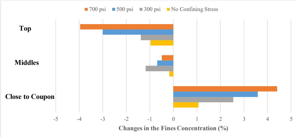
**Figure 12: Changes in Fines Concentration along the Sand-Pack under Different Effective Stresses, for Coupon: 0.014"-0.022" SPC: 54**
