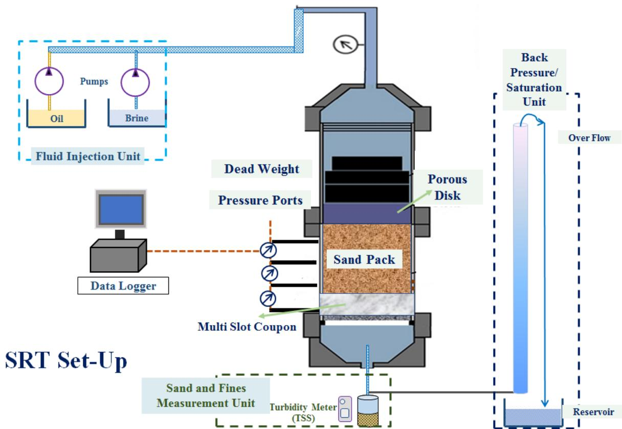
Figure 4: Schematic View of Different Units of the SRT Facility (after Fattahpour et al., 2016)
