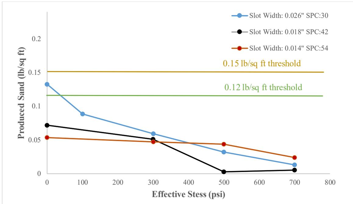
**Figure 11: Cumulative Produced Sand vs. Effective Stress; Solid Lines are the Upper Limits of Acceptable Produced Sand of 0.12 lb/sq ft and 0.15 lb/sq ft**
