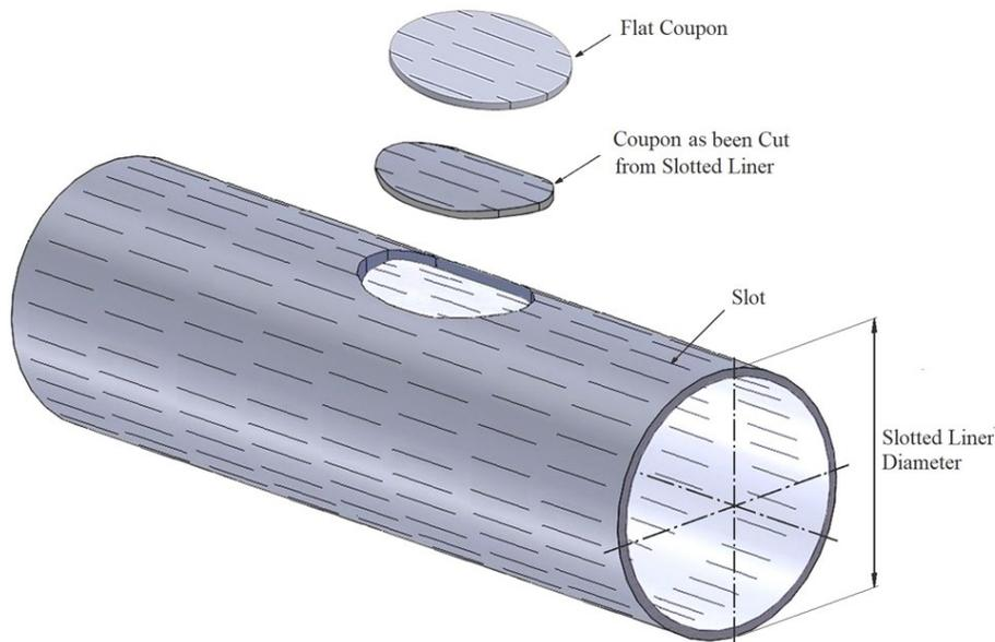
Figure 6: Schematic View of Multi-Slot Coupon as a Section of a 7-Inch Slotted Liner
