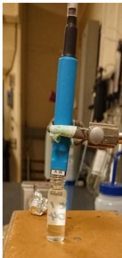
**Figure 14. The IDE setup for measuring total bacteria count (the IDE is immersed in buffer solution with different bacteria concentrations).**
