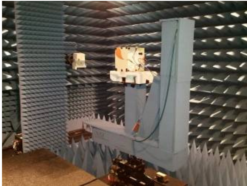
Fig. 3.32 - Photograph of the antenna array mounted on antenna measurement system.
