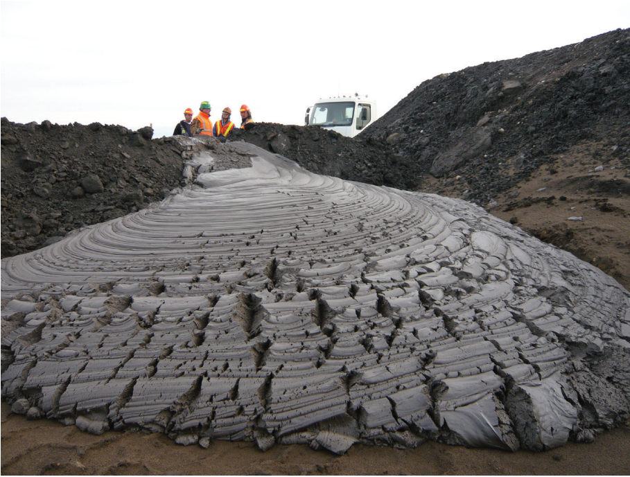
Figure 8.33 Deposited centrifuge cake following flocculation of diluted MFT.
