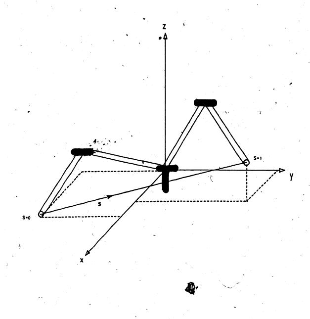
Figure III.5 Typical Three Degree of Freedom Manipulator and Typical Trajectory
