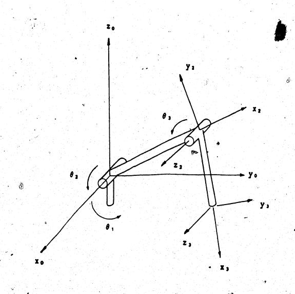
Figure III.1 Three Degree of Freedom Manipulator Used in the Analysis of Misalignments
