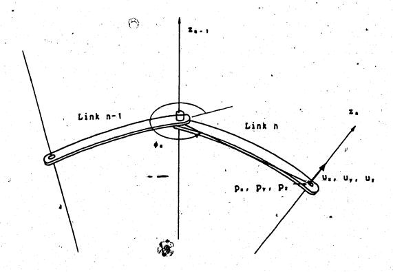
The other problem arises from the use of partial derivatives of the transform matrices in the development of the equations of motion. The partial derivatives of the Denavit-Hartenberg A matrix with respect to the joint of variable theta is
