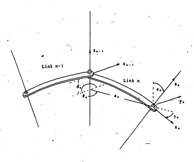
Figure II.5 Modified Denavit-Hartenberg Convention
