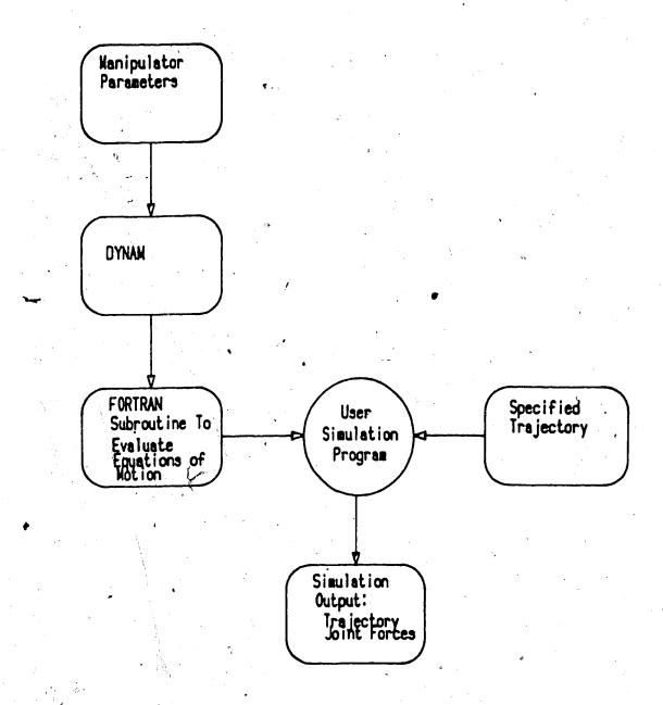
Figure III.3 The Relationship Between DYNAM and the User Simulation Program
