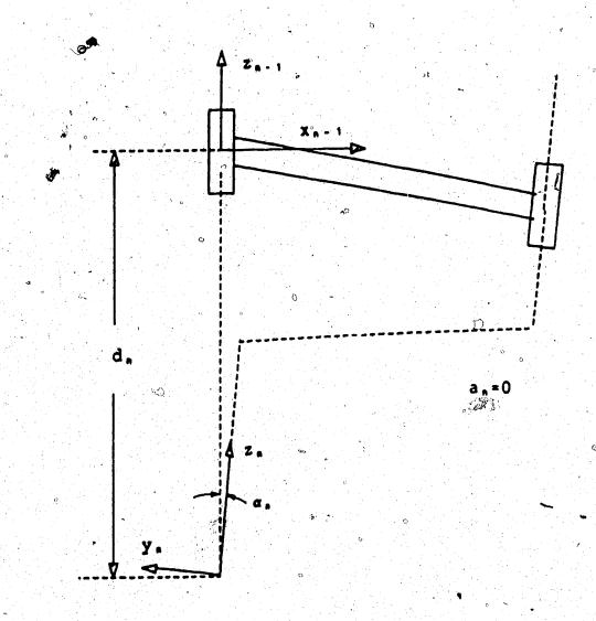
Figure II.3 The Effect of a Slight Misalignment on Coordinate System Location
