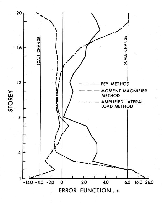
FIGURE 4.6 MOMENT ERRORS IN FRAME TYPE FIVE
