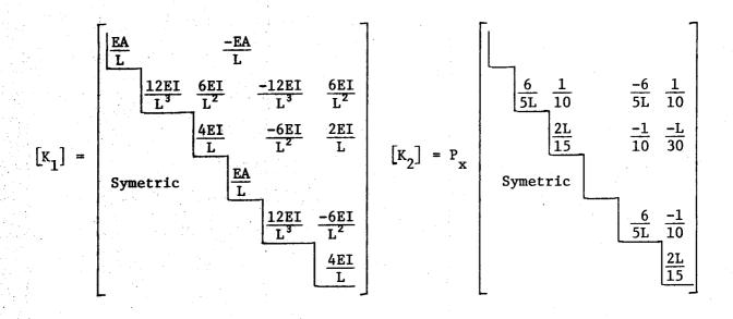
Fig. 2.7 First-Order and Geometric Stiffness Matrices
