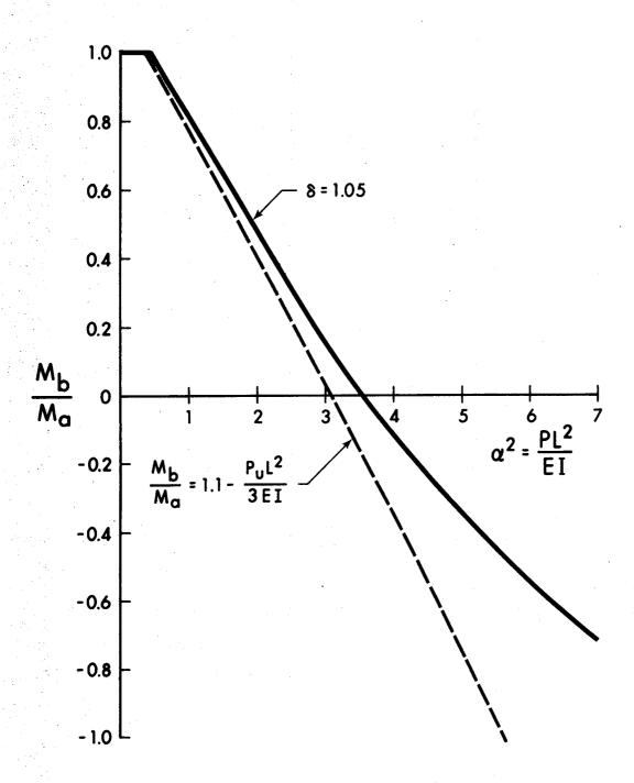
FIGURE 5.2 LIMITS ON COLUMNS WITH MAXIMUM MOMENT AT END OF COLUMN
