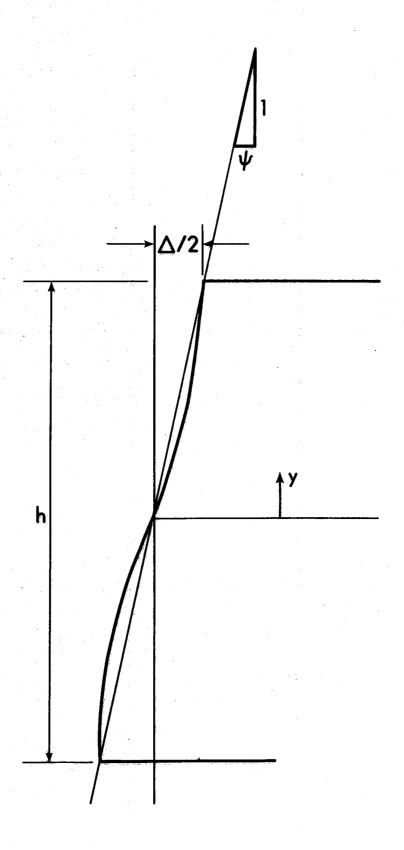
FIGURE 2.2 ISOLATED COLUMN WITH RIGID BEAMS
