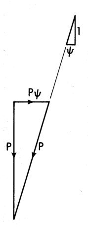
FIGURE 2.1(b) DECOMPOSITION OF VERTICAL LOAD
