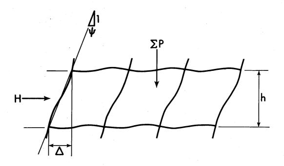
FIGURE 2.1(a) STOREY UNDER COMBINED LOAD
