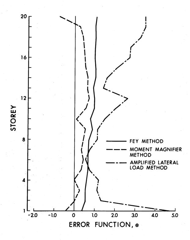
FIGURE 4.2 MOMENT ERRORS IN FRAME TYPE ONE
