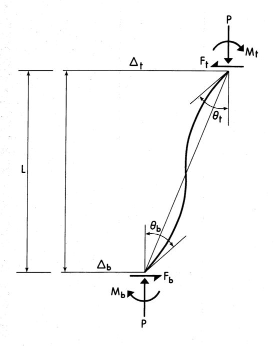
FIGURE 2.5 DEFORMED COLUMN
