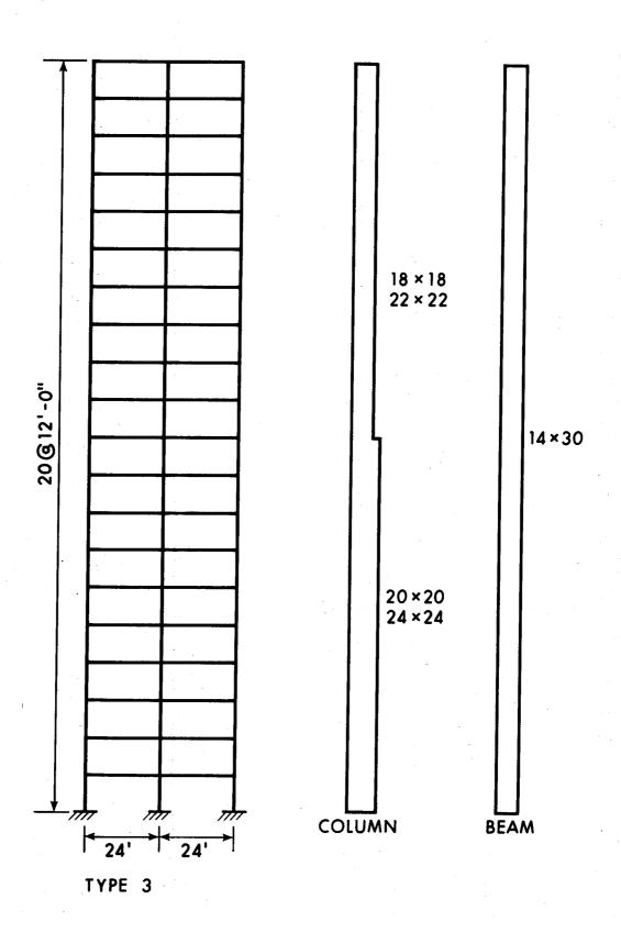
FIGURE 3.2 ELEVATION OF FRAME TYPE THREE
