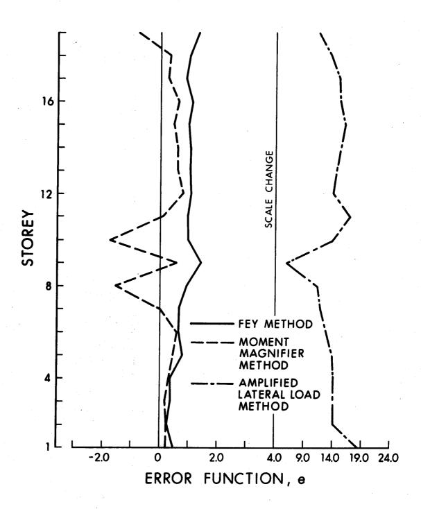
FIGURE 4.10 MOMENT ERRORS IN FRAME TYPE NINE
