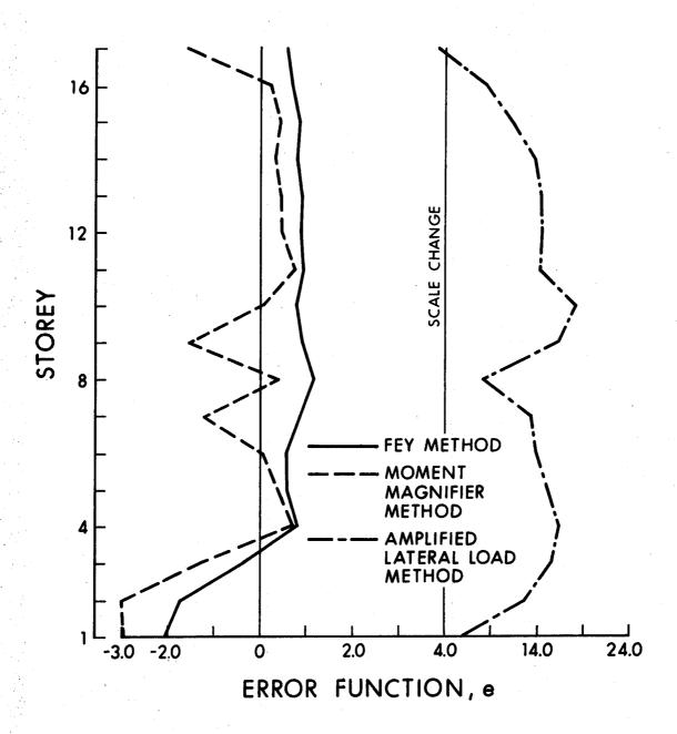
FIGURE 4.11 MOMENT ERRORS IN FRAME TYPE TEN
