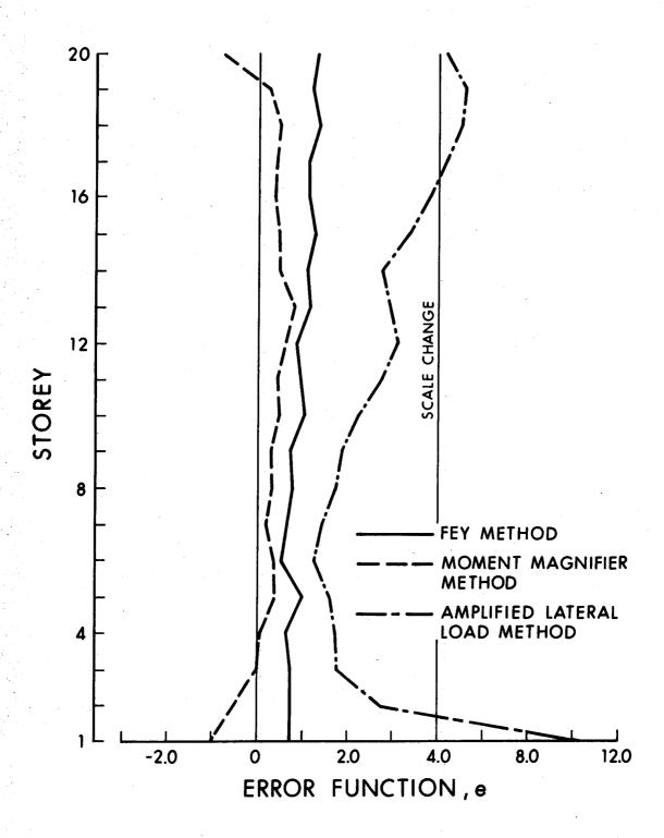
FIGURE 4.5 MOMENT ERRORS IN FRAME TYPE FOUR
