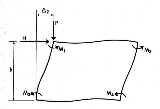
FIGURE 1.1 DEFORMED STOREY UNDER COMBINED LOADING
