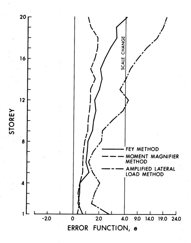
FIGURE 4.12 MOMENT ERRORS IN FRAME TYPE ELEVEN
