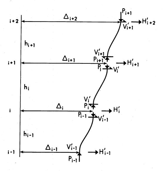
FIGURE 2.3 SWAY FORCES DUE TO VERTICAL LOADS
