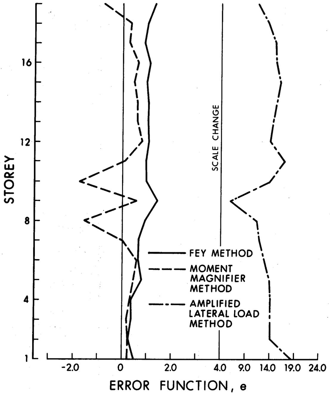
FIGURE 4.10 MOMENT ERRORS IN FRAME TYPE NINE
