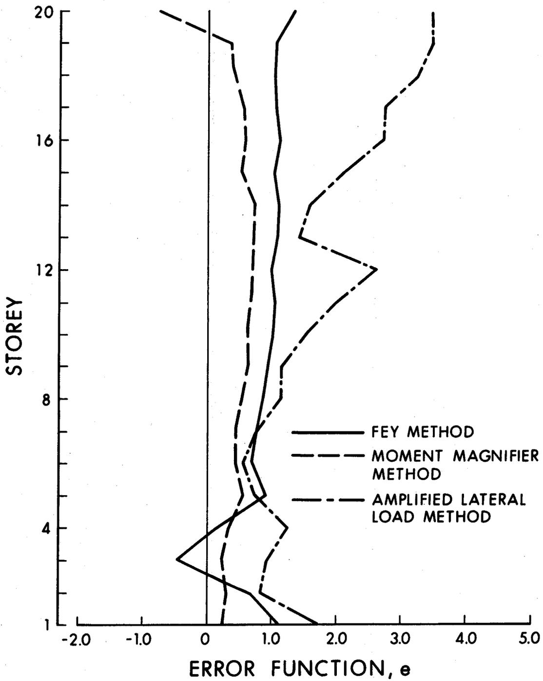
FIGURE 4.3 MOMENT ERRORS IN FRAME TYPE TWO
