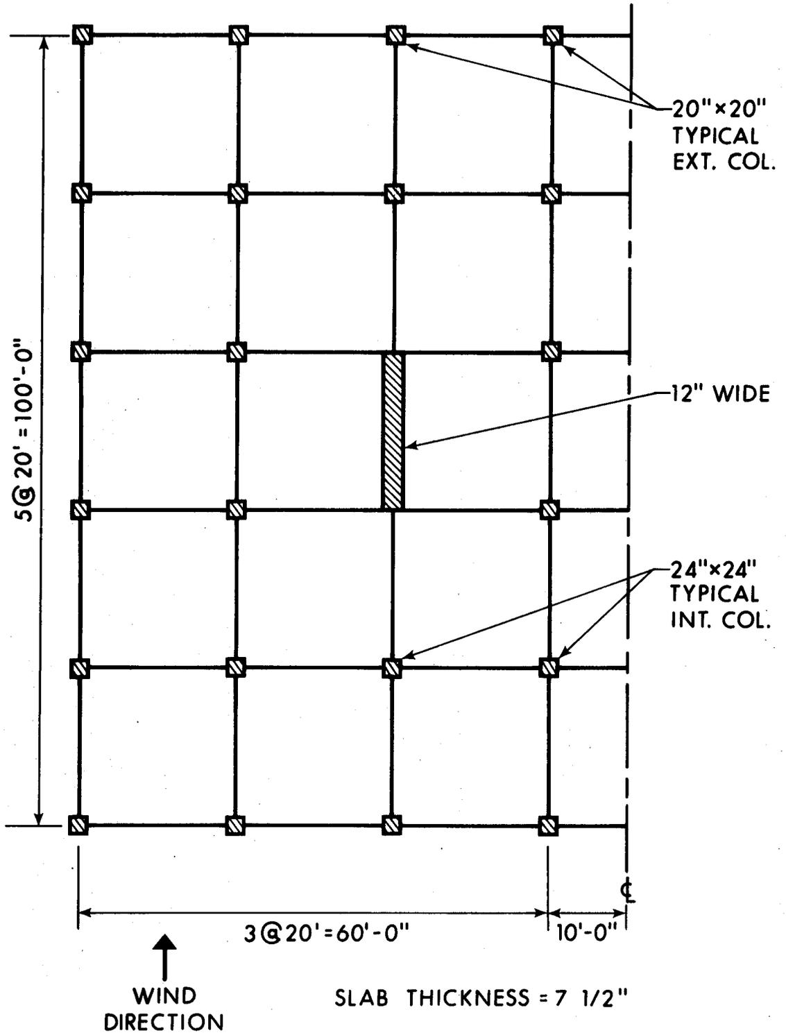
FIGURE 3.4 PLAN OF FRAME TYPE SIX
