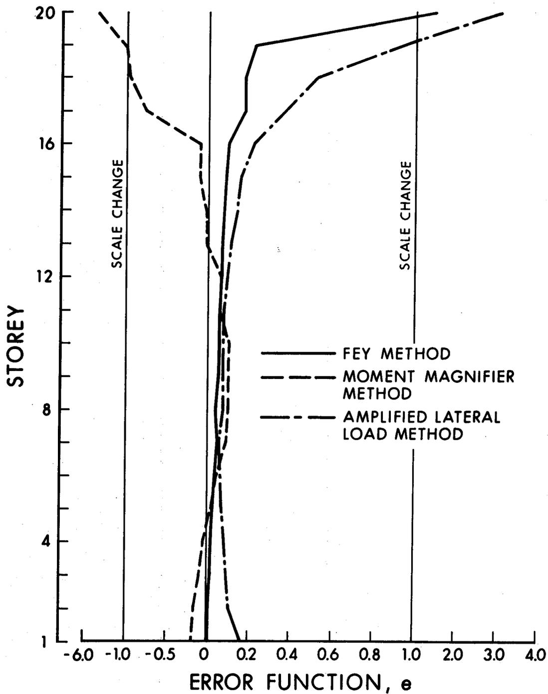
FIGURE 4.8 MOMENT ERRORS IN FRAME TYPE SEVEN
