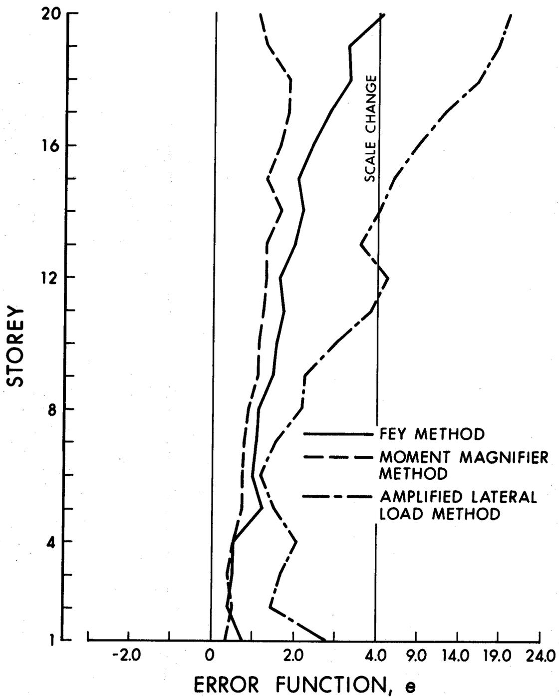
FIGURE 4.12 MOMENT ERRORS IN FRAME TYPE ELEVEN
