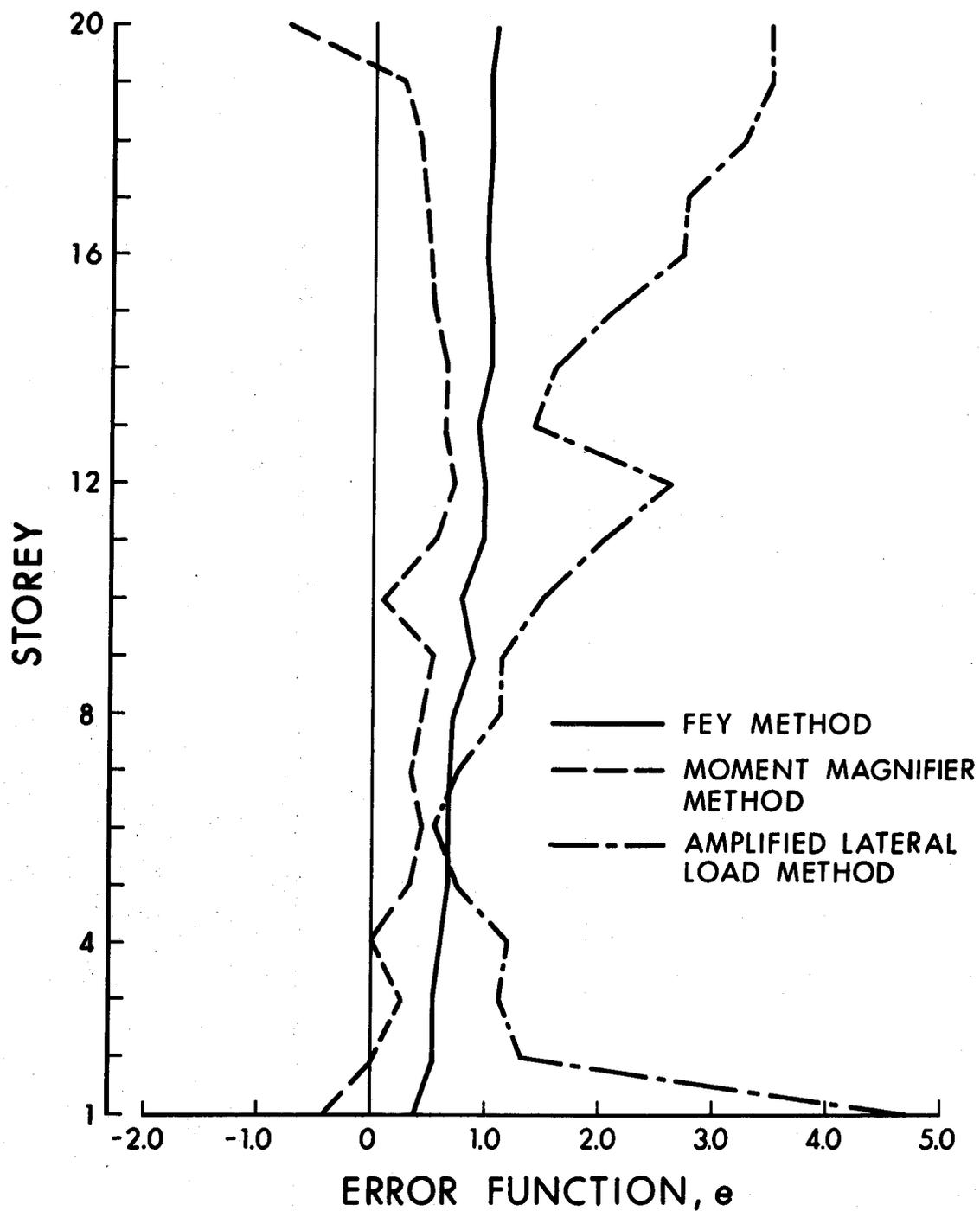
FIGURE 4.2 MOMENT ERRORS IN FRAME TYPE ONE
