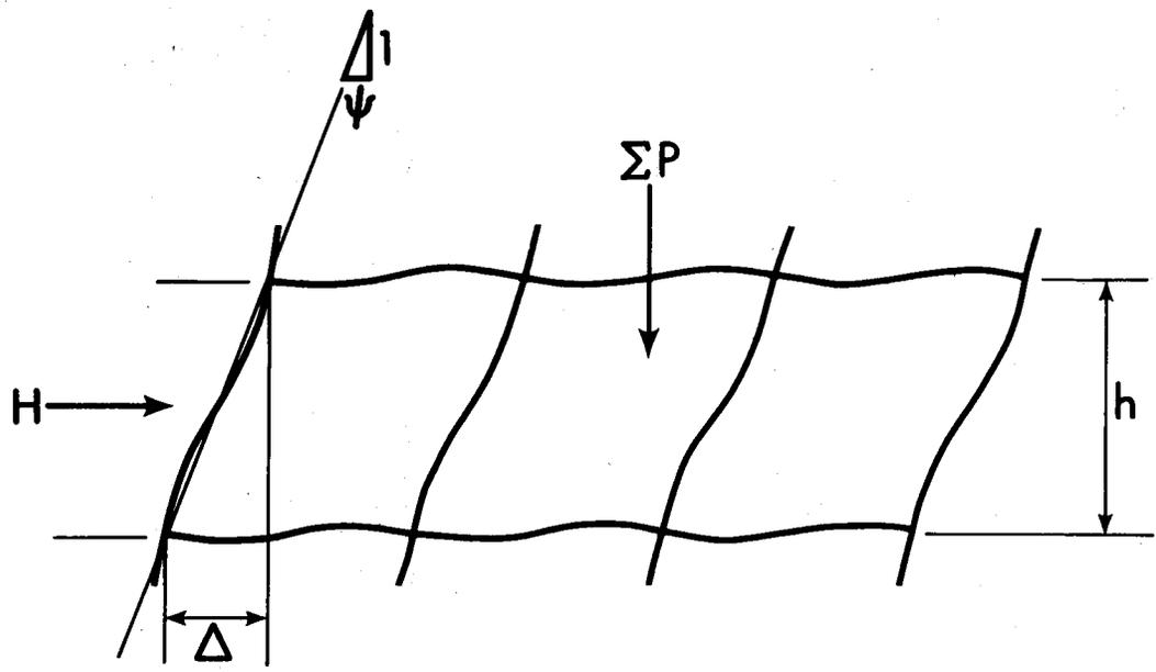
FIGURE 2.1(a) STOREY UNDER COMBINED LOAD
