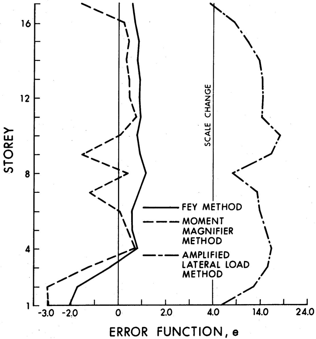
FIGURE 4.11 MOMENT ERRORS IN FRAME TYPE TEN
