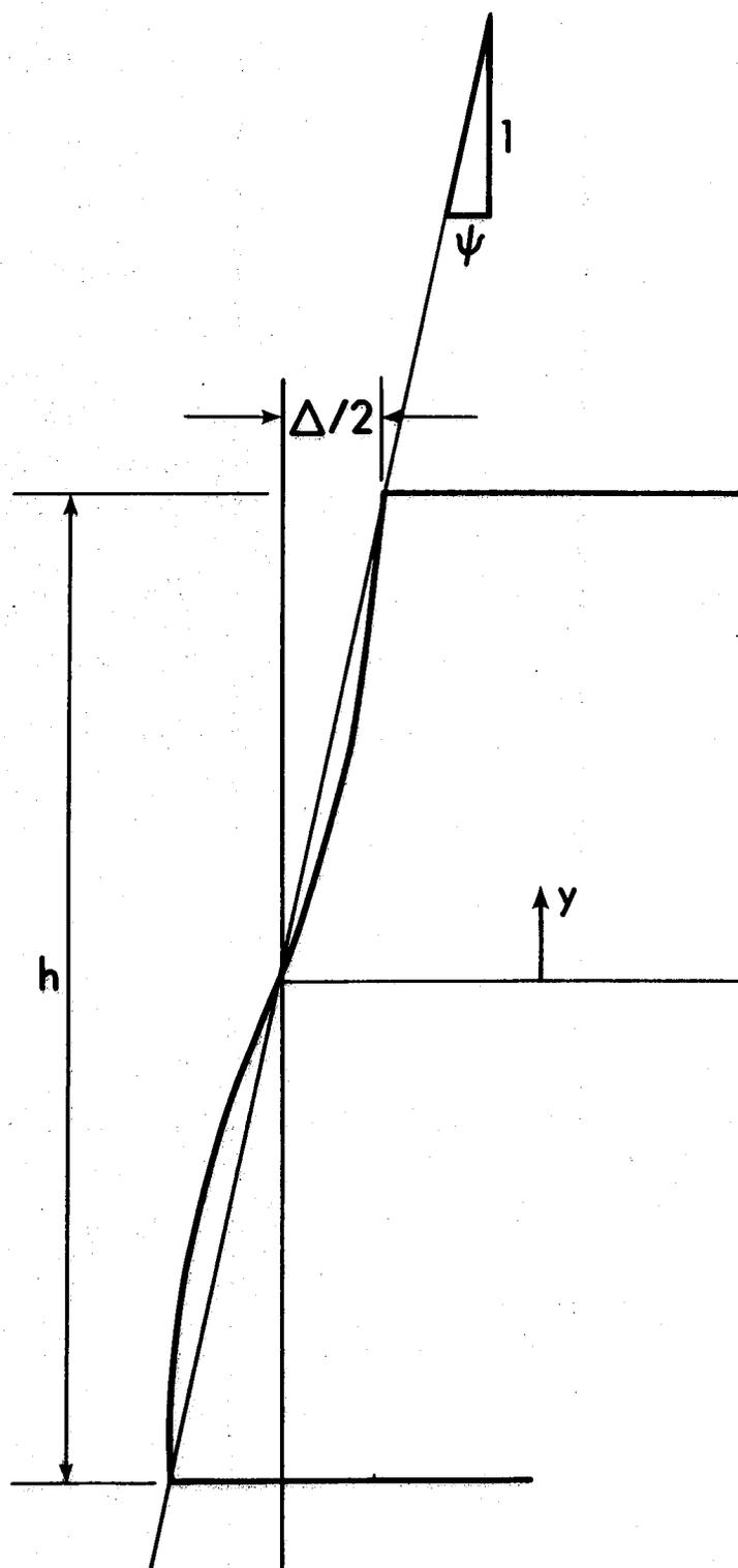
FIGURE 2.2 ISOLATED COLUMN WITH RIGID BEAMS
