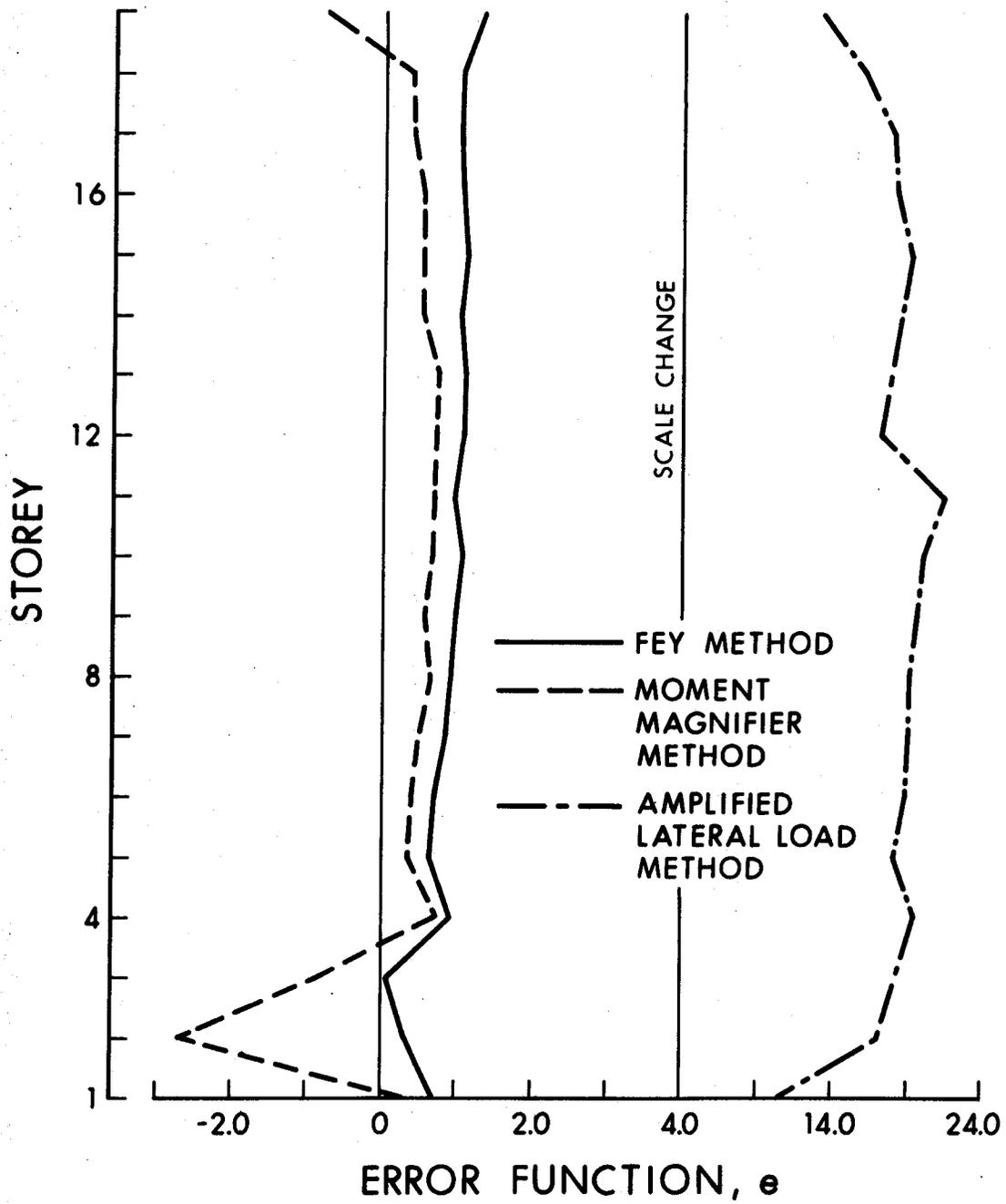
FIGURE 4.9 MOMENT ERRORS IN FRAME TYPE EIGHT
