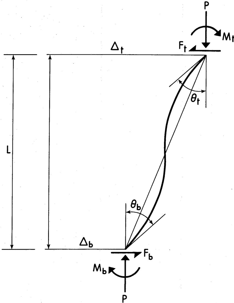
FIGURE 2.5 DEFORMED COLUMN
