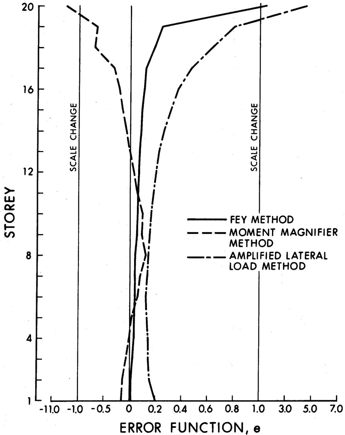
FIGURE 4.7 MOMENT ERRORS IN FRAME TYPE SIX
