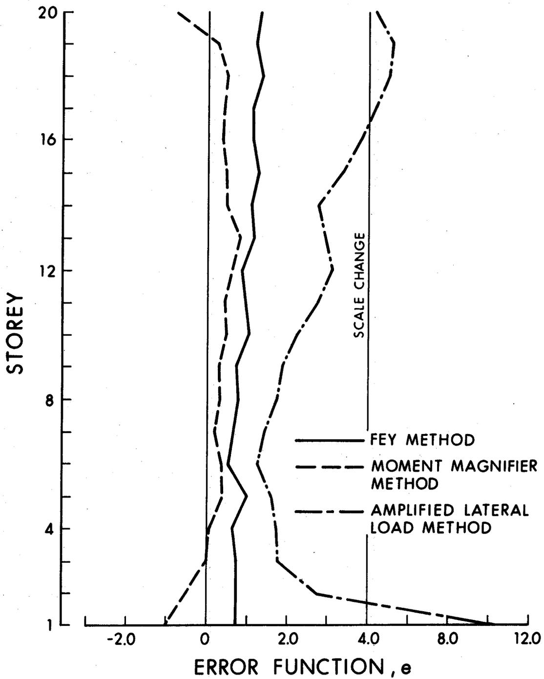
FIGURE 4.5 MOMENT ERRORS IN FRAME TYPE FOUR
