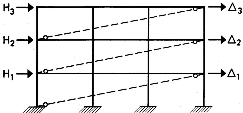
FIGURE 2.4(a) FRAME WITH NEGATIVE BRACING
