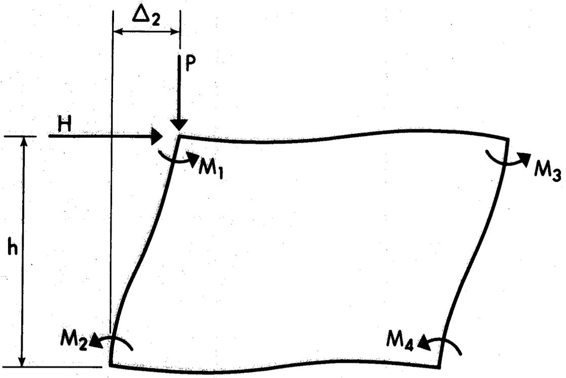
FIGURE 1.1 DEFORMED STOREY UNDER COMBINED LOADING
