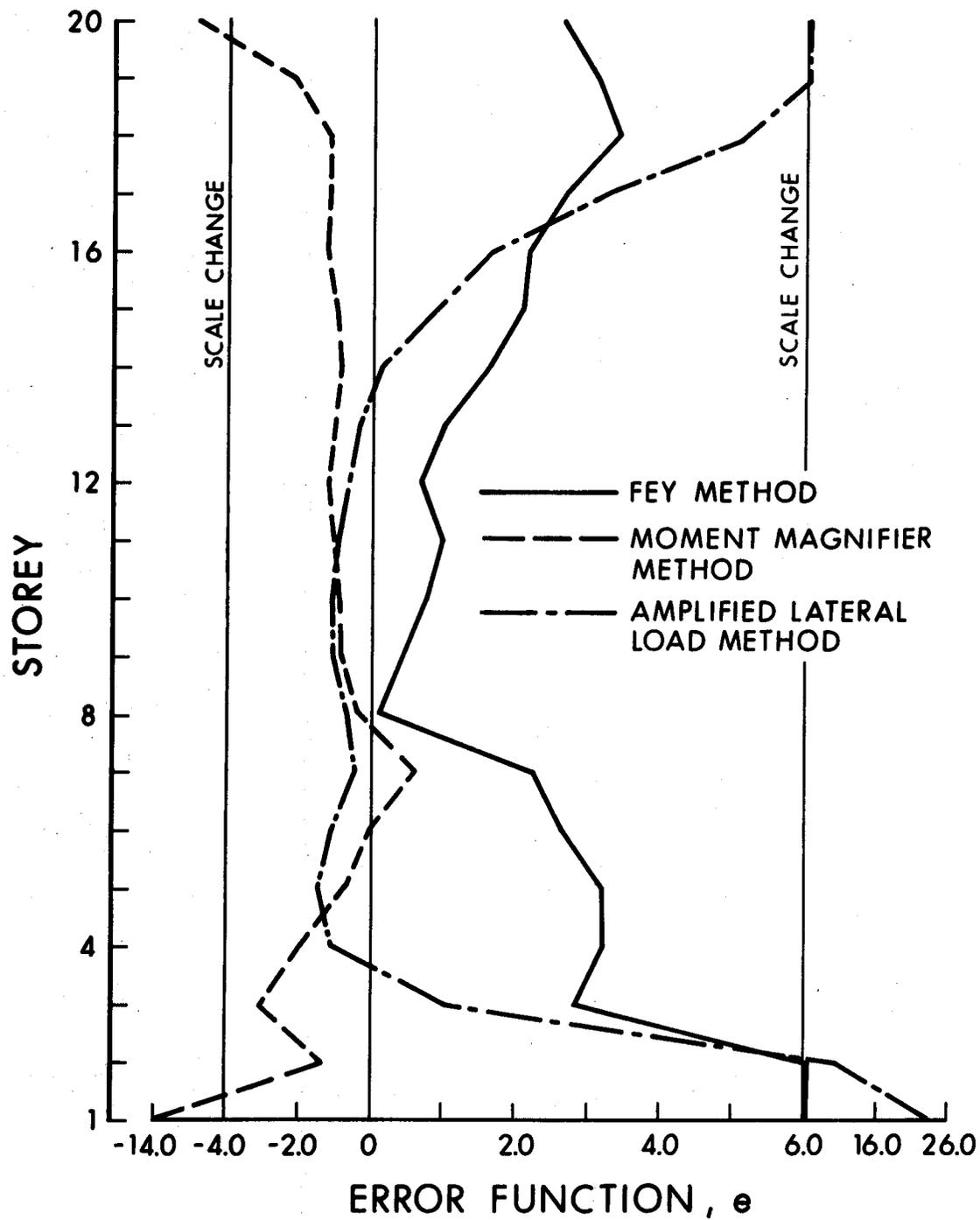
FIGURE 4.6 MOMENT ERRORS IN FRAME TYPE FIVE
