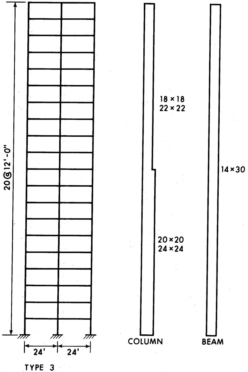
FIGURE 3.2 ELEVATION OF FRAME TYPE THREE
