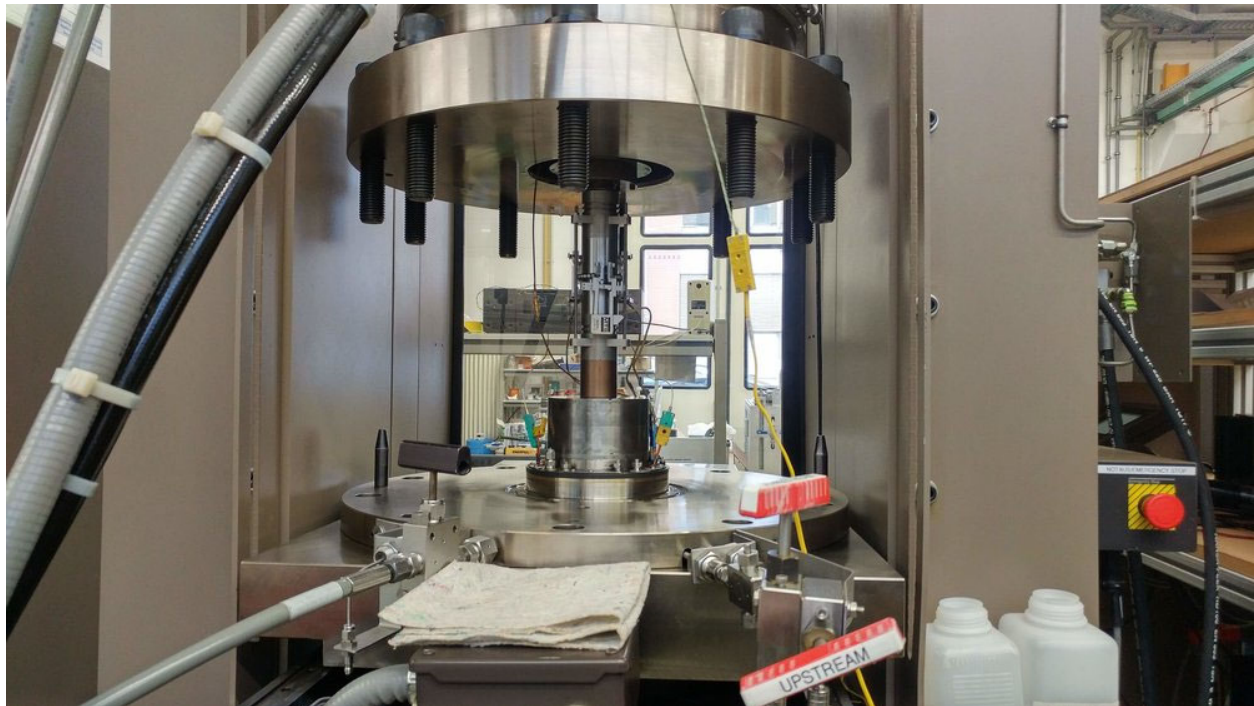
Figure A.44. Rock Mechanics Test System at the GFZ, used for determining behaviour of potential geothermal reservoir rock under stress.
