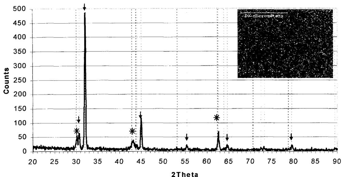
**Figure 5-14- Sample plated at 20% duty. 10:1 Sn:Cu solution in 0.2 M  $\text{H}_2\text{SO}_4$ . 25  $\text{mA}/\text{cm}^2$  average current, 50 $\text{mA}/\text{cm}^2$  peak current. (↓ = Sn phase, \* =  $\text{Cu}_6\text{Sn}_5$  phase, as determined from [Balikrisnan et al, 2003])**
