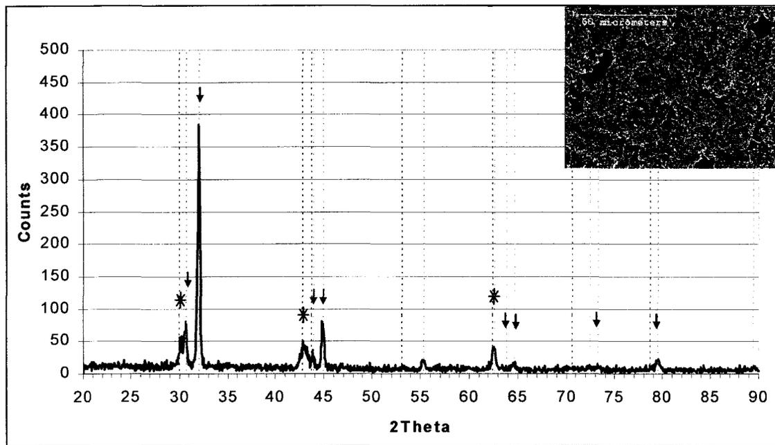
**Figure 5-12- Sample plated at 20% duty. 10:1 Sn:Cu solution in 0.2 M  $\text{H}_2\text{SO}_4$ . 10  $\text{mA}/\text{cm}^2$  average current, 50 $\text{mA}/\text{cm}^2$  peak current. (↓ = Sn phase, \* =  $\text{Cu}_6\text{Sn}_5$  phase, as determined from [Balikrisnan et al, 2003])**
