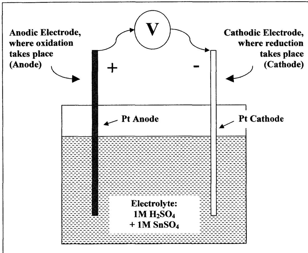
Figure 3-3 – A sample electrodeposition cell at 25°C.
