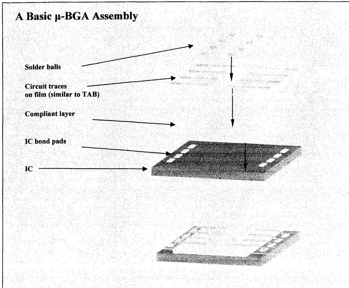
**Figure 2-3 – A basic  $\mu$ -BGA assembly contains a few essential parts, as shown above. In this example, the wires are TAB-bonded to the IC.**
