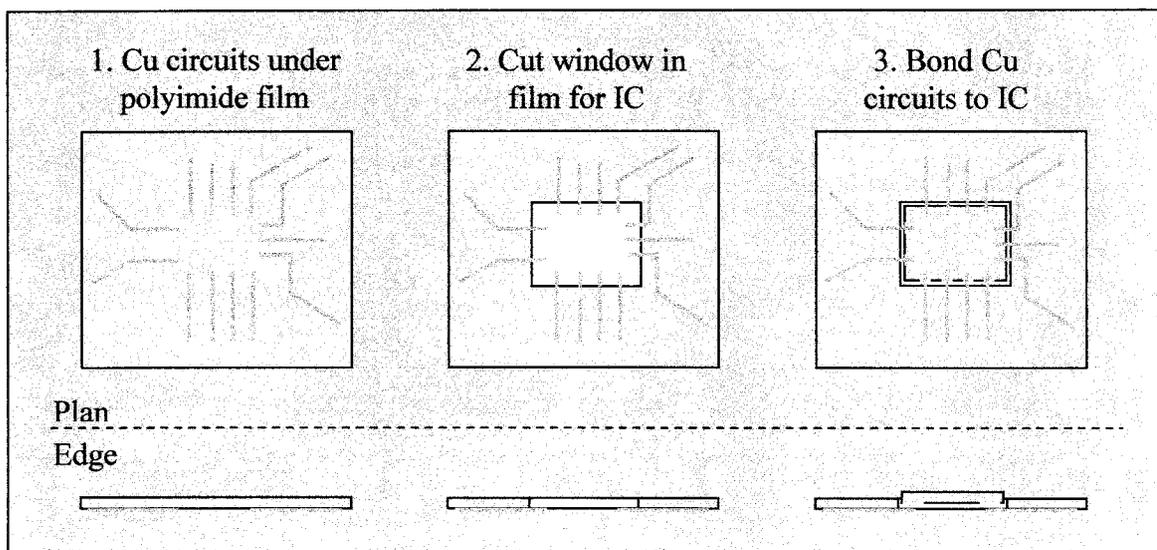
**Figure 1-5 – Major process steps for TAB bonding. Note that the IC can be bare (Level I TAB) or prepackaged (Level II TAB). This drawing is based on descriptions from [Gileo 2002], [Lau & Mayer 1990].**
