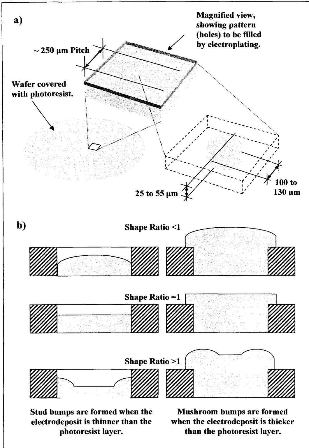
Figure 4-3 – Example of the setup used to electroplate solder bumps by Kim & Ritzdorf. The drawings are based on figures and descriptions in the text.
