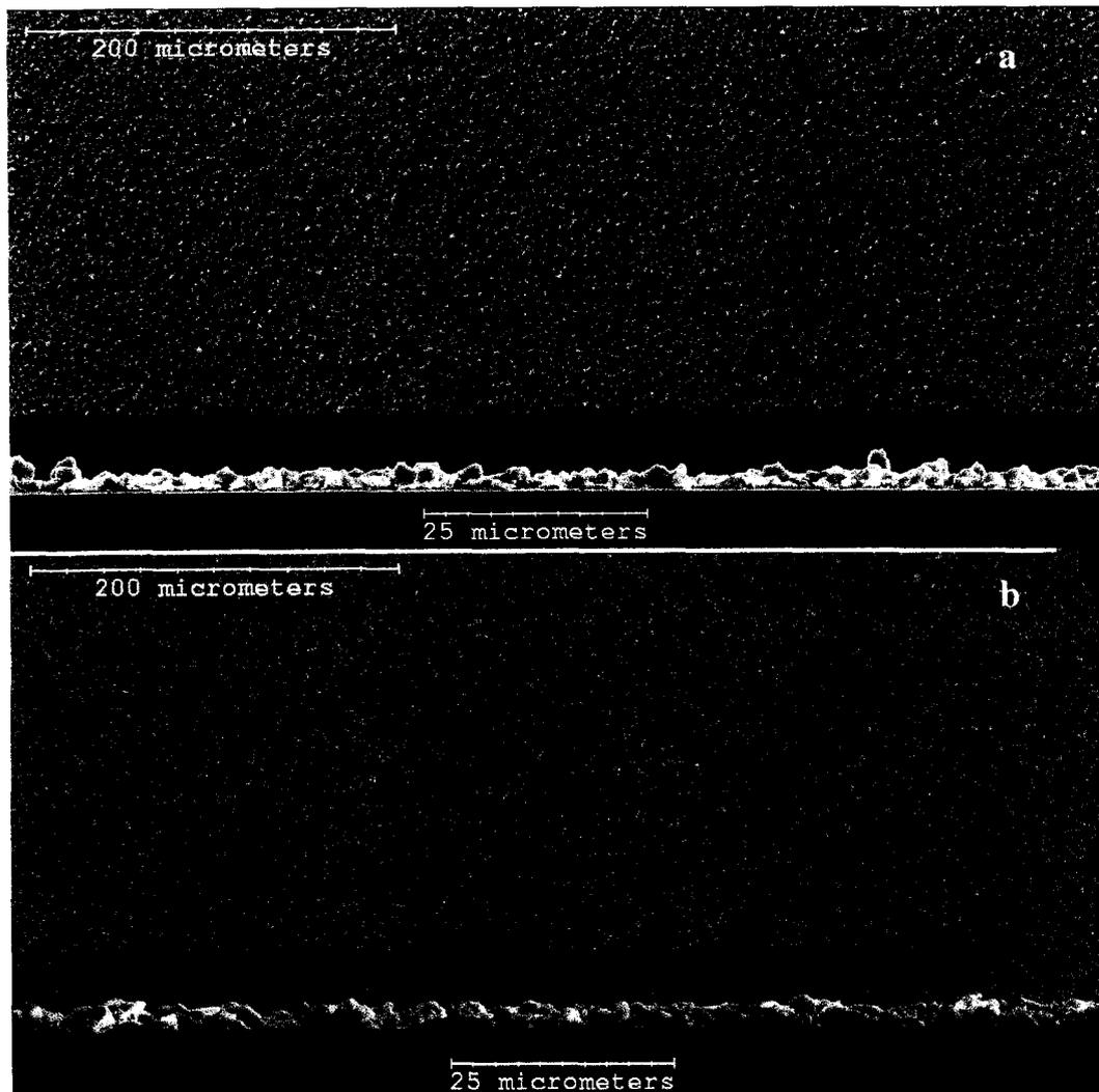
**Figure 5-10 – Plan and edge views of Sn-Cu films plated on Au with near-eutectic (0.7wt%Cu) composition. Lighter shades on the plan view indicate higher regions on the film. (a) Film containing  $0.4\pm 0.2\text{wt}\% \text{Cu}$ , plated at  $90 \text{ mA/cm}^2$  with 20% pulse duty and an agitated (200 RPM stirring) bath. (b) Film containing  $1.5\pm 0.4\text{wt}\% \text{Cu}$ , plated at  $50 \text{ mA/cm}^2$ , with 5% pulse duty and unagitated bath.**
