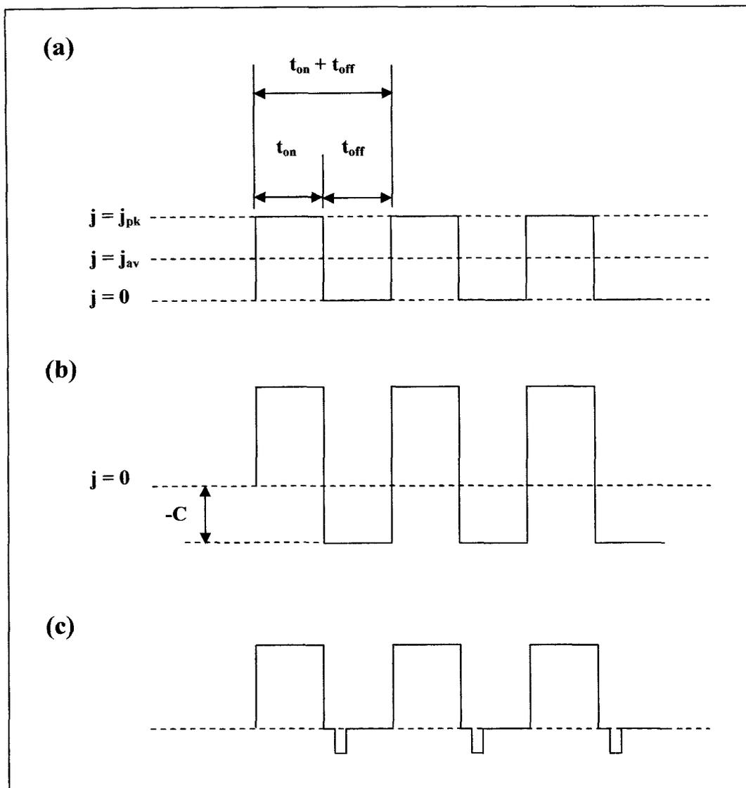
**Figure 3-7 – Illustration of various square pulse waveforms. (a) Simple square wave pulse used for experimental work in this thesis, (b) shifted square wave pulse, to allow reverse pulse plating, (c) simple square wave pulse with a short reverse pulse, used for experimental work in this thesis.**
