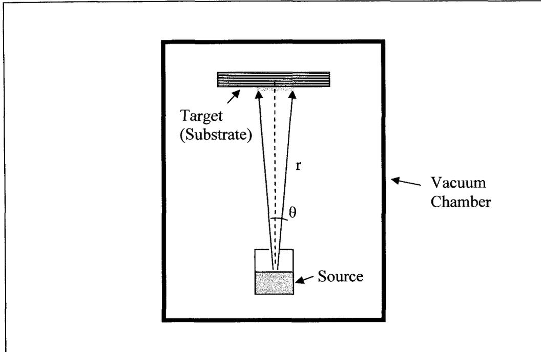
**Figure 3-1 – Schematic of an evaporation deposition process.**
