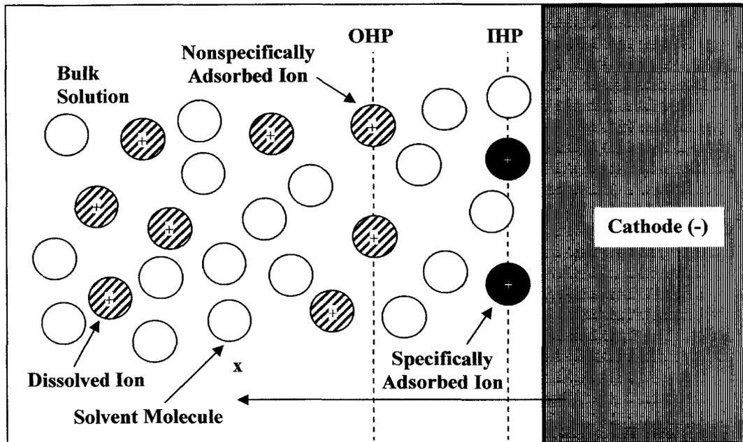
**Figure 3-4 – Diagram of the Electrical Double Layer, bounded by the Inner Helmholtz Plane (IHP) and the Outer Helmholtz Plane (OHP). The IHP contains ions that are “specifically adsorbed,” and therefore are able to be very close to the cathode surface. The OHP is the closest point to the cathode that the bulk (specifically unadsorbed) ions can reach. The distance between the IHP and the OHP is the double layer, and it acts as a capacitor that absorbs charge.**
