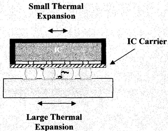
As is done between IC and carrier (Level I), underfill (dots) is added between the substrate and PWB in order to help the solder accommodate the stress. Underfilling is an expensive procedure.
