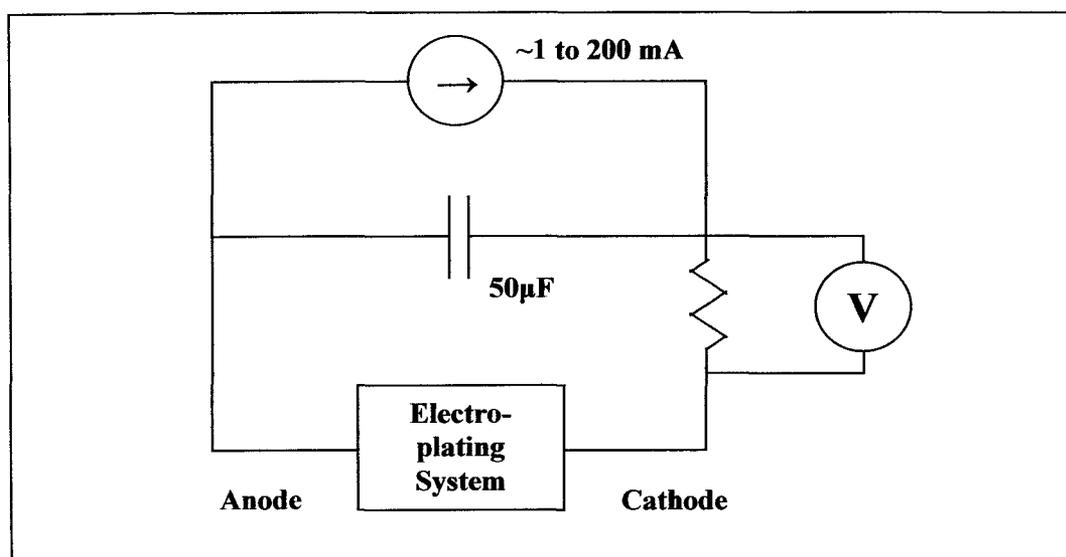
**Figure 5-3 – Schematic of electrical wiring used for experimental work.**
