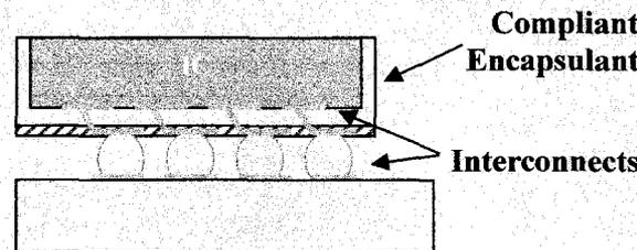
Figure 2-4 – DCA BGA (Level I and Level II) versus  $\mu$ -BGA.
