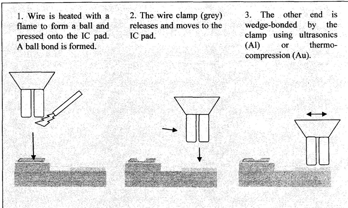
**Figure 1-3 - Method of thermal compression bonding.** As the name implies, heat and pressure are used to form both the ball and wedge bonds. An important feature is the bonding pads (red). The drawing is based on Fig 1.6 of Gilleo, 2002 and Fig 15.5 from Mayer and Lau 1990.
