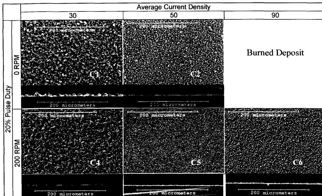
**Figure 5-6 – The effects of agitation at 20% pulse duty include better coverage and flatter films. Higher critical average current density allows faster plating and lower Cu content.**
