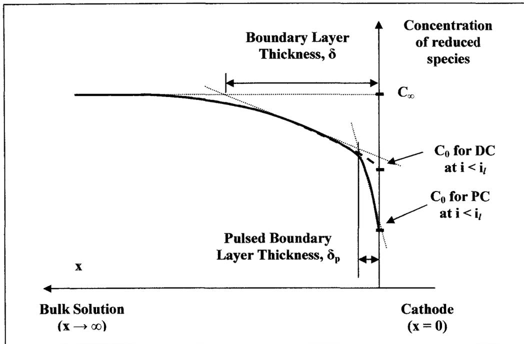
**Figure 3-8 – Pulse plating employs relatively short current pulses with greater magnitude than the average current density. [Puipe 1986-1] claims that this changes the concentration gradient near the cathode.**
