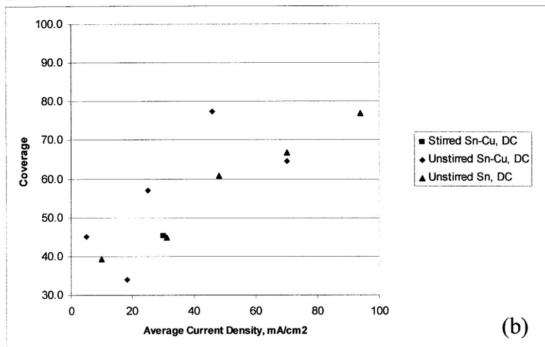
**Figure 5-8 – Coverage plots, showing that 5% pulse duty films (a) tend to have better coverage than DC films (b). DC films show a linear trend for coverage vs. average current density. Measurement error limits are within the symbol size.**
