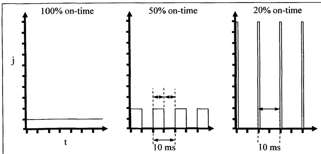
**Figure 6-1 – Example of PC plating waveforms used to deposit Sn-Cu films on Au and Cu. All three waveforms have the same average current density.**
