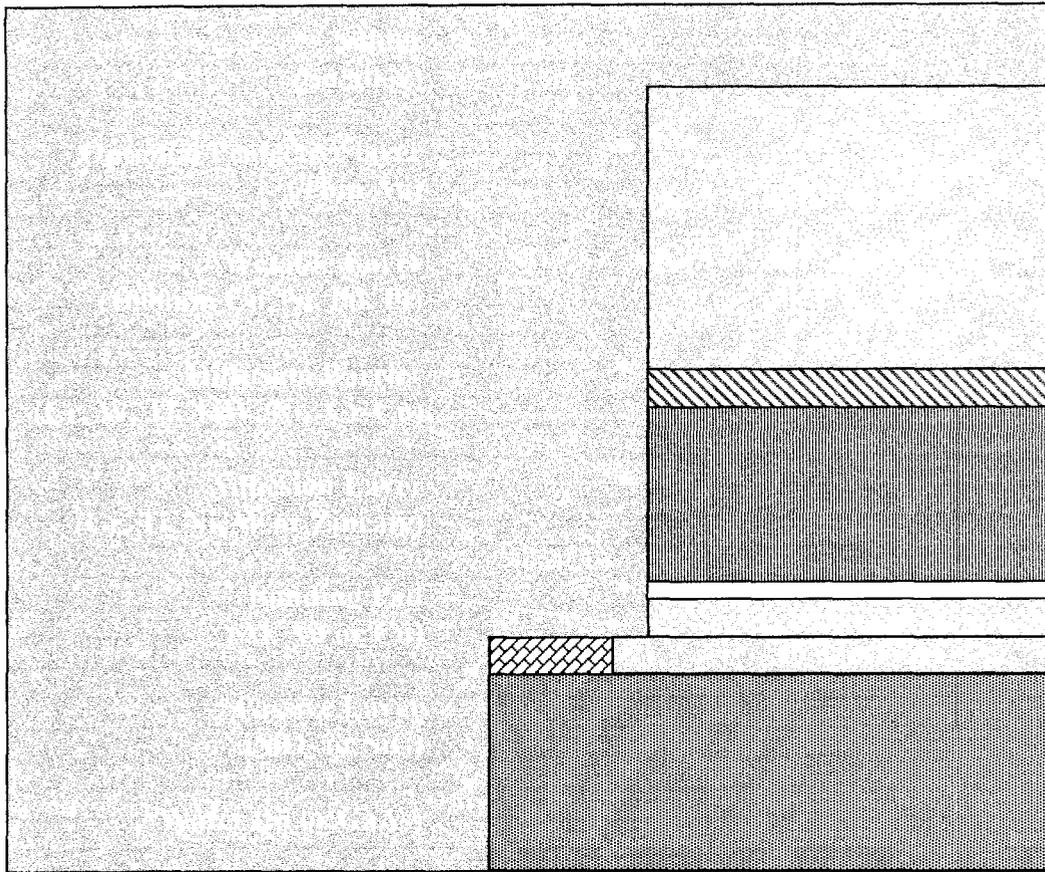
**Figure 2-1 – Anatomy of an IC bump. The drawing is based on descriptions in [Okikawa 1989] and [Baldwin & Higgins 2005].**
