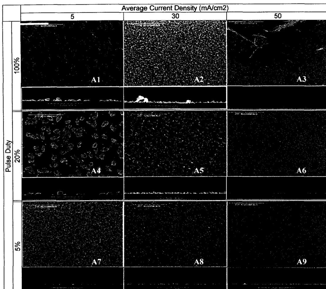
**Figure 5-4 – Plan views and cross sectional views of Sn-Cu films electrodeposited onto Au-coated Si. The plating bath was not agitated. Surface coverage, feature size and film roughness are all functions of pulse duty and average current density.**
