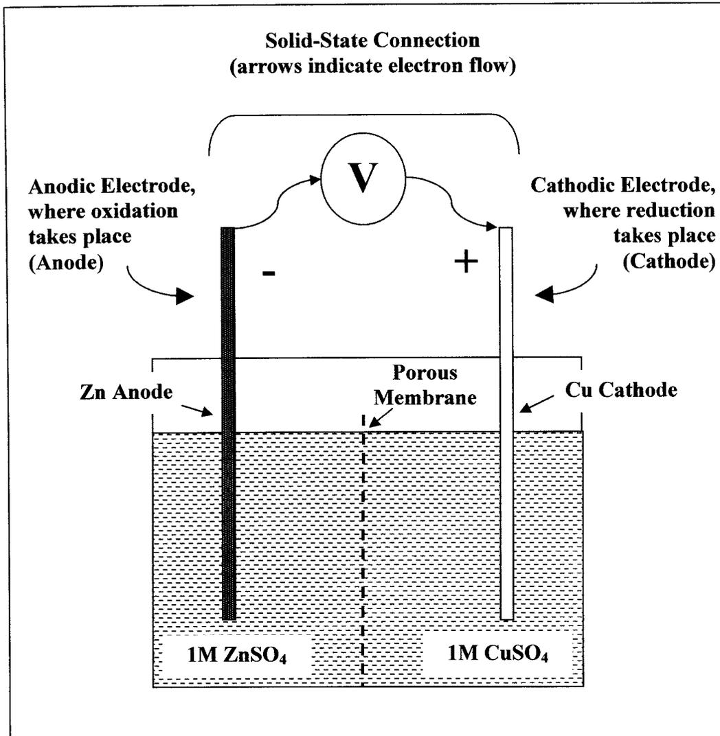
Figure 3-2 – A sample electrolytic cell at 25°C.
