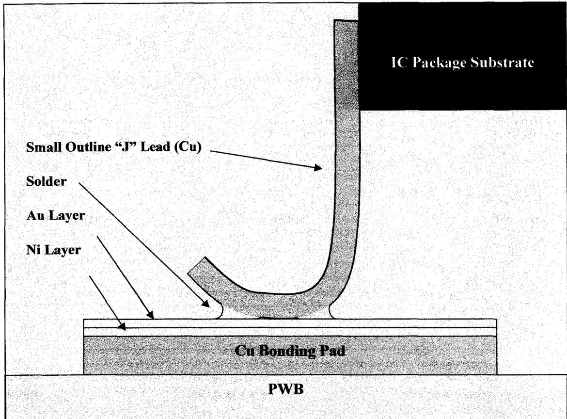
**Figure 2-5 – Drawing (not to scale) of the Cu small outline “J” lead soldered to a PWB finish as reported by Wu et al in Figure 1 of their work. Drawing by Olsen.**
