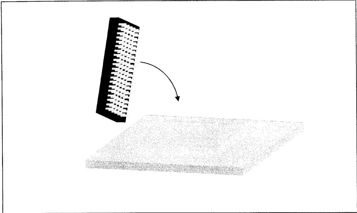
**Figure 1-10 – An IC package (black) can be bonded to a PWB by means of a Pin Grid Array (PGA). In this case, there is a socket that is surface mounted to the PWB. Based on Fig 15.7 from Mayer and Lau, 1990 and descriptions from Gileo.**
