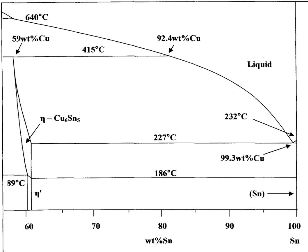
**Figure 4-1 – Sn-rich side of the Cu-Sn phase diagram, highlighting the liquid, ordered and disordered Cu<sub>6</sub>Sn<sub>5</sub> and pure Sn phase. Figure is redrawn from the full Sn-Cu binary after [Humpston & Jacobson 2004].**
