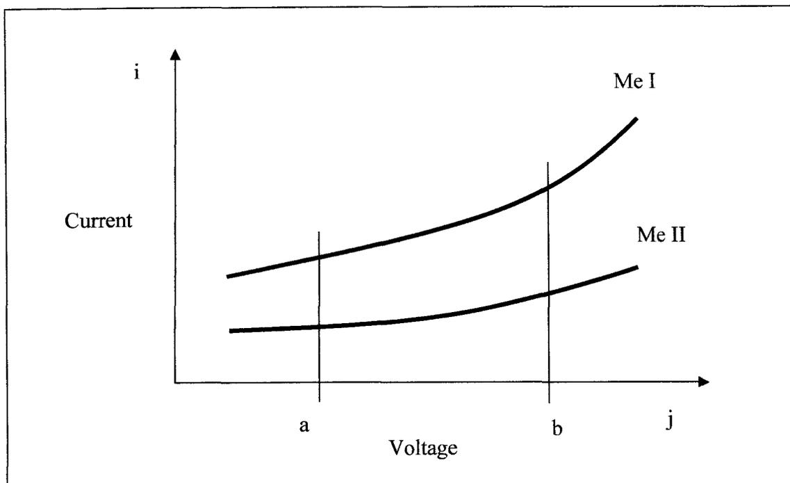
**Figure 3-9 – A current-voltage curve for two competing reduction reactions with different kinetics. Me I = Reaction 1, Me II = Reaction 2. (Redrawn from Puipe, p.7)**
