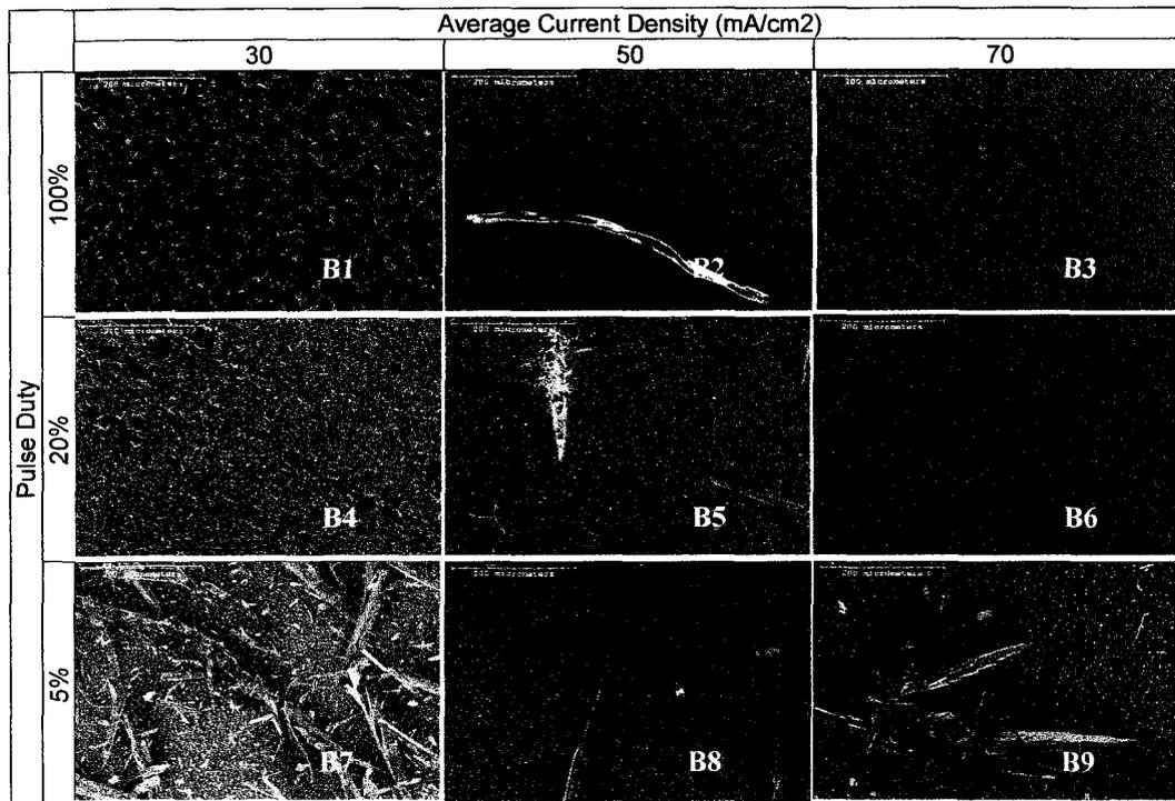
**Figure 5-5 – Composite of pure Sn films at various pulse duty and  $j_{avg}$  values. The scale bars are 200  $\mu$ m wide.**
