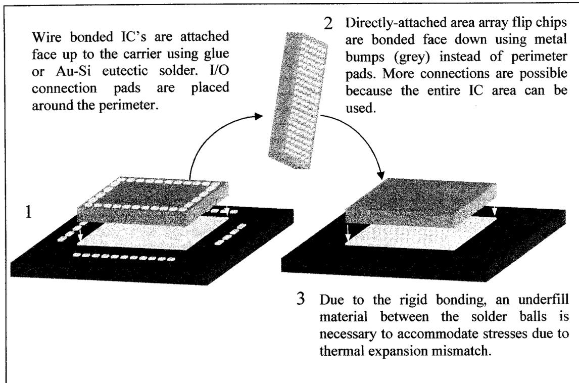
**Figure 1-6 - The active surface of the IC is “flipped” face down, as compared to the face up wire bonded configuration. The most important features of this Direct Chip Attach method is that the entire IC area chip can be used for connections to the carrier. Further, those connections are shorter than wires.**
