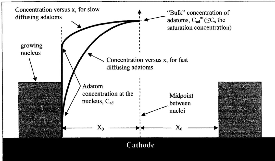
**Figure 3-10 – Diagram showing concentration profiles of fast- and slow-diffusing adatoms at various locations. This drawing is based on descriptions and Fig. 3.1 of [Puipe 1986-2].**
