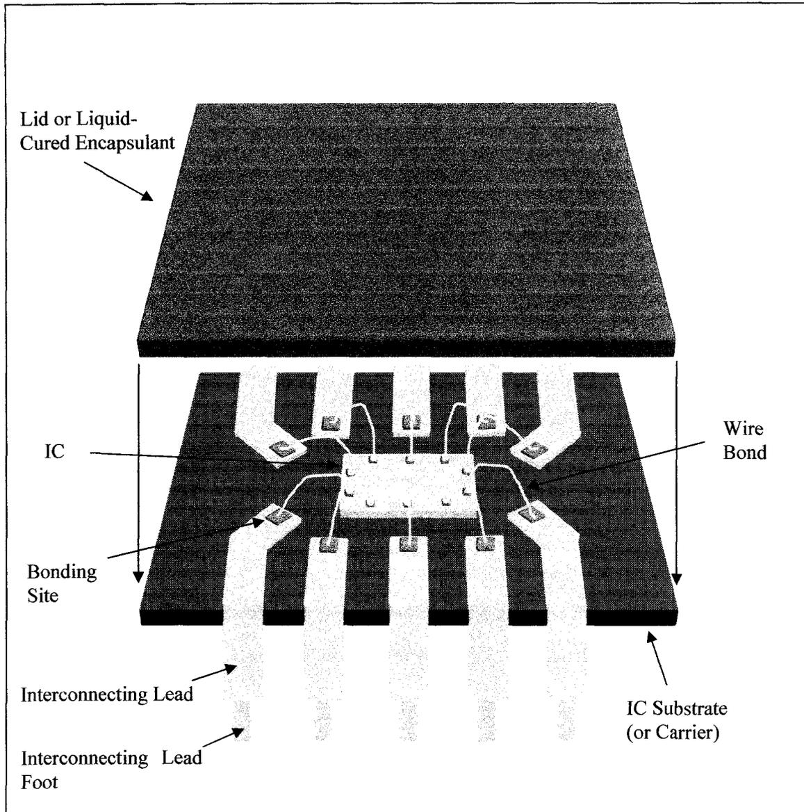
**Figure 1-1 – Cross-section of a wire-bonded chip mounted on a dual-in-line package, or DIP. This drawing is based on Figure 15.9 of Mayer and Lau 1990.**
