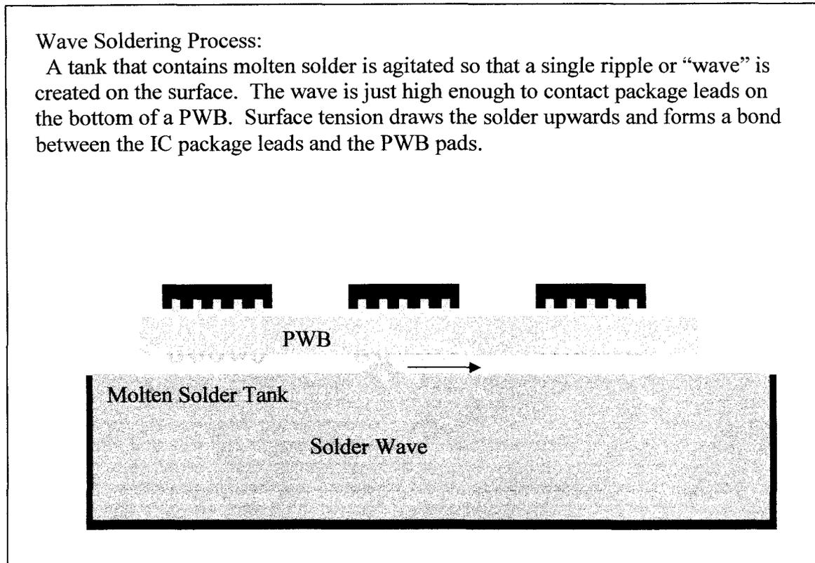
Figure 1-7 – Wave soldering process.
