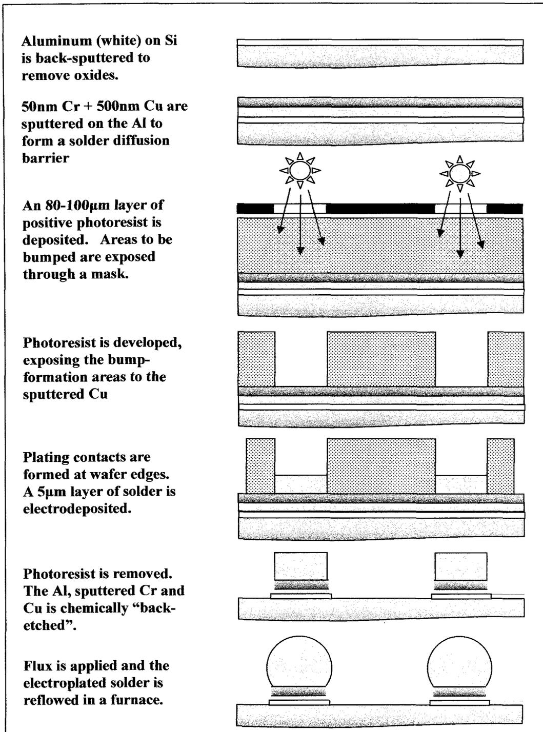
**Figure 4-2 – Method of Sn-Cu solder bump deposition on metallized Si IC's. Drawing is based on descriptions in [Karim & Schetty 2000].**
