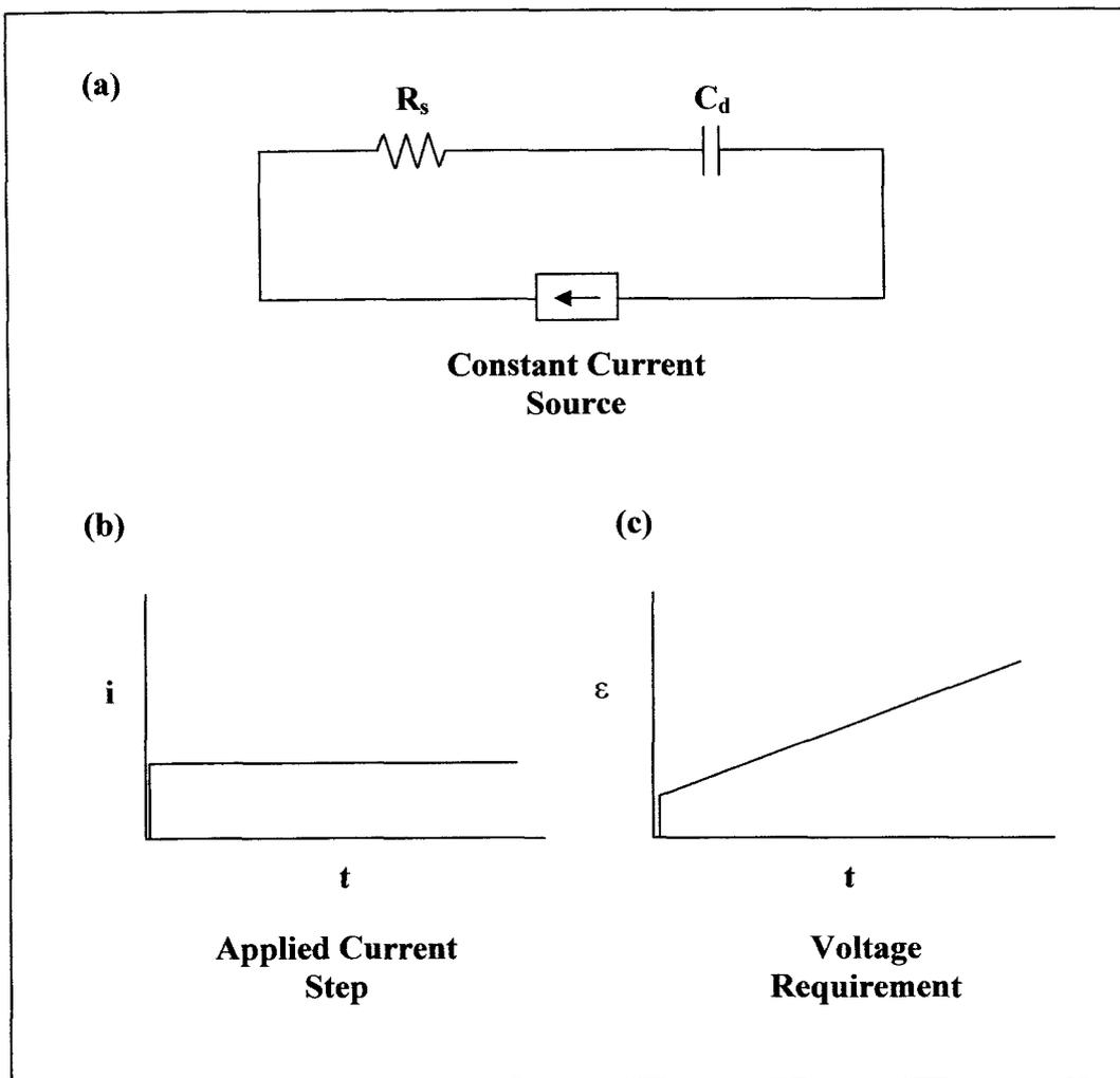
**Figure 3-5 – Characteristics of an electrochemical cell under constant applied current. Drawing based on Figures 1.2.8 and 1.2.9 of [Bard & Faulkner 2001].**
