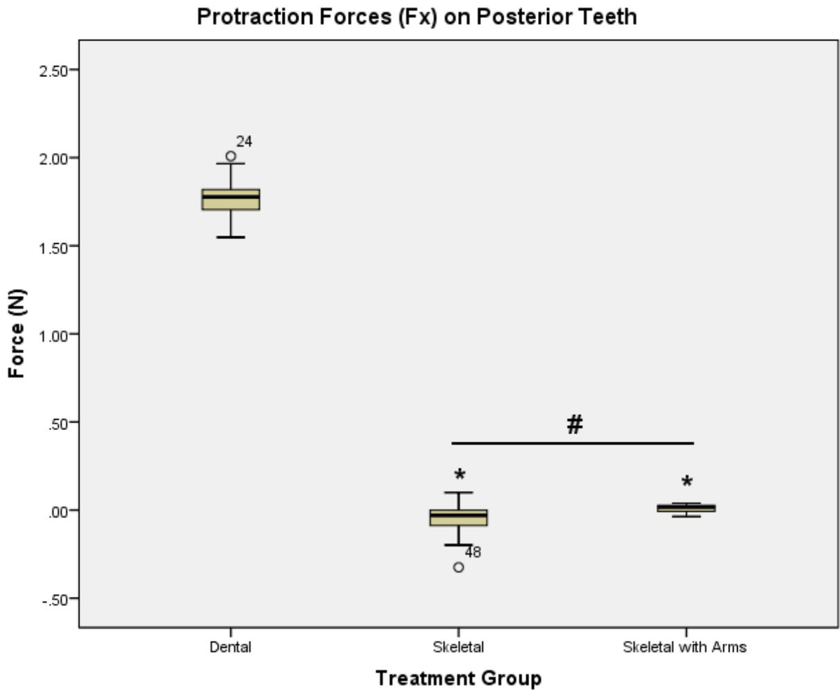
Figure 3.13. Comparison of protraction forces on the posterior teeth segment. (\*) denotes difference to 'Dental' group ( $p < 0.001$ ). (#)  $p < 0.001$ .
