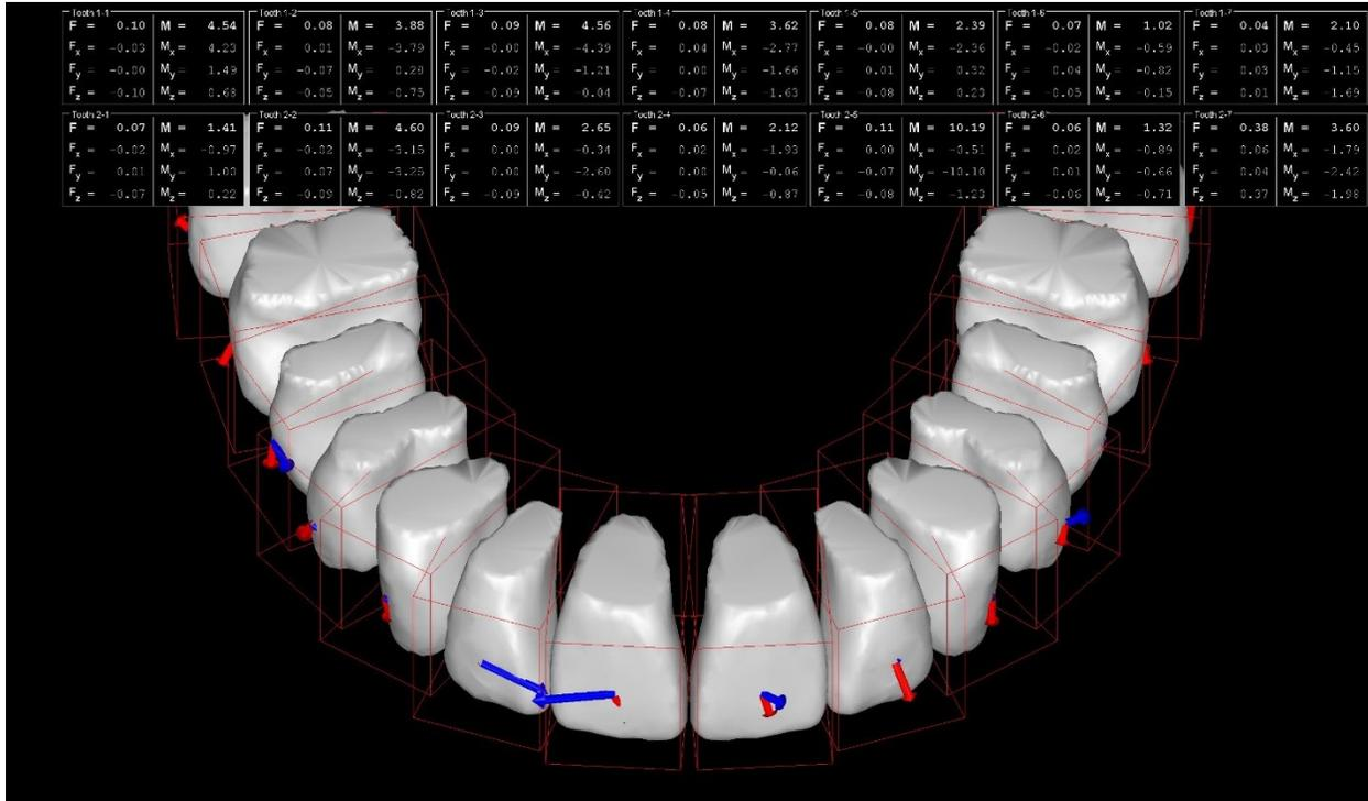
Control Group pre-test setup. Load cells kept to 0.10N or less.
