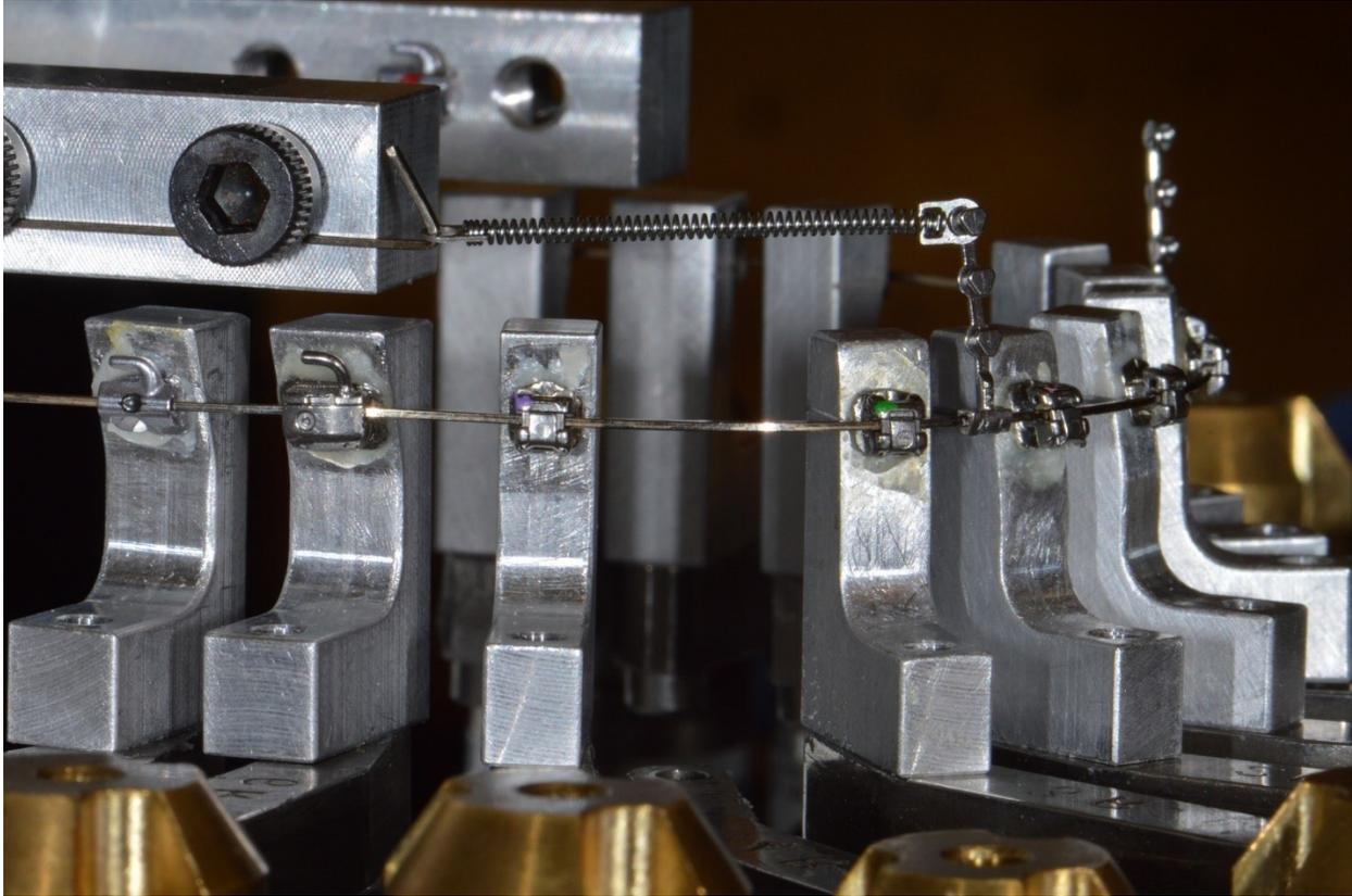
Figure 3.8. OSIM setup for skeletal retraction with power arms.
