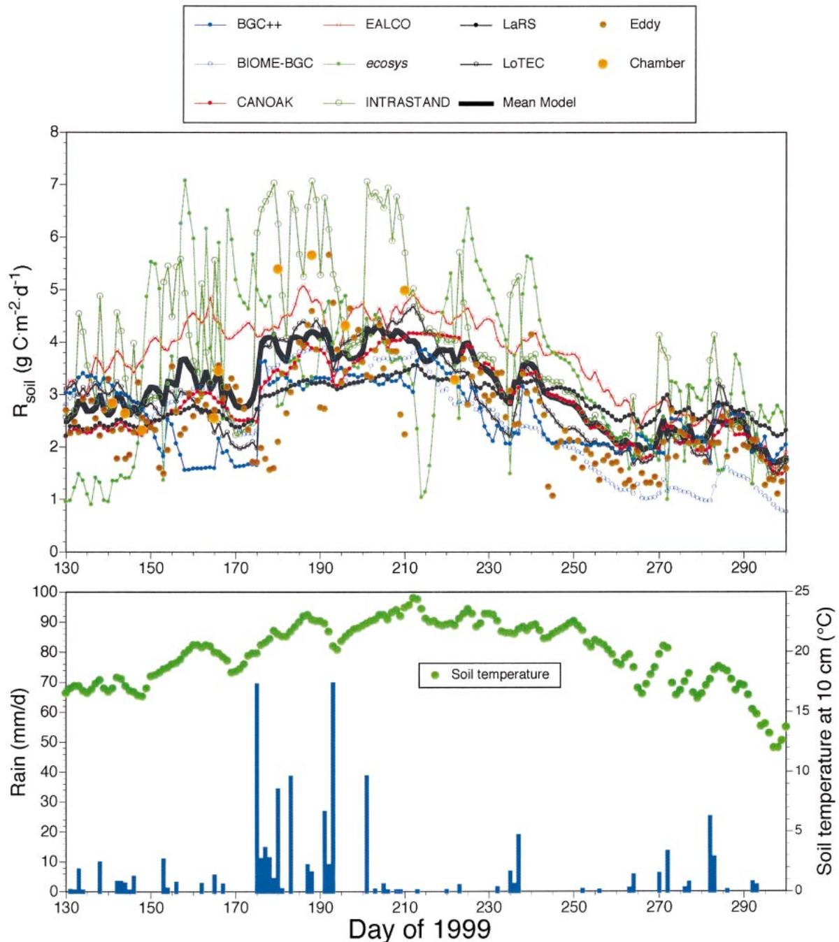
FIG. 14. Daily soil respiration ( $R_{soil}$ ) from chamber observations (Chamber), 1.5 m eddy covariance observations (Eddy), selected models, or the mean daily model response for the growing season of 1999.
