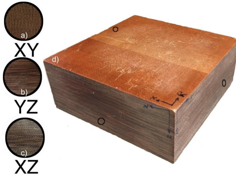
Figure 4.4. The texture of CE canvas fabric phenolic laminate with views along a) x -axis displaying warp and layering, b) y -axis displaying layering and weft, and c) z -axis displaying warp and weft. Arrows in each panel are 2 cm in length. d) Block of zero tilted ( \psi = 0^\circ ) Phenolic sample that is 5 cm * 12.5 cm * 12.5 cm.
