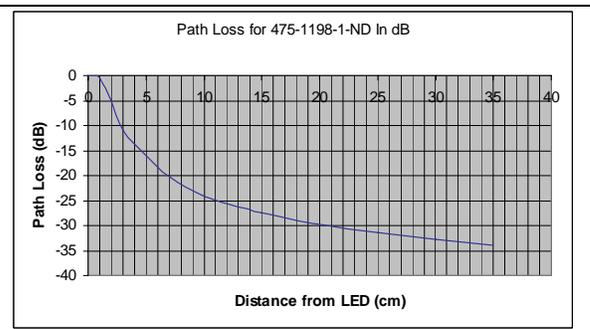
**Using the Power Measured at Ten Centimeters From the 475-1198-1-ND LED at Zero Degrees, This is a Plot of the Distance Required to Measure the Same Power Level at Angles around the LED**
