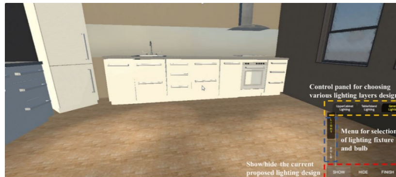
Figure 4-11 VR interface of lighting design
