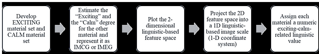
Figure 3-15 Procedures for material linguistic-based image scale construction
