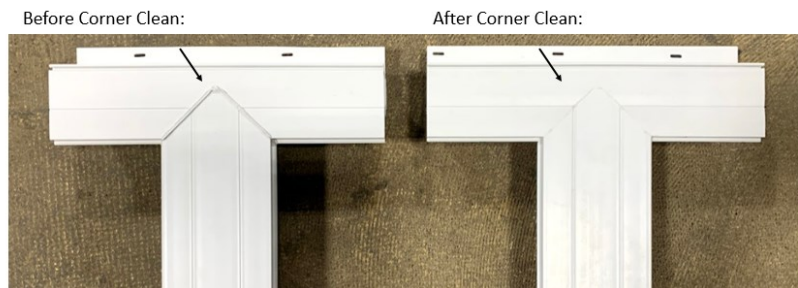
Figure 3-11: Comparison between Before and After Corner Clean
