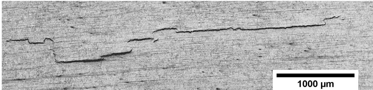
Figure E.1: Optical micrograph of a HIC crack observed in a section cut at 90° from High Mo steel.
