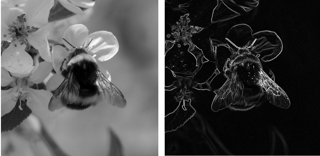
Figure 1.2: A grey-scale image (originally 1024 \times 1024 pixels) transformed with the Sobel operator. Any pixel intensity greater than 255 is set to 255.
