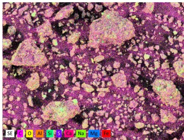
**Figure 3-3** Secondary Electron SE image from Mancal's Coal elemental distribution in SEM-EDS (Map/Spectrum)
