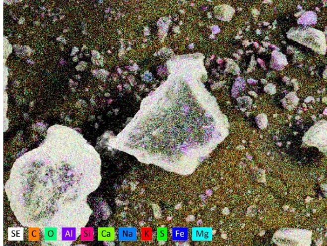
**Figure 6-1** Secondary Electron SE image from Mancal's Coal elemental distribution in SEM-EDS (Map/Spectrum) for feed to OCD with changes on temperature at 1 MPa.
