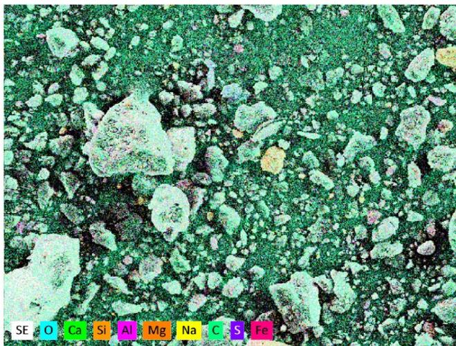
**Figure 5-1** Secondary Electron SE image from Mancal's Coal elemental distribution in SEM-EDS (Map/Spectrum) for feed to OCD with changes on temperature at 5 MPa.
