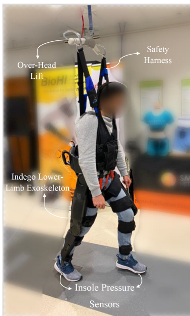
Fig. 4: Experimental set-up: Indego lower-limb exoskeleton in a user study (having a safety harness) during over-ground walking
