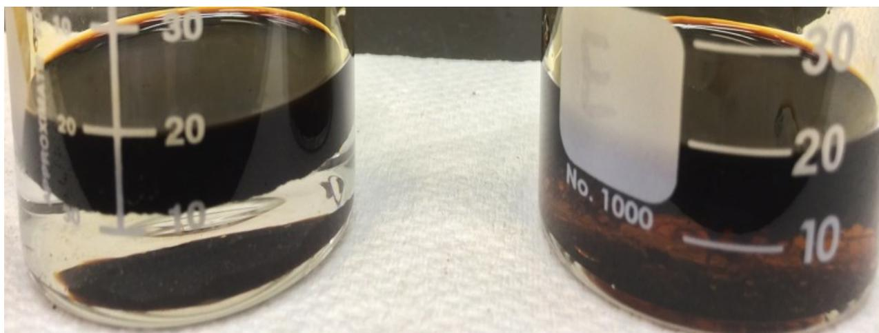
**Figure 5.11 - Emulsion test. Left: bitumen in toluene/distilled water; Right: bitumen in toluene/polymer A solution.**
