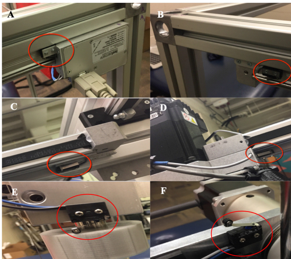
Figure 2-6. Mechanical limit switches: A) X-axis head, B) X-axis feet, C) Y-axis left, D. Y-axis right, E) Z-axis bottom, F) Z-axis top
