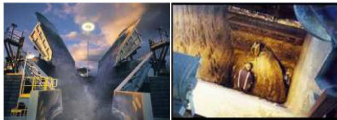
Figure 1.2: (a) Two haul trucks empty their load of oil sand into the top of a double roll crusher [3] and (b) People are employed to remove large lump in crusher caused jam event.
