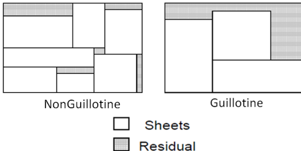
Figure 3.36: NonGuillotine and Guillotine cutting pattern (Manrique et al. 2011).
