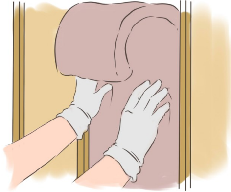
Figure 3.5: Insulation installation between two studs (“Basement Wall Insulation Blanket - Viewing Gallery” 2014).
