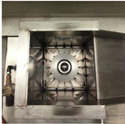
Figure 3-2: View of the batch flotation cell from the top
