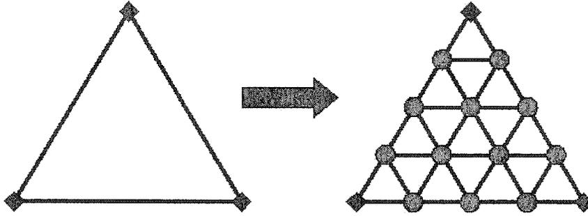
Figure 3.1: The interpolatory 4-adic subdivision scheme for the triangular mesh. By adding 3 new vertices on an edge and 3 new vertices for each face, one edge is split into 4 new edges and one face is split into 16 new faces. “ $\diamond$ ” denotes the old vertices and “ $\circ$ ” denotes the new inserted vertices.
