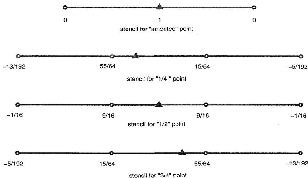
Figure 2.4: Associated subdivision stencils for the best interpolatory 4-adic subdivision scheme. By the symbol “ $\triangle$ ” we denote the new inserted vertex, and the symbol “ $\circ$ ” denotes vertices at the previous level.
