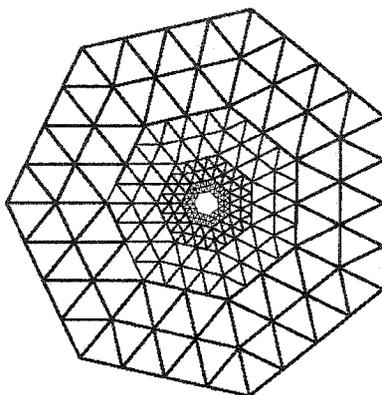
Figure 4.2: The  $k$ -gon without origin extraordinary vertex can be decomposed into similar rings. Taking dyadic subdivision schemes into account, each two times smaller than the previous ring. The size of the ring is chosen in such a way that the control set of any ring does not contain the extraordinary vertex. In this figure the control set is assumed to consist of the vertices of the triangles of the ring itself, and of a single layer of vertices outside the ring.
