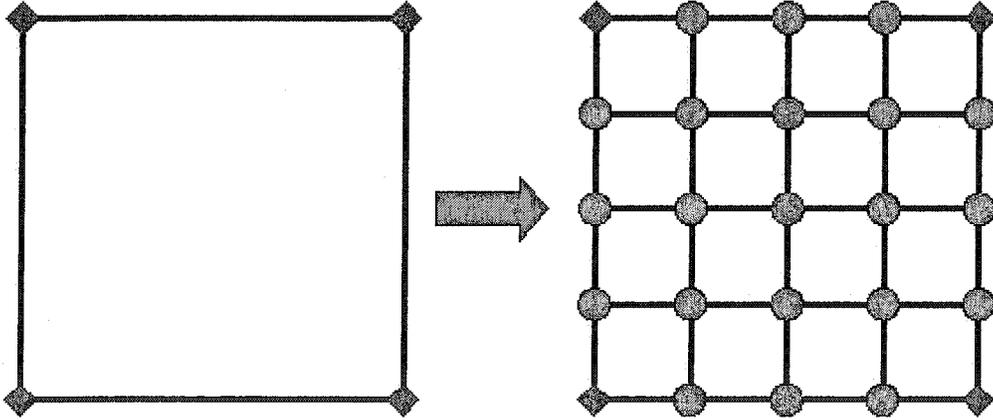
Figure 3.11: The interpolatory 4-adic subdivision scheme for the quadrilateral mesh. By adding 3 new vertices on an edge and 4 new vertices for each face, one edge is split into 4 new edges and one face is split into 16 new faces. “ $\diamond$ ” denotes the old vertices and “ $\circ$ ” denotes the new inserted vertices.
