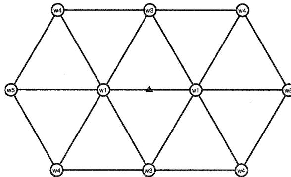
Figure 3.6: Associated subdivision stencil for “1/2 vertex” on an edge.
