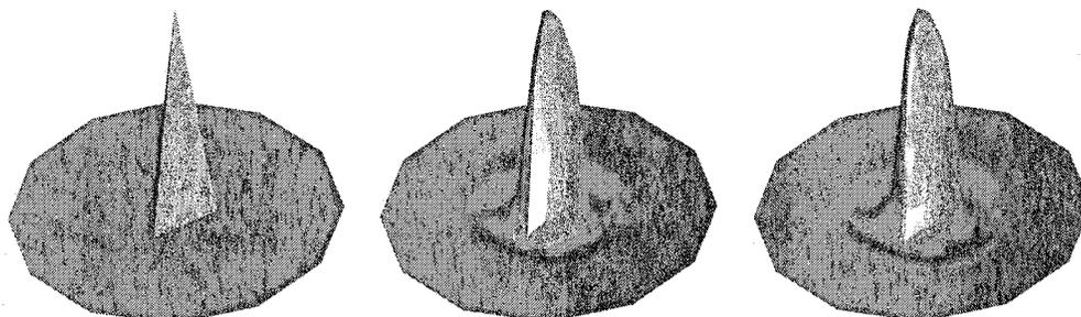
Figure 4.16: Applying the special interpolatory 4-adic subdivision scheme on an example mesh with an unique extraordinary vertex ( $k = 3$ ). From left to right are the initial, first level and second level subdivision surfaces, respectively.
