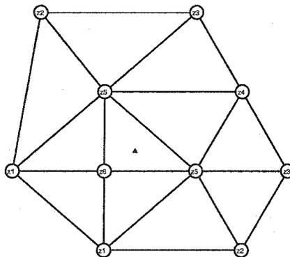
Figure 4.10: The stencil for a new inserted interior vertex inside a face which contains a  $k = 4$  extraordinary vertex.
