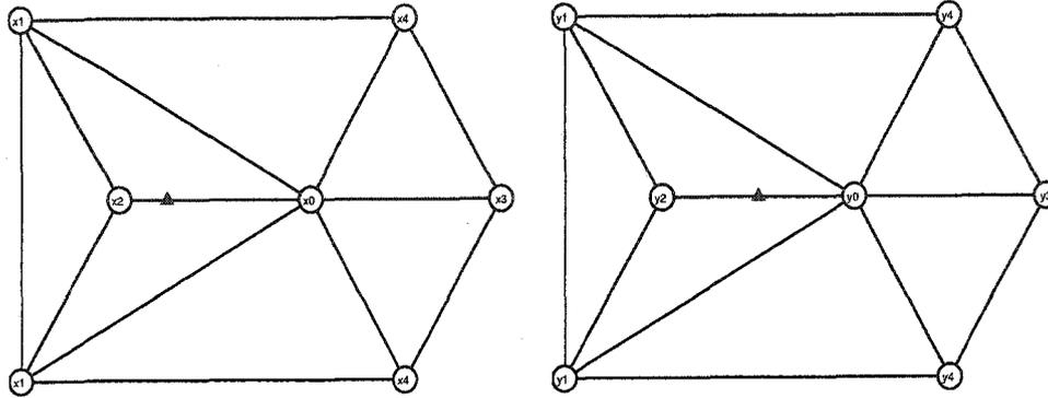
Figure 4.13: The stencil for a new inserted “1/4 vertex” and “1/2 vertex” on an edge associated with a  $k = 4$  extraordinary vertex.
