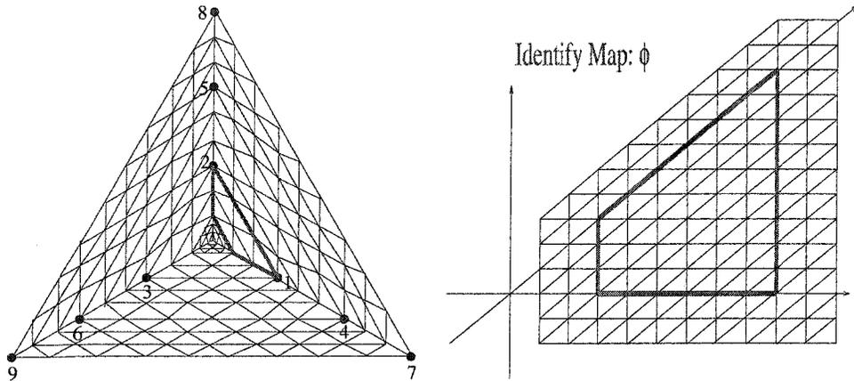
Figure 4.7: Identify a section around extraordinary vertex with a sector in the regular triangular mesh. All the vertices inside this bold area can be computed by the vertices within two rings outside this bold area.
