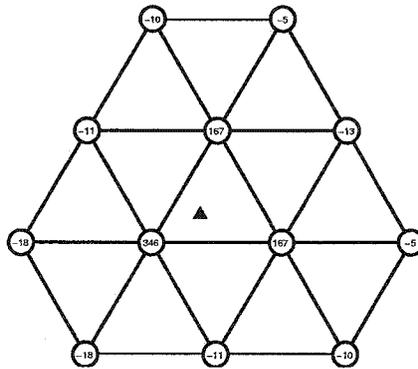
Figure 3.3: The interpolatory subdivision stencil for new inserted *interior* vertex inside a face, with  $t_1 = 10/3$ ,  $t_2 = 0$ ,  $t_3 = -5/3$  and  $t_4 = 0$ . All the numbers in the above stencil should be divided by 576.
