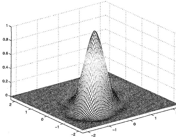
Figure 3.8: The graph of the basis function  $\phi$  for the subdivision triplet in the Theorem 3.1 with  $t_1 = 10/3$ ,  $t_2 = 0$ ,  $t_3 = -5/3$  and  $t_4 = 0$ .
