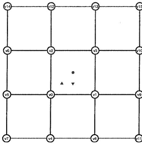
Figure 3.13: Associated subdivision stencils for new inserted interior vertices inside a face. The upper triangle symbol denotes the “ $(1/4, 1/4)$  vertex”, down triangle symbol denotes the “ $(1/2, 1/4)$  vertex” and small circle symbol denotes the “ $(1/2, 1/2)$  vertex”.
