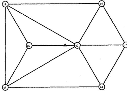
Figure 4.14: The stencil for a new inserted “3/4 vertex” on an edge associated with a  $k = 3$  extraordinary vertex.
