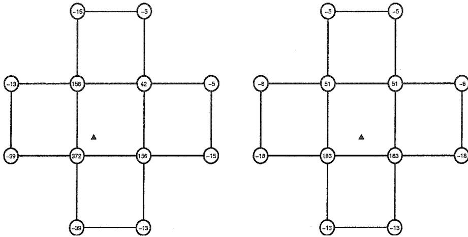
Figure 3.17: Associated subdivision stencils for new inserted vertices interior of a face at the “(1/4, 1/4) vertex” and at “(1/2, 1/4) vertex”. All the weights are divided by 768.
