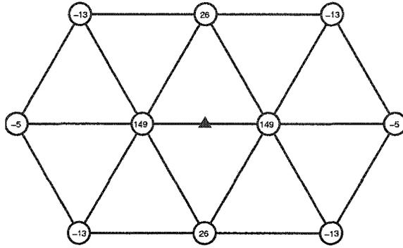
Figure 3.7: The interpolatory subdivision stencil for “1/2 vertex” on an edge, with  $t_1 = 10/3$ ,  $t_2 = 0$ ,  $t_3 = -5/3$  and  $t_4 = 0$ . All the numbers in the above stencil should be divided by 288.
