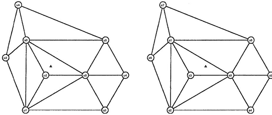
Figure 4.15: The stencil at left is for a new inserted interior “(1/4,1/4)” vertex, and at right is for a new inserted interior “(1/2, 1/4)” vertex inside a face which contains a  $k = 3$  extraordinary vertex.
