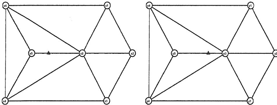
Figure 4.5: The stencil at left is for a new inserted “1/3 vertex”, and at right is for a new inserted “2/3 vertex” on an edge associated with a  $k = 3$  extraordinary vertex.
