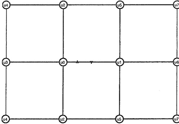
Figure 3.12: Associated subdivision stencils for new inserted vertices on an edge. Up triangle denote the “1/4 vertex” and down triangle denotes the “1/2 vertex”.
