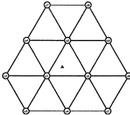
Figure 3.2: Associated subdivision stencils for the best two-dimensional interpolatory 4-adic subdivision scheme for the interior new inserted vertex. By the symbol “ $\triangle$ ” we denote the new inserted vertex, and the symbol “ $\circ$ ” denotes vertex of the previous level, the numbers inside the circles, which are named  $u_1, u_2, \dots, u_7$ , are the weights of the corresponding vertices.
