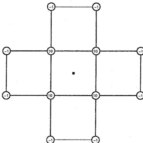
Figure 3.16: Associated subdivision stencils for new inserted vertices interior of a face at the “(1/2, 1/2) vertex”. All the numbers in the above stencils should be divided by 32.
