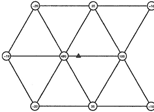
Figure 3.5: The interpolatory subdivision stencil for “1/4 vertex” on an edge, with  $t_1 = 10/3$ ,  $t_2 = 0$ ,  $t_3 = -5/3$  and  $t_4 = 0$ . All the numbers in the above stencil should be divided by 576.
