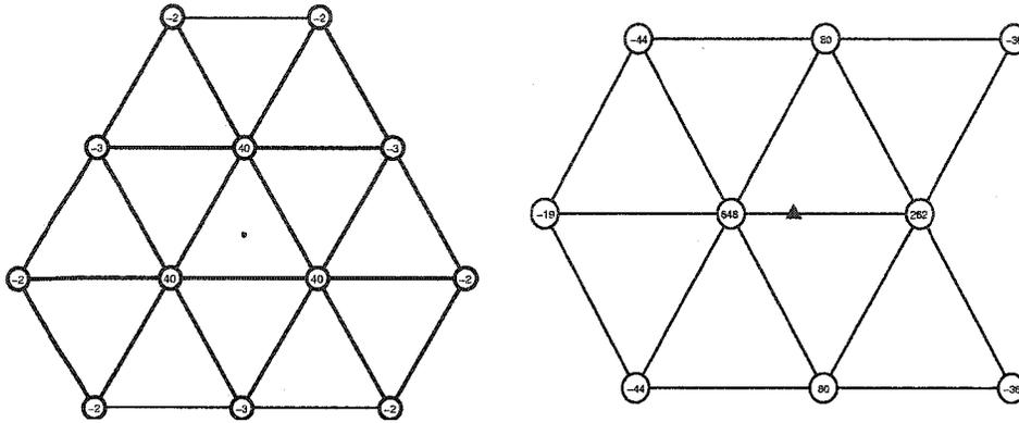
Figure 4.3: The stencils of the ternary subdivision schemes for regular meshes. The numbers at left shall be divided by 99; the numbers at right shall be divided by 891 [19].
