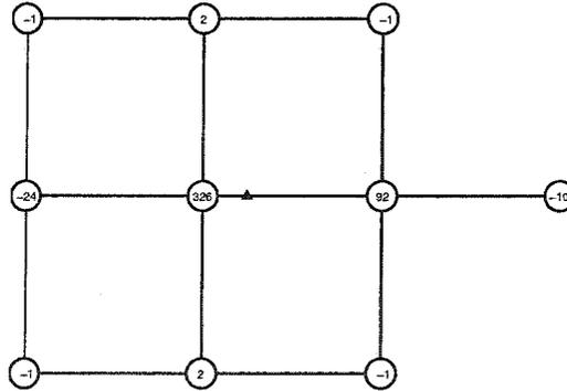
Figure 3.14: Associated subdivision stencils for new inserted vertices on an edge at the “1/4 vertex”. All the numbers in the above stencil should be divided by 384.
