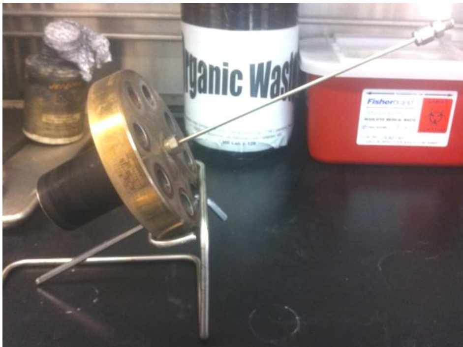
Figure 11. Designated structure to protect the bellows cap.
