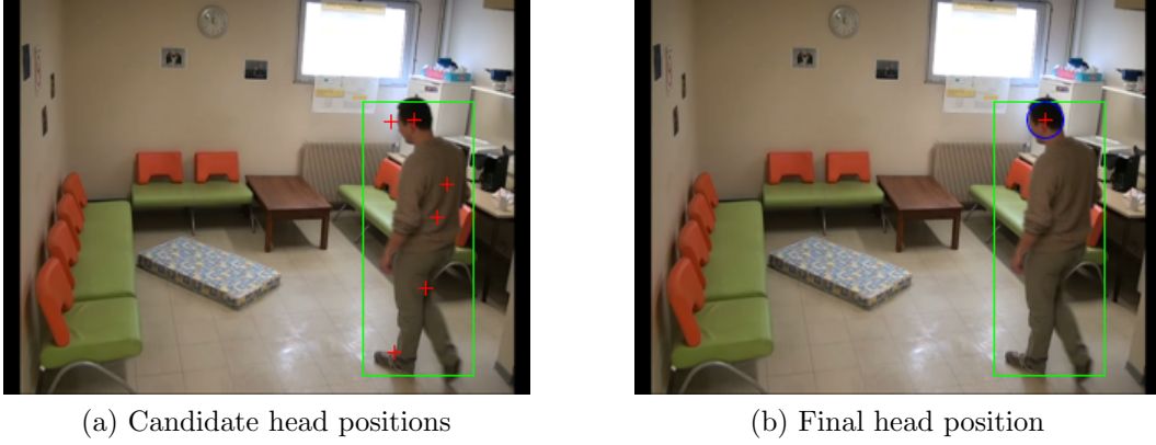
Figure 3.6: The steps and result of the head detection approach.
