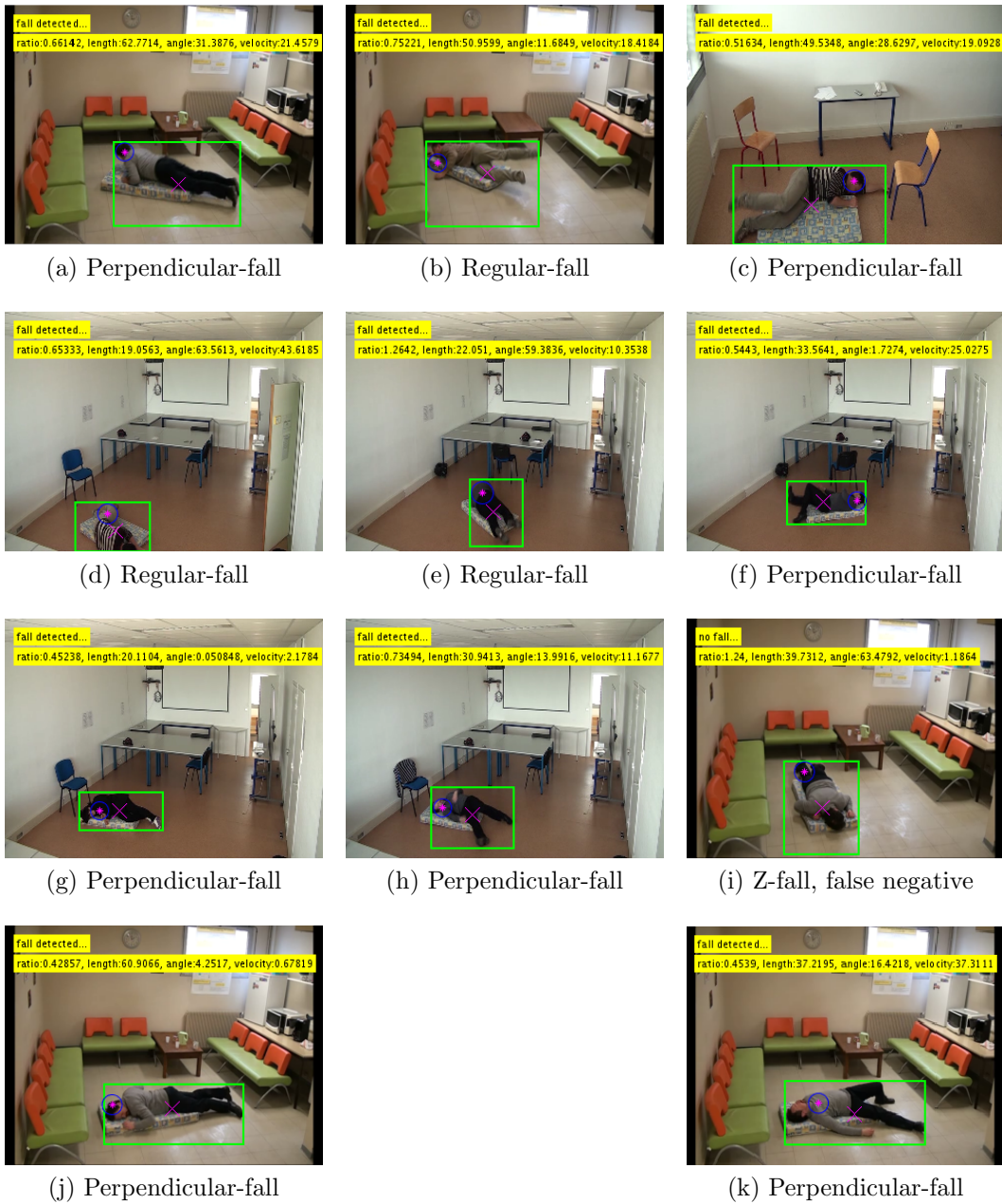
Figure 3.9: The result of proposed detection system on fall actions.
