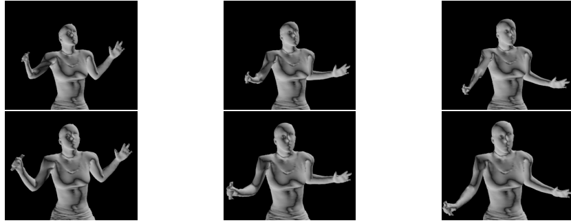
Figure 5.13: Top row: frames from animation using skeleton without optimization. Bottom row: corresponding frames using skeleton optimized by our algorithm. Note that the right arm does not look warped in the bottom row.
