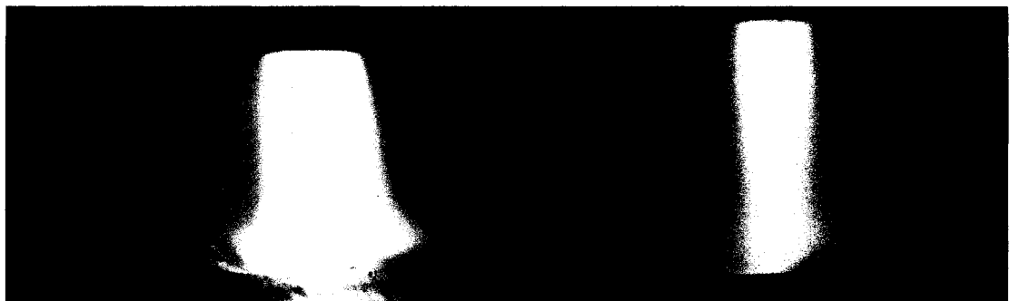
Figure 44 – Arc Images of Secondary Arc (left) and Reverse Metal Transfer (right)
