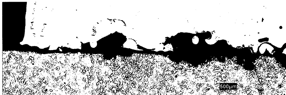
Figure 88 – 410SS Argon-Helium Plasma Gas (P9.1): Overlay Tie-in Flaws
