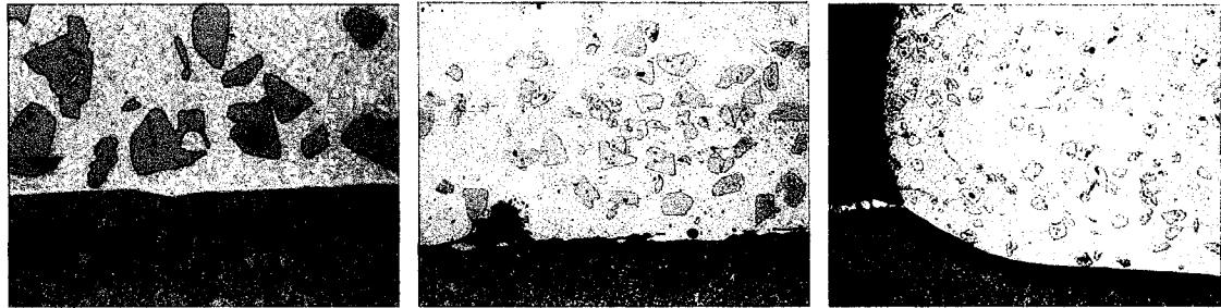
Figure 96 – Micrographs of Good Interface Fusion with Composite Region (Left, Sample W1, 300X), Variable Interface Fusion (Center, Sample W6, 100X), & Excellent Tie-In Fusion (Right, Sample W4, 50X)
