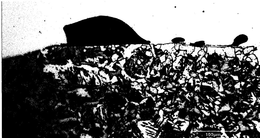
Figure 87 – 410SS Argon Standard (P8.2): Interface Porosity and Cracking at Overlay Center
