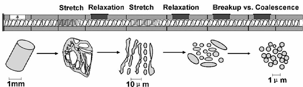
**Figure 2-6** The flow fields in extruder and the evolution of the dispersed phase down the length of the extruder.
