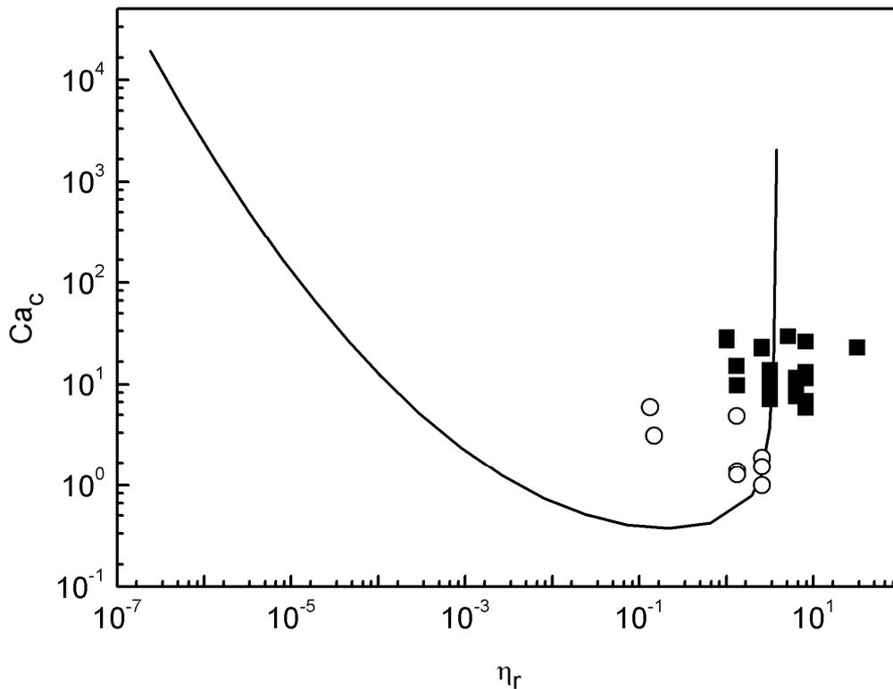
**Figure 4-11** The relationship between  $Ca_c$  and  $\eta_r$  for viscoelastic drop breakup. The dashed line is the correlation for Newtonian drop breakup adapted from de Bruijn [35]. Solid squares are for vorticity breakup and empty circles are for breakup in the flow direction.
