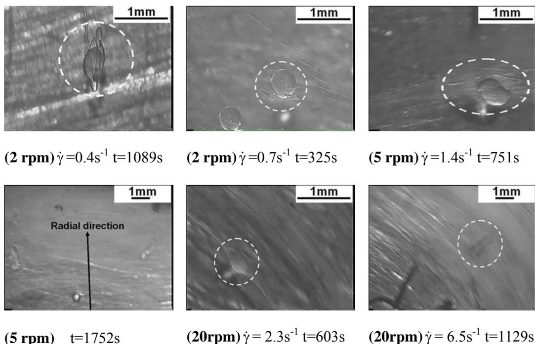
**Figure 5-7** PS drops are sheared in PE matrix while the rotation rate is increased stepwise by 1 rpm/min. The shear rates shown in the figure are the shear rate for the drops in white circles.
