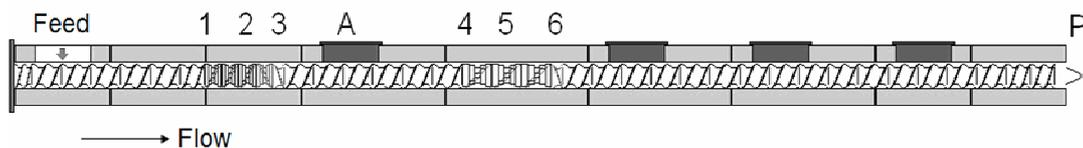
**Figure 2-4** Schematic of sampling locations along Berstorff ZE25A UTX Ultragliding co-rotating twin screw extruder.
