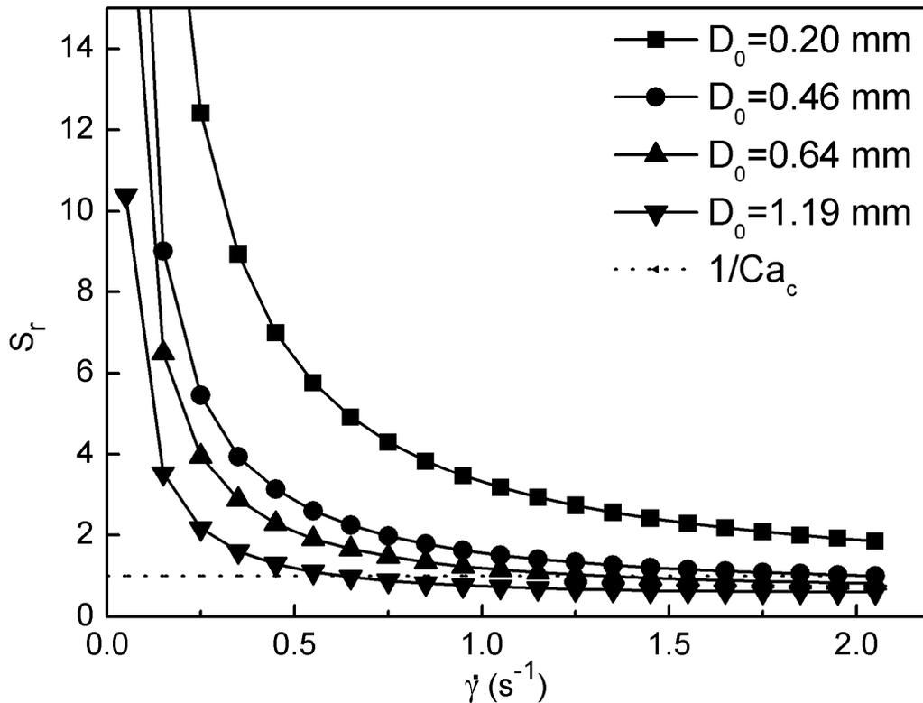
**Figure 4-9** Dependence of stress ratio on shear rate for different drop sizes for system M3/D3.
