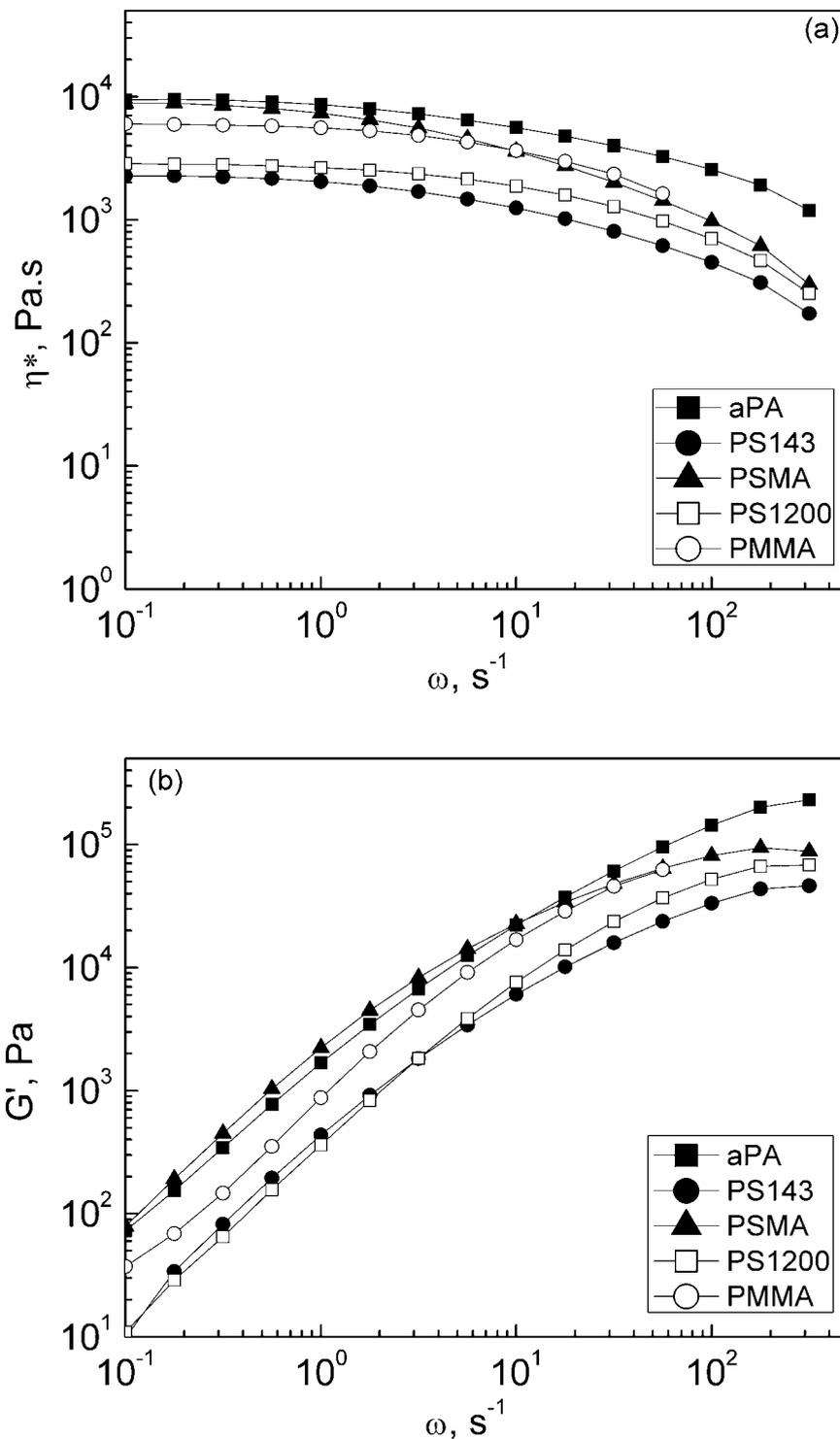
**Figure 2-3** Rheological properties of polymers at 220°C. (a) Complex viscosity; (b) Elastic modulus.
