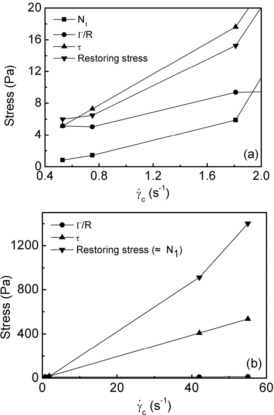
**Figure 4-10** Drop size effect on the stresses at breakup, M3/D3. (a) Stresses at low shear rates; (b) Stresses in the whole range of shear rate in this study.
