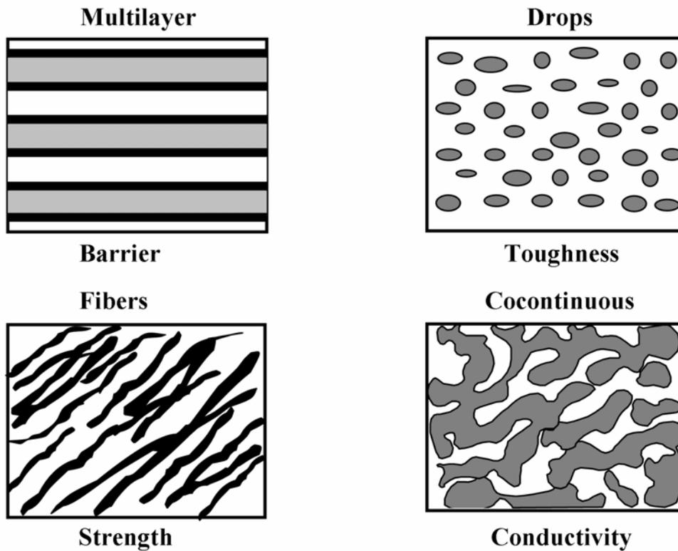
**Figure 2-1** Polymer blend morphologies and their characteristic properties. Adapted from [2, 31].
