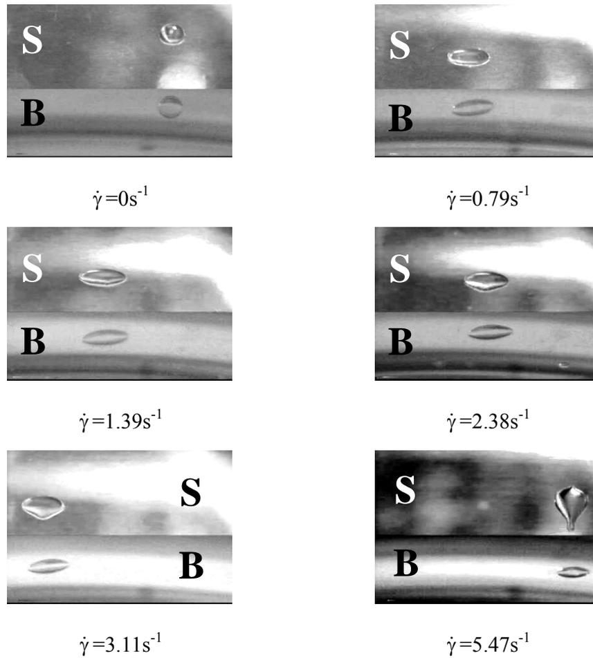
**Figure 3-6** Vorticity direction deformation of system M3/D4,  $\eta_r = 3.2$ ,  $D_0=0.88\text{mm}$ .
