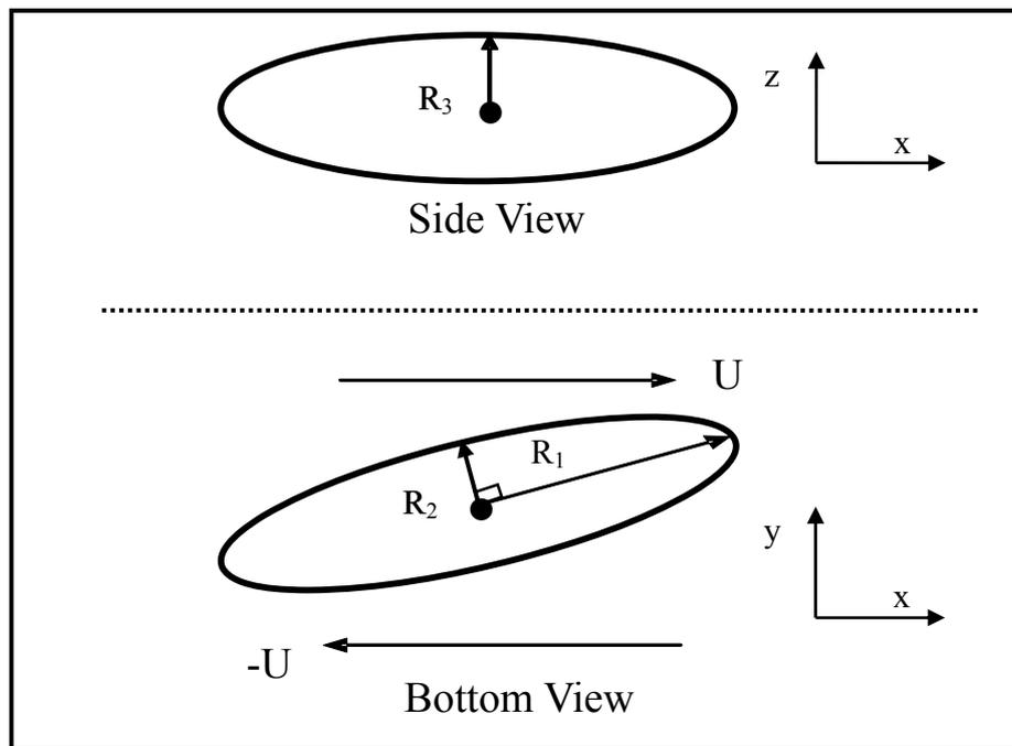
**Figure 3-3** A schematic of a drop subjected to simple shear flow. • is the drop center;  $U$  is the velocity at the cylinder wall.
