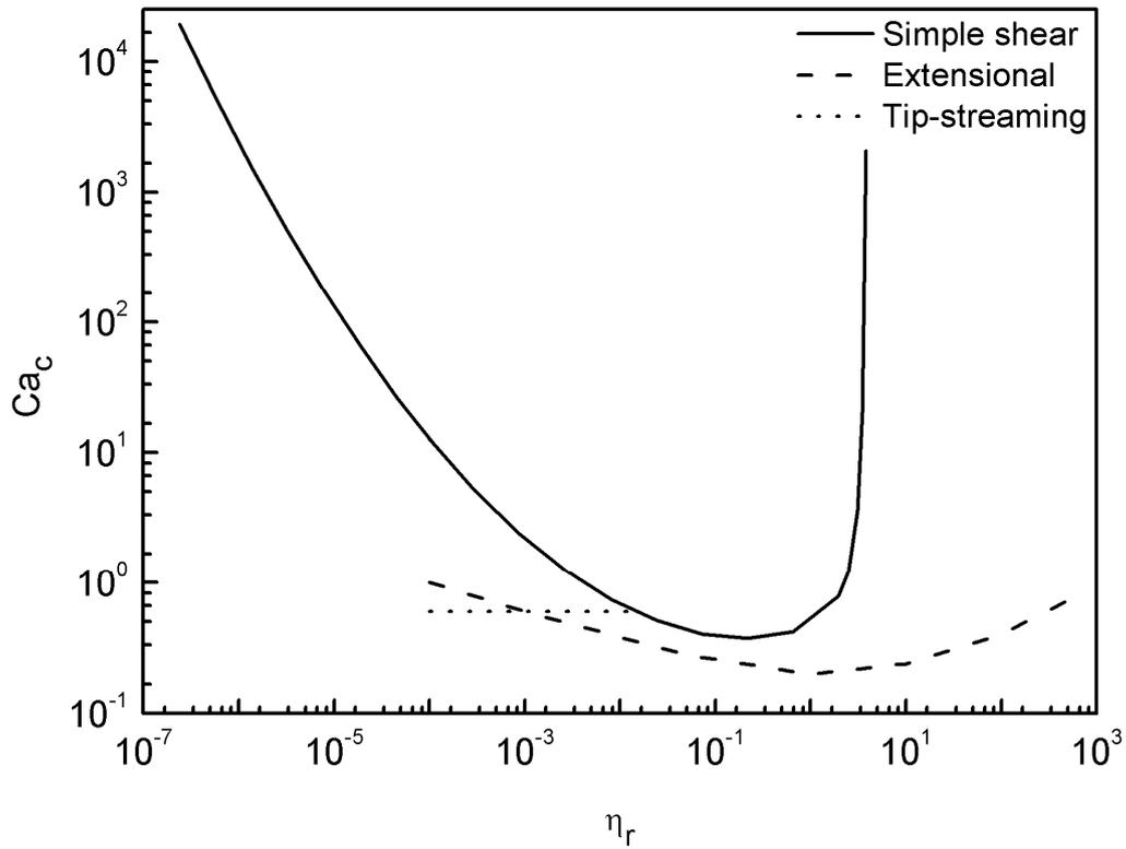
**Figure 4-1** Critical capillary number versus viscosity ratio for Newtonian drop breakup (adapted from Grace[4]).
