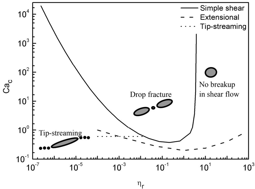
**Figure 1-5** Correlation of critical capillary number and viscosity ratio for Newtonian drop breakup. Adapted from [34].
