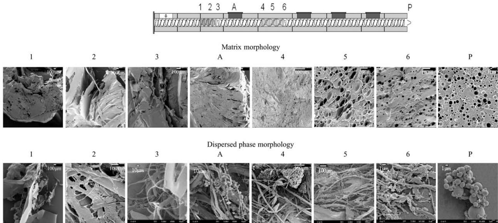
**Figure 2-5** Morphology development of uncompatibilized system PS143/aPA (20 wt% aPA ) at 220°C, rotation rate of 400 rpm and a feed rate of 25 kg/hr in Berstorff twin screw extruder. (Note different scale bars).
