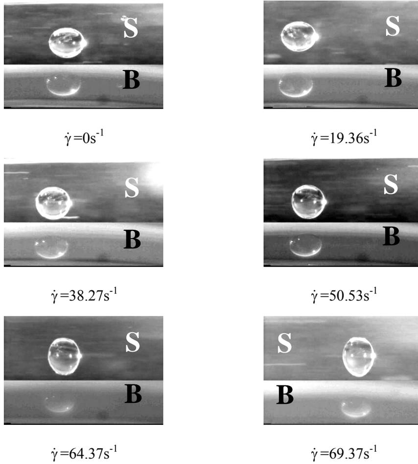
**Figure 3-8** Vorticity direction deformation of system M1/D4,  $\eta_r = 32$ ,  $D_0=1.6\text{mm}$ .
