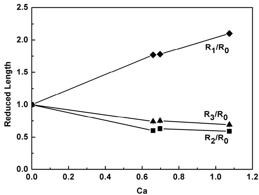
**Figure 3-5** Reduced radii of M3/D3,  $\eta_f=2.6$ ,  $D_0=1.16\text{mm}$ . Error bars are within data points.
