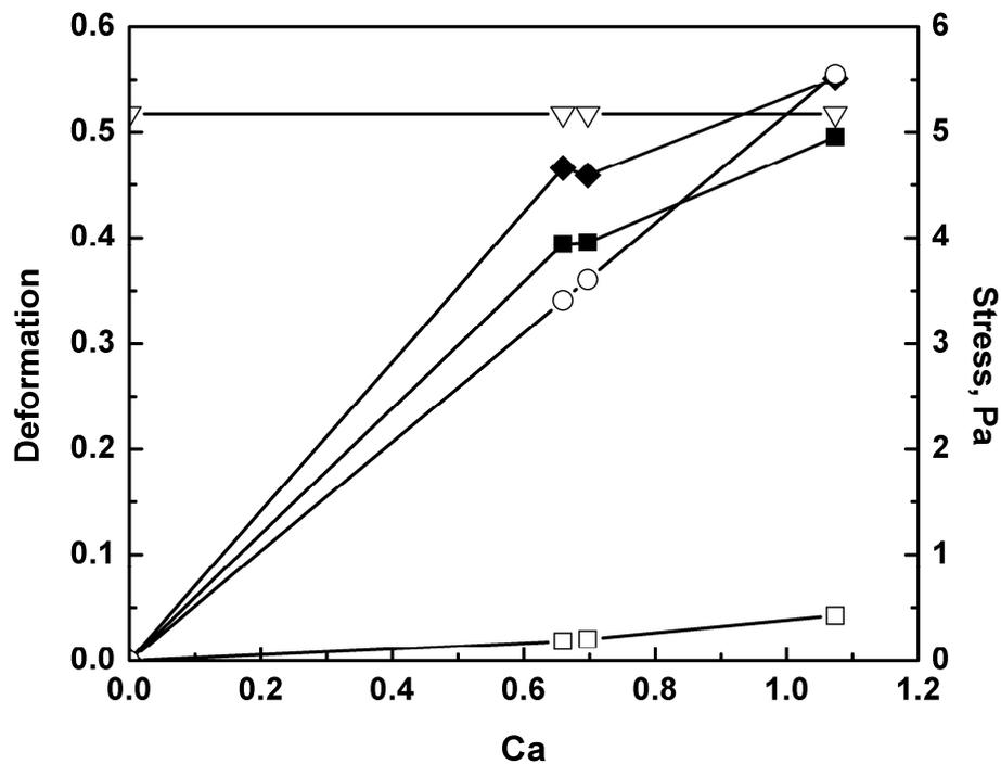
**Figure 3-10** Development of stresses and deformations with increasing capillary number, M3/D3,  $\eta_r = 2.6$ ,  $D_0=1.16\text{mm}$ . Solid symbols are deformations:  $Df_1$  (■),  $Df_2$  (◆); and unfilled symbols are stresses:  $\Gamma/R_0$  (▽),  $\tau$  (○),  $N_1$  (□).
