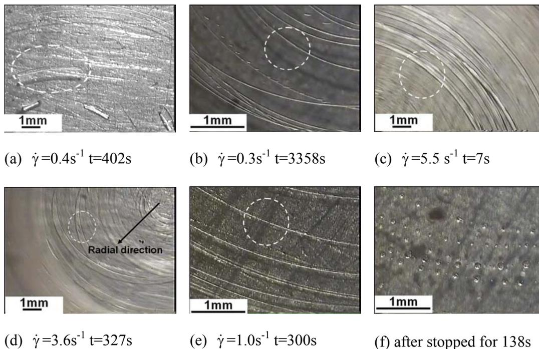
**Figure 5-9** PC1050 drops are sheared in PE matrix at different shear rates. (a) and (b): the rotation rate is 2 rpm by start-up mode. (c) and (d): the rotation rate is 20 rpm by start-up mode. (e): the rotation rate is increased to 5 rpm stepwise by 1 rpm/min. (f): after (e) stopped for 138s, the fibers break up into spheres. The shear rates shown in the figure are the shear rate for the drops in white circles.
