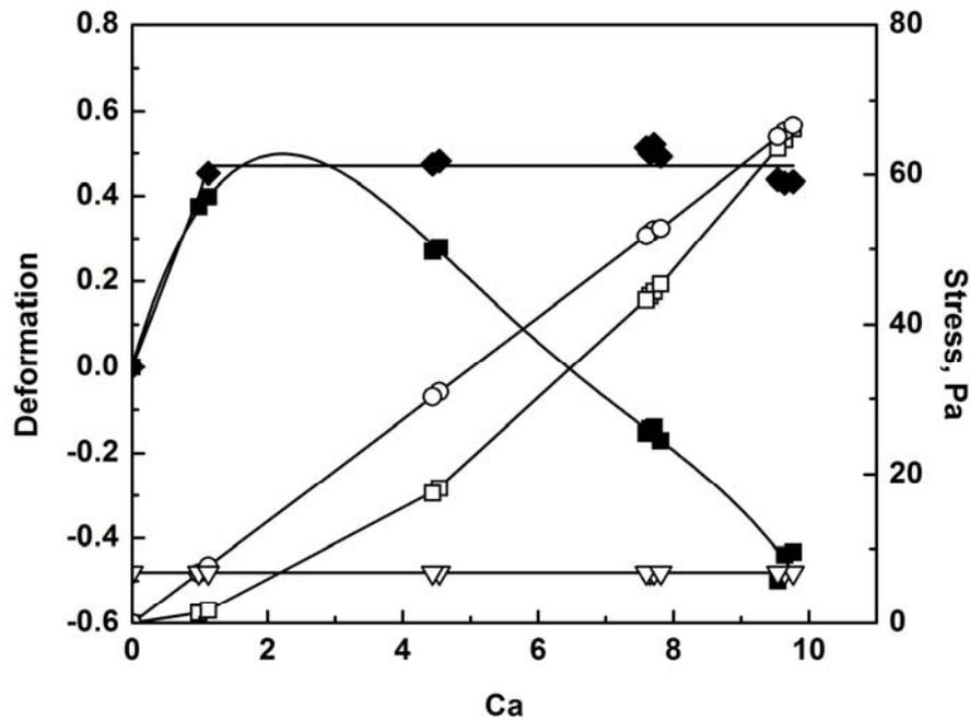
**Figure 3-11** Development of stresses and deformations with increasing capillary number,  $M3/D4$ ,  $\eta_r = 3.2$ ,  $D_0 = 0.88$  mm. Solid symbols are deformations:  $Df_1$  (■),  $Df_2$  (◆); and unfilled symbols are stresses:  $\Gamma/R_0$  (▽),  $\tau$  (○),  $N_1$  (□).
