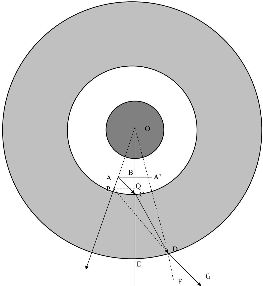
**Figure II-1** Cross section of the Couette device. The shaded areas denote the inner cylinder and the outer cylinder respectively. Figure not drawn to scale.
