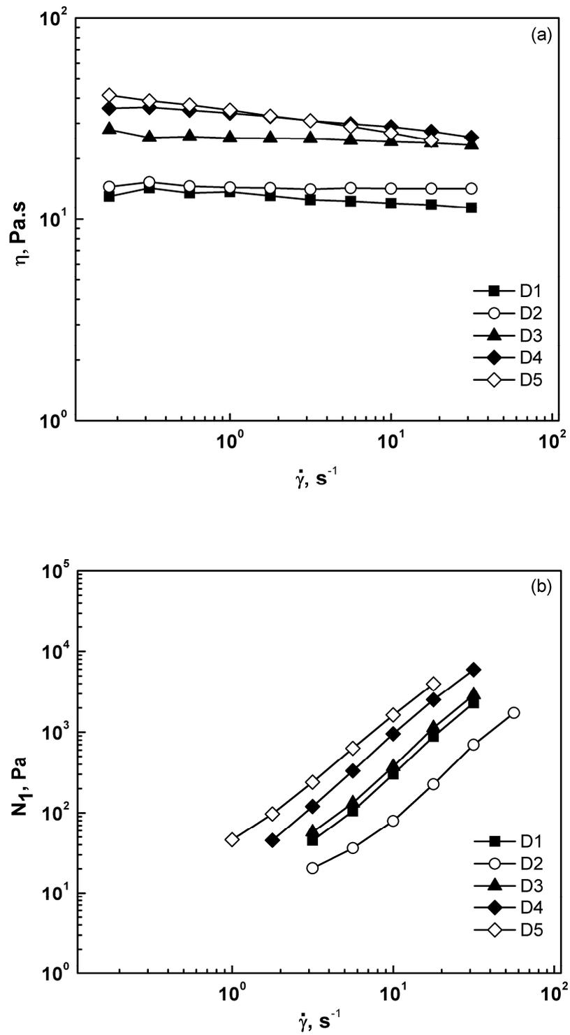
**Figure 4-3** Steady rheology properties of Boger fluids. (a) Viscosity of Boger fluids. (b) First normal stress difference of Boger fluid.
