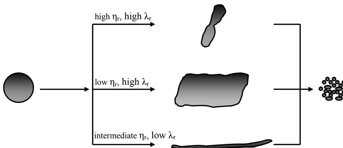
**Figure 5-12** Morphology development mechanism during blending.
