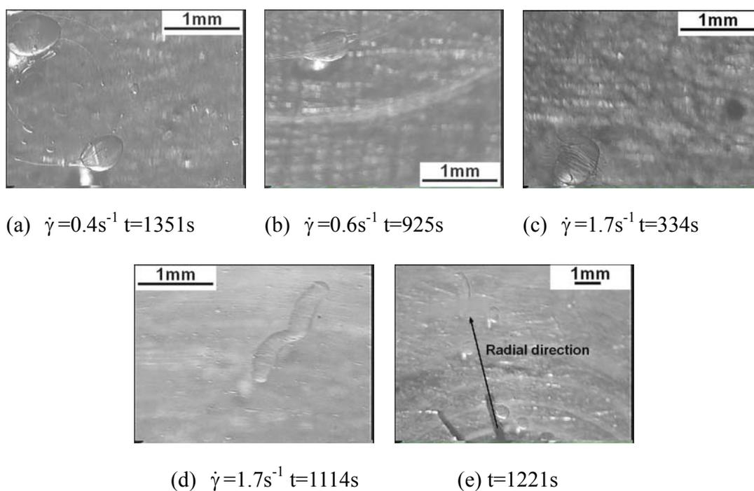
**Figure 5-5** PE/PS sheared at a rotation rate of 5rpm of the master rotor. (a) and (b): threads developed at the drop ends. (c): threads developed at the drop surface. (d): drop elongates in the vorticity direction. (e): drops elongates in the high shear rate zones. The shear rates are shown below each micrograph.
