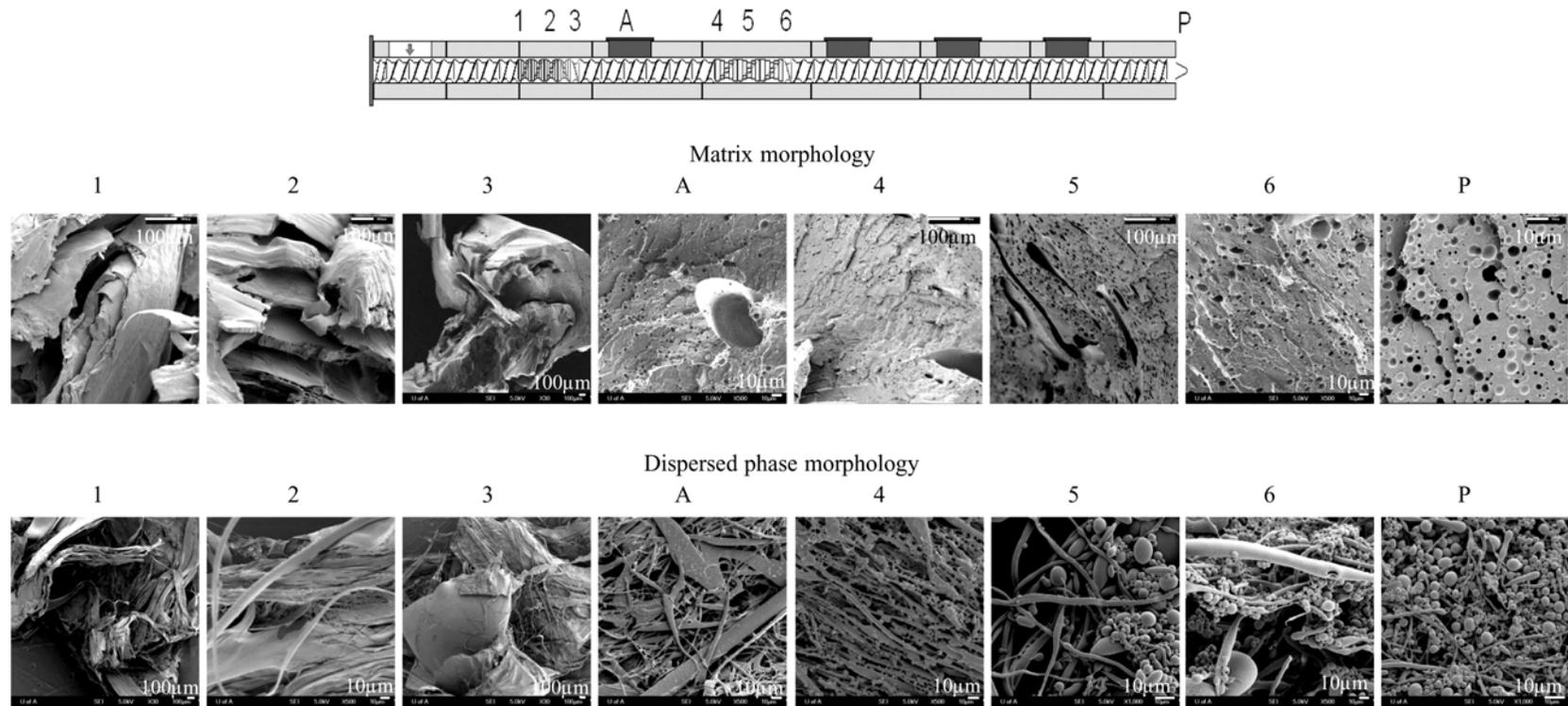
**Figure 2-8** Morphology development of uncompatibilized system PS143/aPA (20 wt% aPA ) at 220°C, rotation rate of 1000 rpm and a feed rate of 62.5 kg/hr in Berstorff twin screw extruder. (Note different scale bars).
