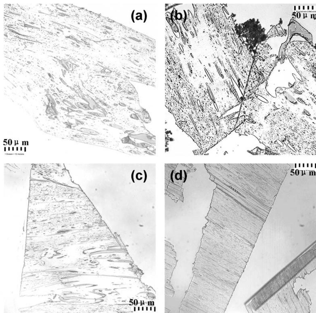
**Figure 2-12** Optical photomicrographs of PMMA/aPA and PSMA/aPA obtained from internal batch mixer at 220°C and 20 rpm after mixing for 20 seconds and 40 seconds. (a) PMMA/aPA, 20 seconds, 20rpm. (b) PMMA/aPA, 40 seconds, 20rpm. (c) PSMA/aPA, 20 seconds, 20rpm. (d) PSMA/aPA, 40 seconds, 20rpm.
