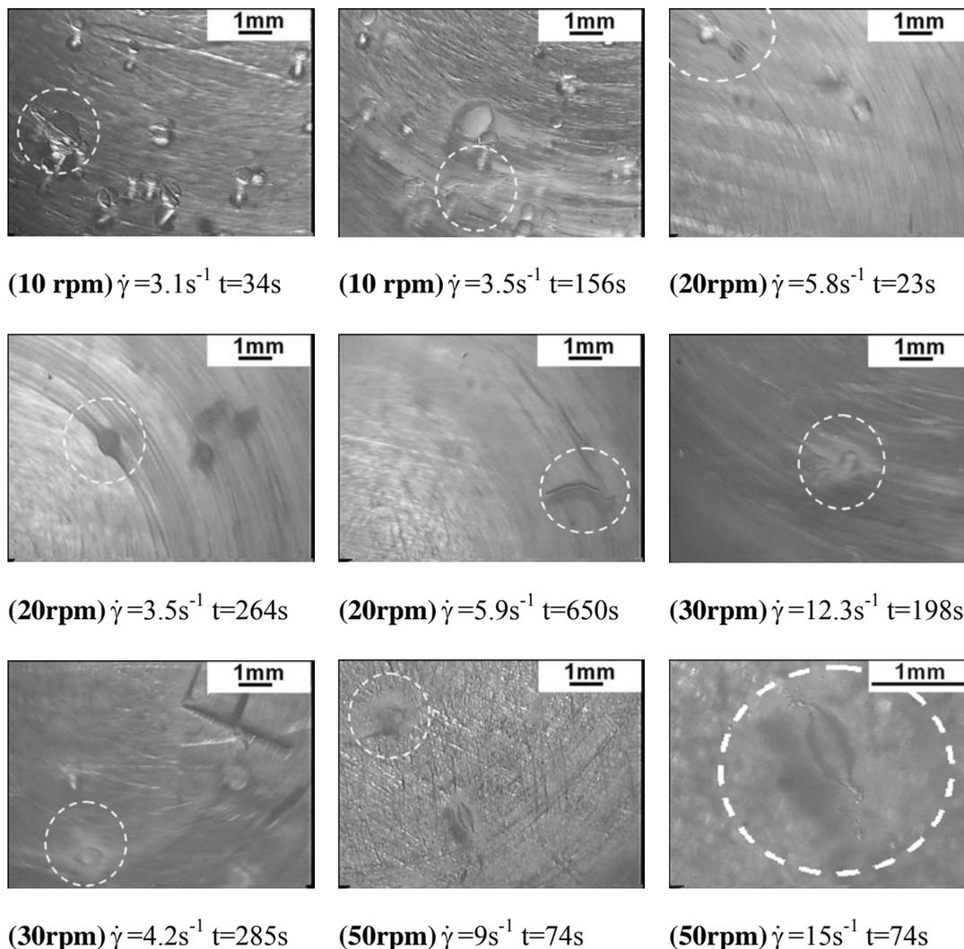
**Figure 5-6** PE/PS sheared at a rotation rate of 10 to 50 rpm of the master rotor. The shear rates shown in the figure are the shear rate for the drops in white circles.
