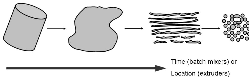
**Figure 1-2** Schematic of morphology development during blending.
