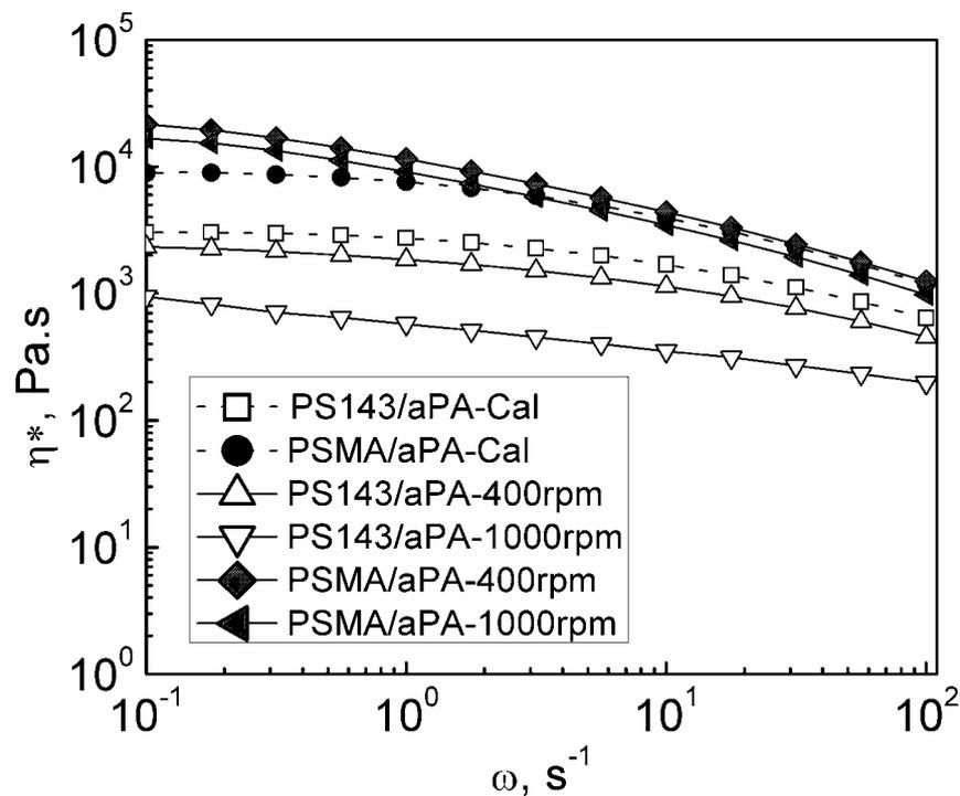
**Figure 2-10** Viscosities of polymer blends obtained from location P of the extruder. Open symbols are uncompatibilized systems and closed symbols are compatibilized systems. Solid lines are measured viscosities for polymer blends obtained from location P of the extruder. Dashed lines (PS143/aPA-Cal and PSMA/aPA-Cal) denote predicted viscosities based on log-additive mixing rule (Eqn 2.3).
