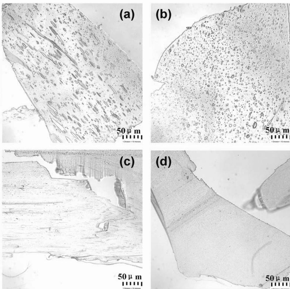
**Figure 2-11** Optical photomicrographs of PS1200/aPA and PSMA/aPA obtained from internal batch mixer at 220°C and 100 rpm after mixing for 10 seconds and 20 seconds. (a) PS1200/aPA, 10 seconds, 100rpm. (b) PS1200/aPA, 20 seconds, 100rpm. (c) PSMA/aPA, 10 seconds, 100rpm. (d) PSMA/aPA, 20 seconds, 100rpm.
