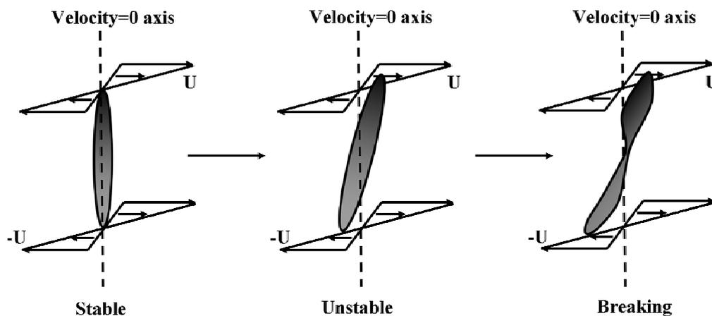
**Figure 4-6** Disturbance causes instability of vorticity-elongated drop.  $U$  is velocity.
