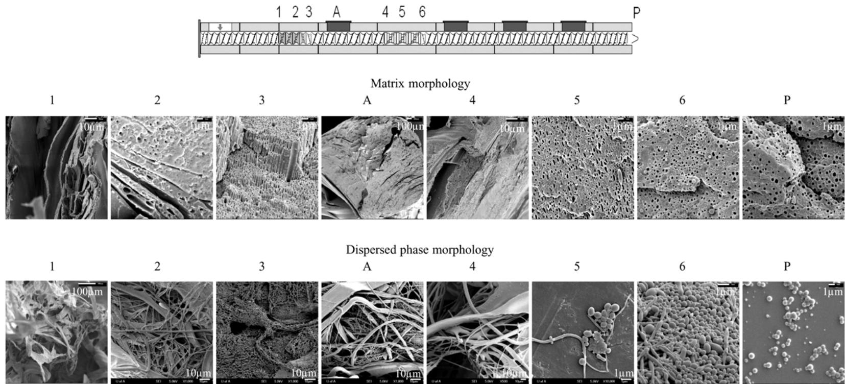
**Figure 2-9** Morphology development of compatibilized system PSMA/aPA (20 wt% aPA ) at 220°C, rotation rate of 1000 rpm and a feed rate of 62.5 kg/hr in Berstorff twin screw extruder. (Note different scale bars).
