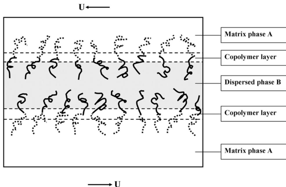
**Figure 2-13** Compatibilization reduces slip at the interface of polymer blends. Chains of block copolymer formed at the interface penetrate into both phases and enhance the effective shear stress on the dispersed phase. The dashed and black curved segments denote polymer chains A and B respectively. Velocity  $U$  applies shear stress to the system.
