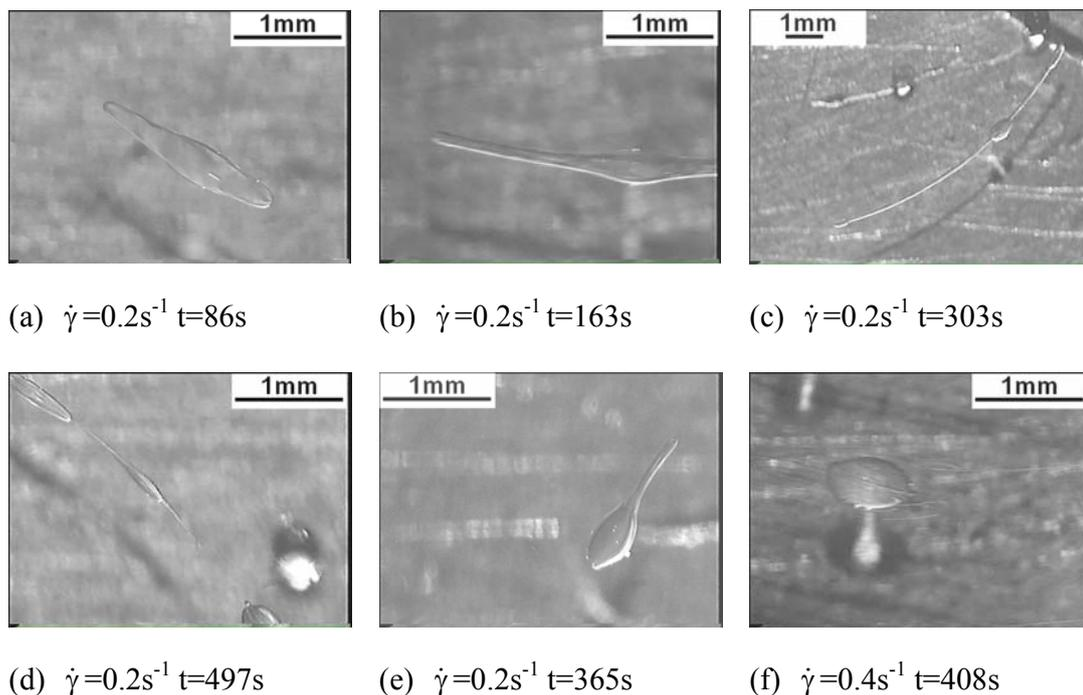
**Figure 5-4** PS sphere sheared in PE matrix at a rotation rate of 1rpm of the master rotor. (a), (b), (c) and (d) show the morphology of the same PS drop after shearing for different time. (e) and (f) show the morphology of another two PS spheres. The shear rates are shown below each micrograph.
