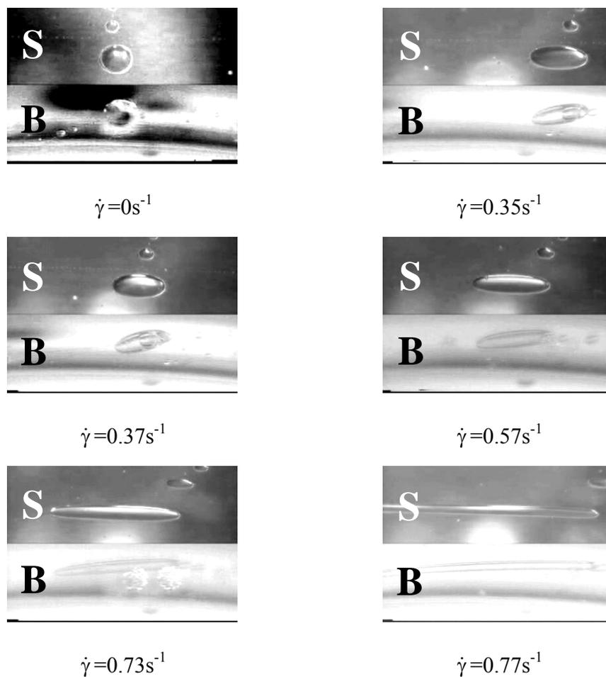
**Figure 3-4** Flow direction deformation of system M3/D3,  $\eta_r=2.6$ ,  $D_0=1.16\text{mm}$ . S and B denote side view and bottom view respectively.
