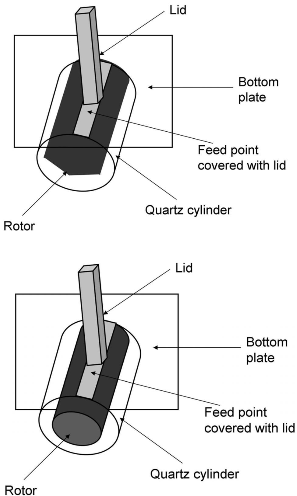
**Figure 6-1** Basic design of cone-plate (top) and Couette device (bottom) for simple shear flow.
