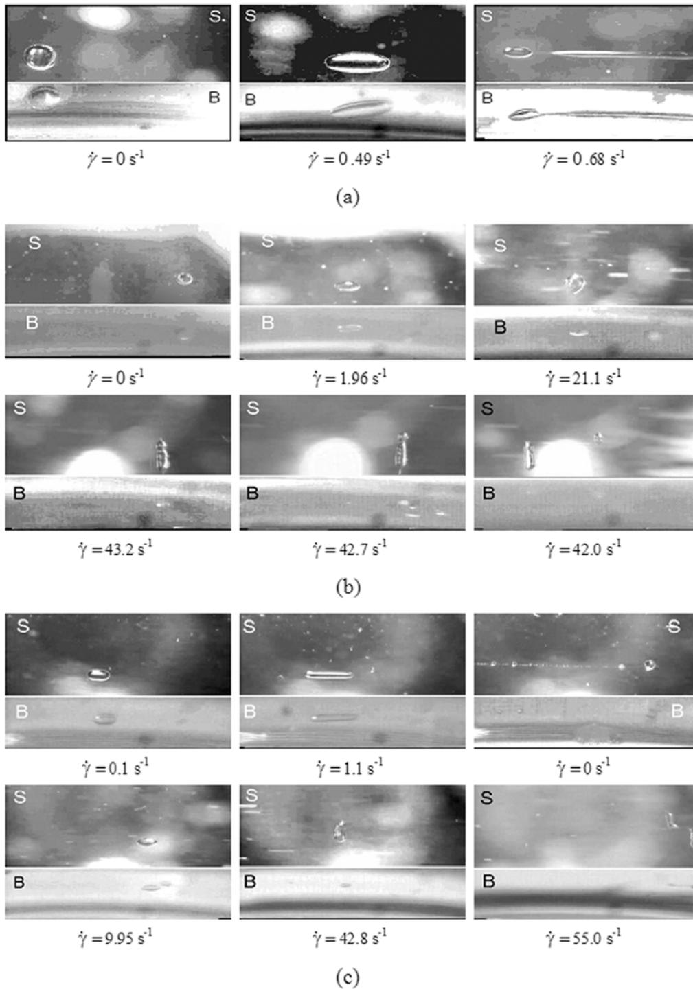
**Figure 4-7** Breakup modes of M3/D3,  $\eta_r=2.6$ , for different drop sizes. (a) Elongation and breakup in the flow direction:  $D_0=1.16$  mm; (b) Elongation and breakup in the vorticity direction:  $D_0=0.57$  mm; (c) Transition from flow direction to vorticity direction,  $D_{20}=0.64$  mm;  $D_{10}=0.46$  mm. S and B denote side view and bottom view respectively.
