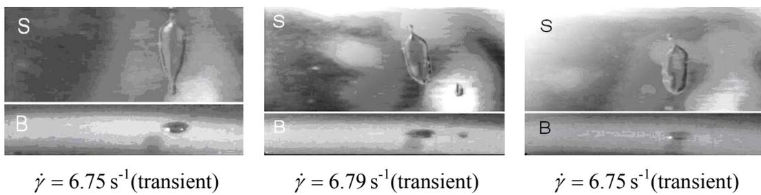
(c) Tip breakup in vorticity direction: M3/D4,  $\eta_r=3.2$ ,  $D_0=1.45\text{mm}$ **Figure 4-5** Drop deformation and breakup modes. For each image, S and B denote the side view and bottom view, respectively.
