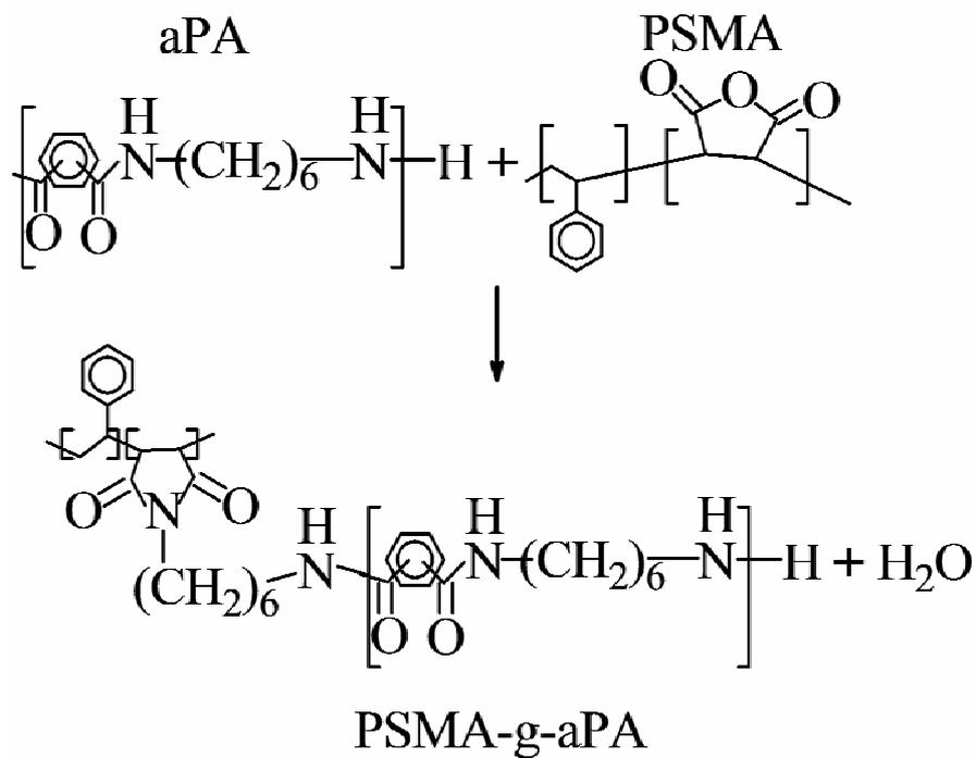
**Figure 2-2** Coupling reaction between aPA and PSMA.
