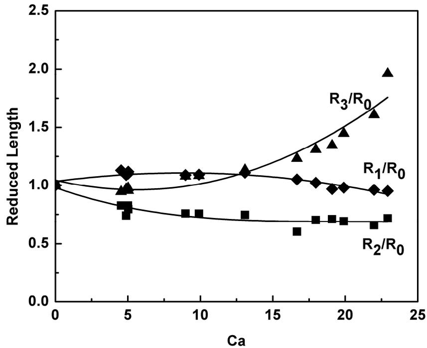
Figure 3-9 Reduced radii of M1/D4,  $\eta_r = 32$ ,  $D_0=1.6\text{mm}$ .
