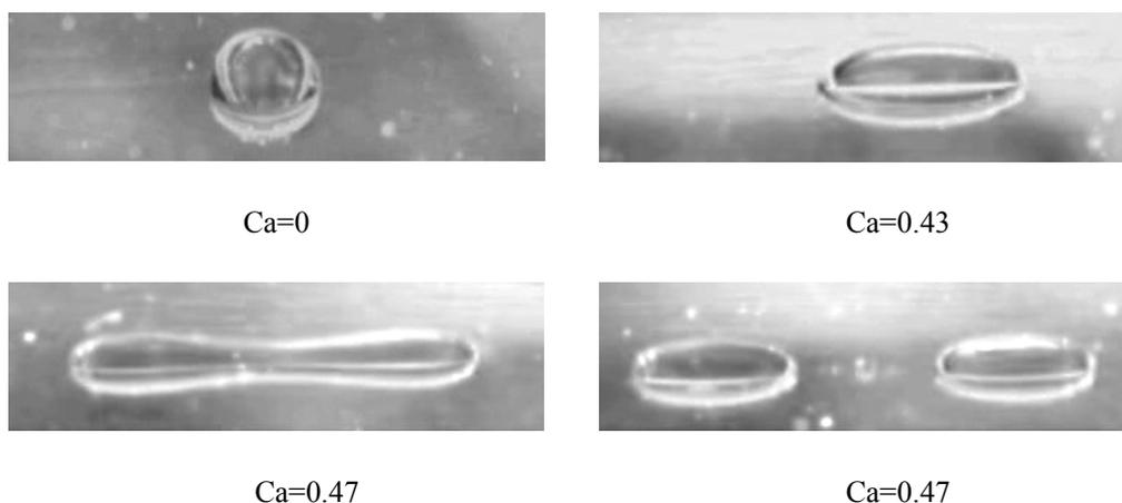
**Figure 1-3** Deformation and breakup process of a corn syrup drop in polydimethylsiloxane (PDMS) under shear flow in a Couette device,  $\eta_r=0.55$ . The original drop diameter is 1.2mm.
