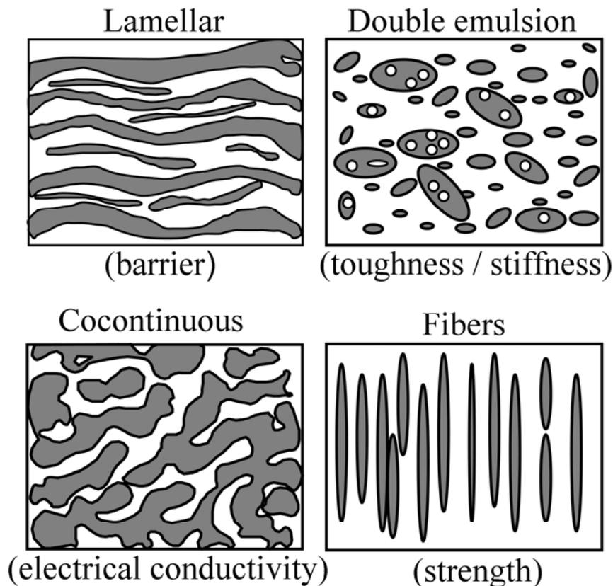
**Figure 1-1** Polymer blend morphologies and their characteristic properties. Adapted from [3, 9].
