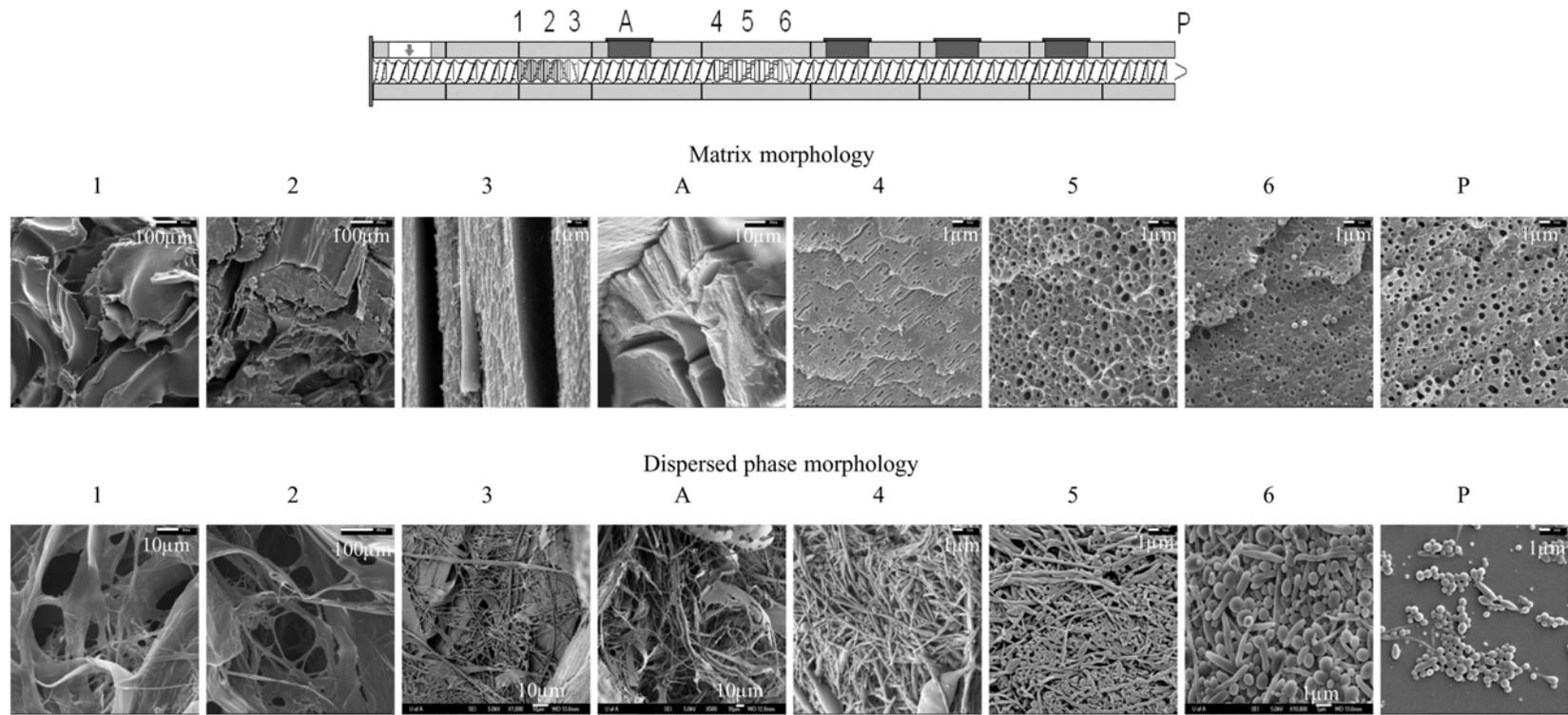
**Figure 2-7** Morphology development of compatibilized system PSMA/aPA (20 wt% aPA ) at 220°C, rotation rate of 400 rpm and a feed rate of 25 kg/hr in Berstorff twin screw extruder. (Note different scale bars).
