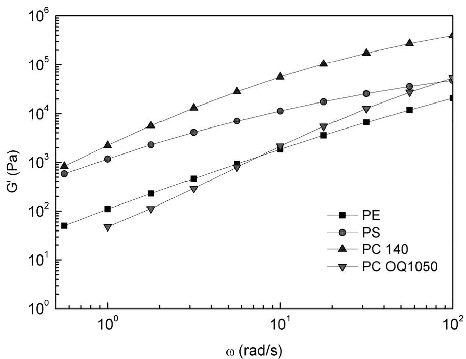
**Figure 5-2** Elastic modulus ( $G'$ ) versus frequency ( $\omega$ ) for polymers at 220°C.
