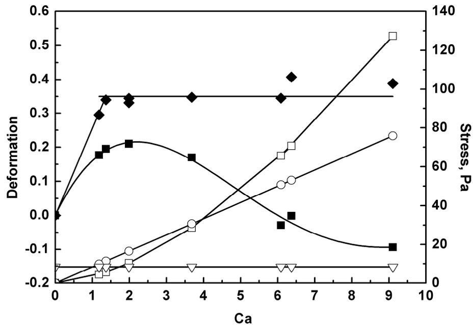
**Figure 3-12** Development of stresses and deformations with increasing capillary number,  $M3/D5$ ,  $\eta_r = 4.1$ ,  $D_0 = 0.72$  mm. Solid symbols are deformations:  $Df_1$  (■),  $Df_2$  (◆); and unfilled symbols are stresses:  $\Gamma/R_0$  (▽),  $\tau$  (○),  $N_1$  (□).
