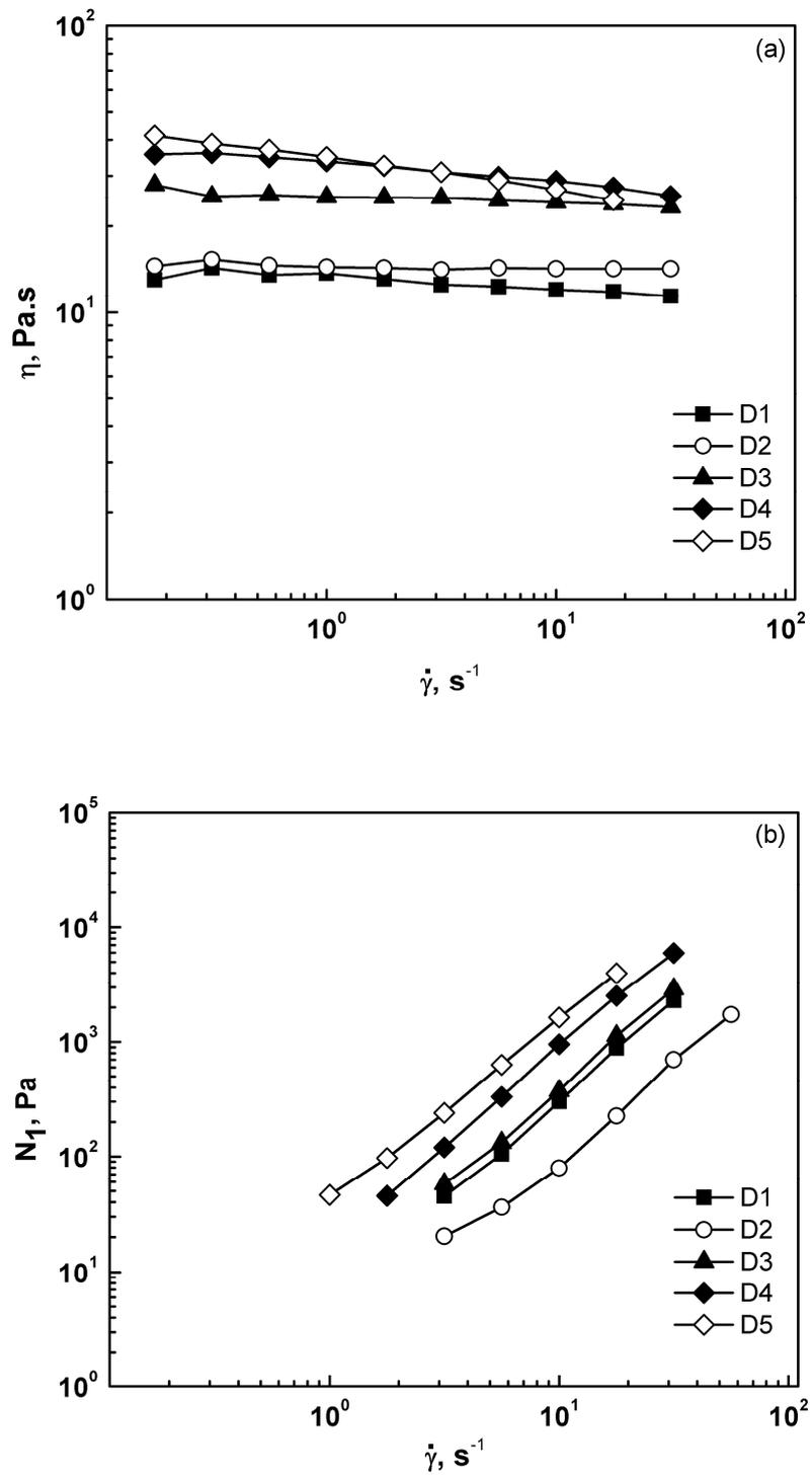
**Figure 3-1** Rheological properties of Boger fluids. (a) Viscosity of Boger fluids. (b) First normal stress difference of Boger fluid.
