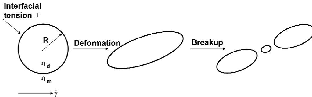
**Figure 1-4** Schematic of drop deformation in a shear flow.
