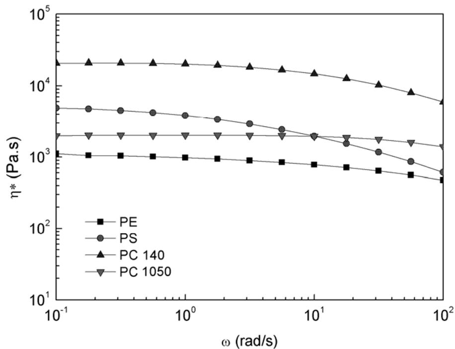
**Figure 5-1** Complex viscosity ( $\eta^*$ ) versus frequency ( $\omega$ ) for polymers at 220°C.
