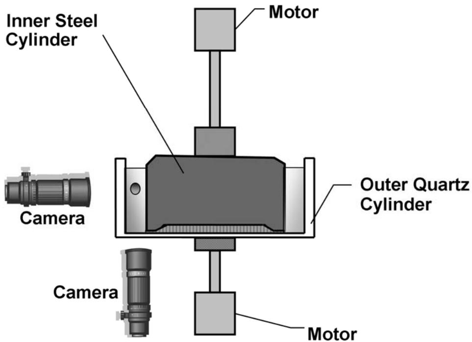
**Figure 4-4** Couette apparatus diagram.
