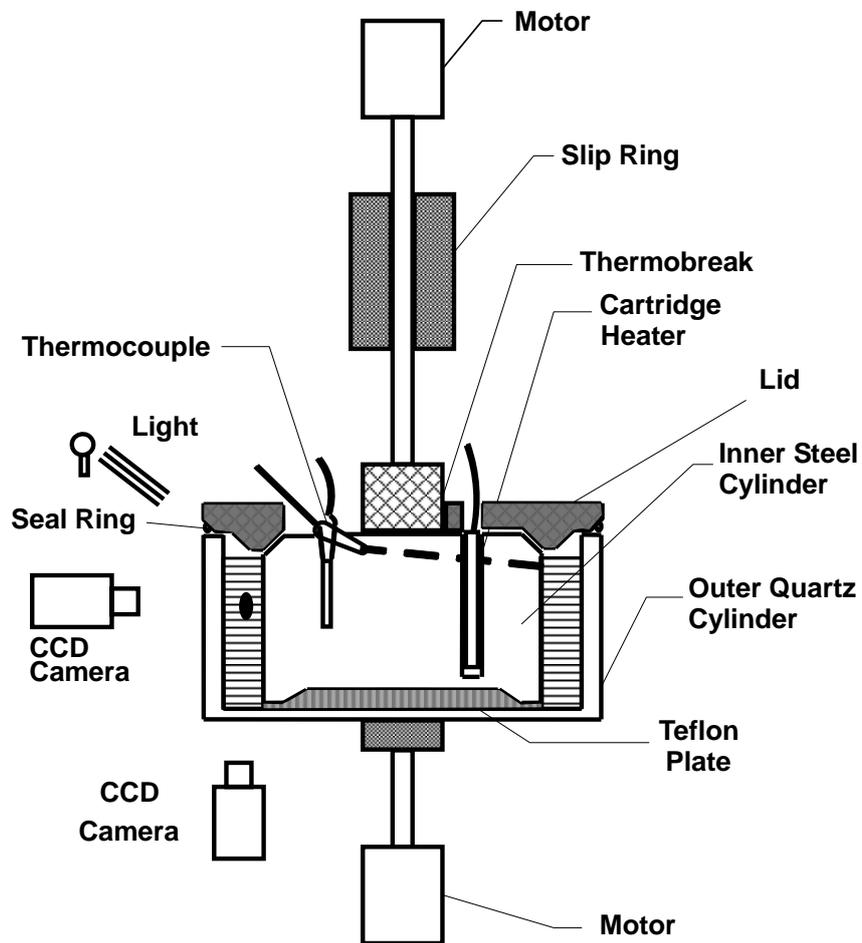
**Figure 3-2** A schematic of the Couette apparatus.
