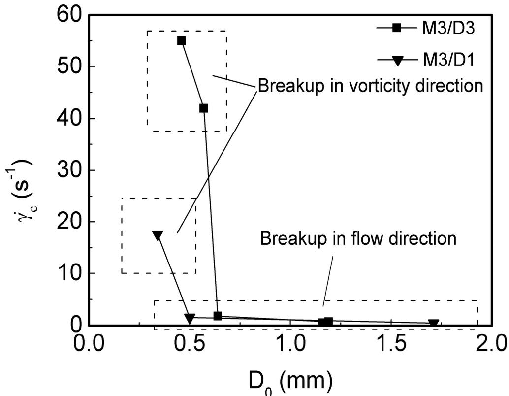
**Figure 4-8** The critical shear rate jumps when the breakup mechanism changes.
