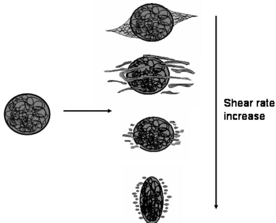
**Figure 5-10** Surface instability of polymer drop during shearing.
