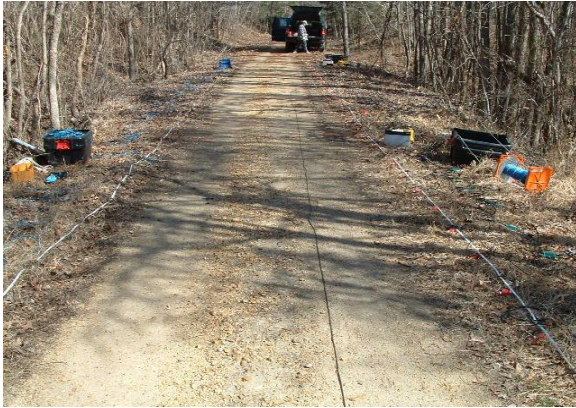
Figure A-11 this is the surface layout of tunnel 5, on the left is the ERT survey, the right is the seismic
