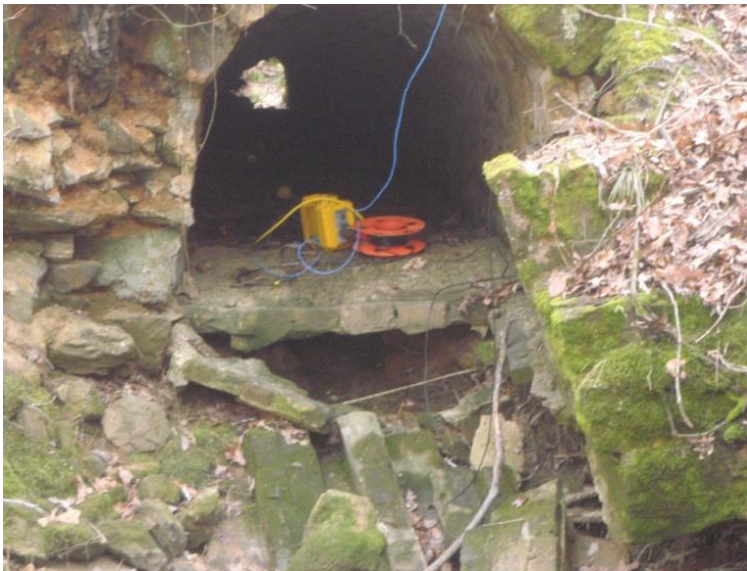
Figure A-2 Picture of the south side of the tunnel entrance. Te yellow box is the geode and orange reel is the trigger line for the accelerated weight drop
