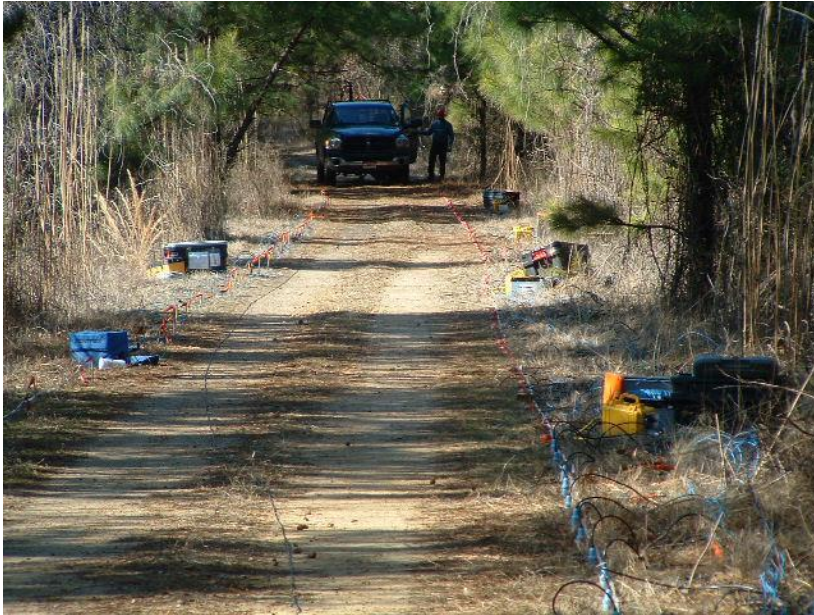
Figure A-19: This is the surface layout for tunnel 8. The right has the geophones attached, the blue geophones are the 10Hz geophones, and the 10Hz geophones are red. The left hand side of the surface has the ERT survey
