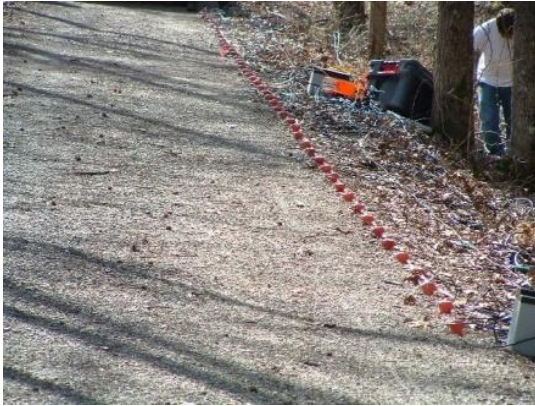
Figure A-16 This is the surface layout of Tunnel 7, the geophones are on the side of the path.
