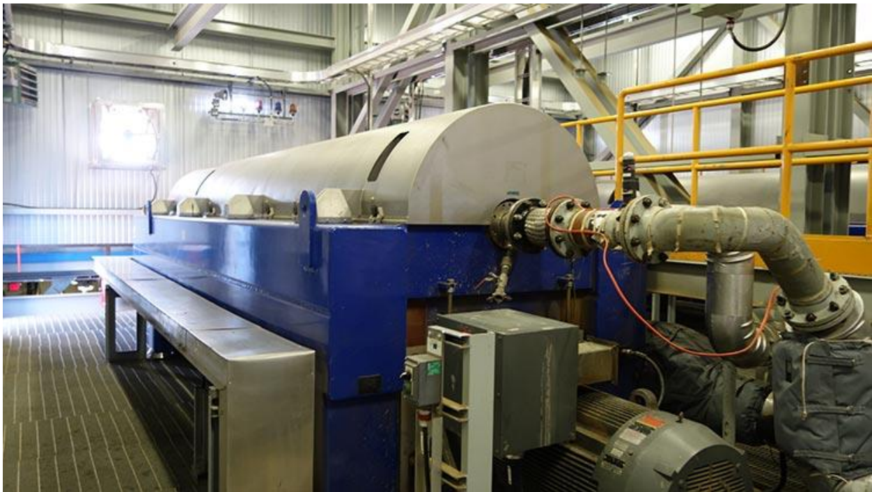
Figure 2-13: Centrifuge used at Albian's Jackpine Mine (Canada's Oil Sands Innovation Alliance 2021)
