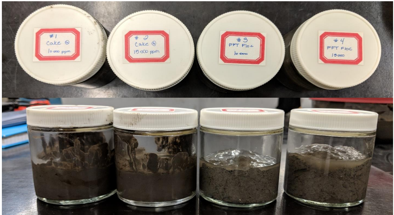
Figure 3-9: Qualitative - bacteria treated samples after 30 days of incubation at room temperature
