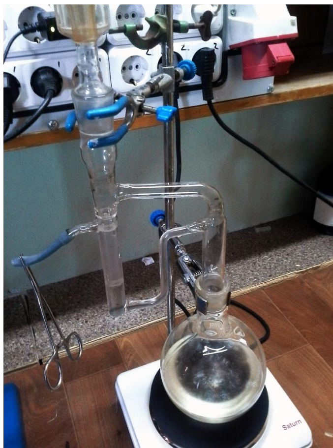
Figure A-1: Dean Stark extraction setup
